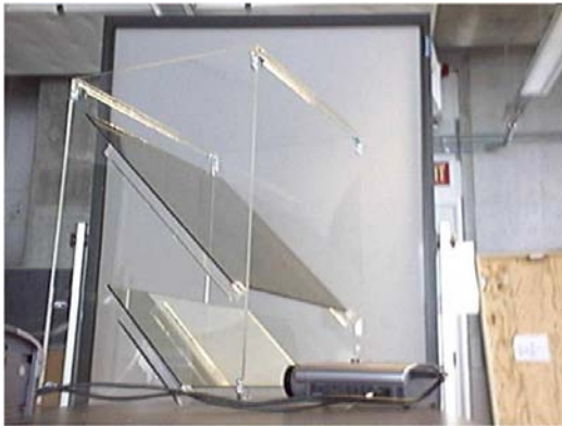
(c) The video tunnel with projector, mirror, and half silvered mirror. The entire apparatus was held together with clear acrylic.
