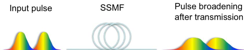
Figure 4.1 Input pulse with positive chirp will be broadened monotonically as it propagates along 1550-nm standard single-mode fiber (SSMF), because high frequency (blue) components travel faster than low frequency (red) components. Transmission distance is severely limited by pulse broadening.
