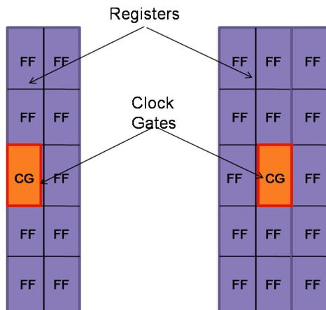
Figure 5.4. Structured placement of clock gates and the latches in their fanout cone. By constraining the placement of the clock gates and the latches in datapath blocks, the local clock networks exhibit low skew and power.
