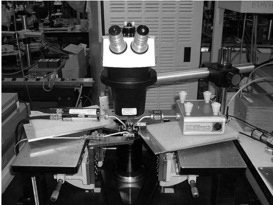
Figure 4.15 On-wafer noise figure measurement setup.
