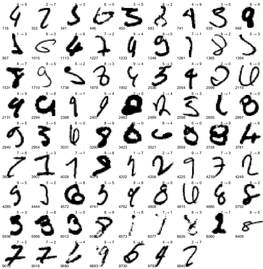
Figure 2: All the 79 misclassifications using pyramid HOG features with the intersection kernel SVM, on the MNIST dataset. X \rightarrow Y on the top right corner of each example denotes that X is misclassified as Y . The number in the bottom left corner is the index of the example in the test set.
