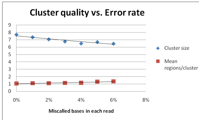
Figure 4: Clustering Accuracy. Our algorithm is able to maintain the cluster size relatively well even as the error rate increases to the maximum seen in practice. Also, the mean number of regions per cluster increases by a negligible amount, which means that cluster integrity is not compromised.
