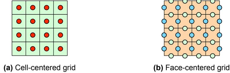
Figure 2.7: This diagram shows that the cell-centered grid in (a) requires far fewer grid points than the face-centered grid in (b). The grid points in (b) are color-coded, where the points along a cell’s horizontal edges are green and the points along the vertical edges are in blue.
