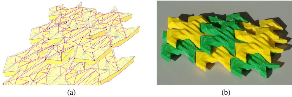
Figure 20: A  $2\frac{1}{2}$ D offset tiling: (a) displaying the laterally offset layer that lies below the tile; and (b) manufactured tiles.
