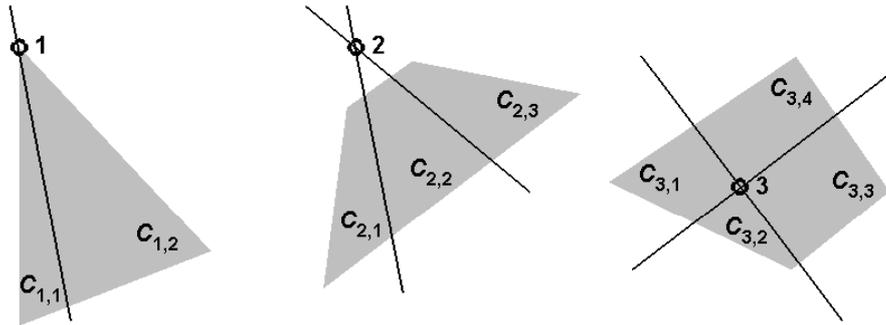
Figure 3.3: Three examples of camera domains  $\mathcal{D}_\alpha$ . Cameras can be inside or outside their domains. Our camera model spans projection models from perspective cameras to omni-directional cameras. Decompositions are shown for each set.
