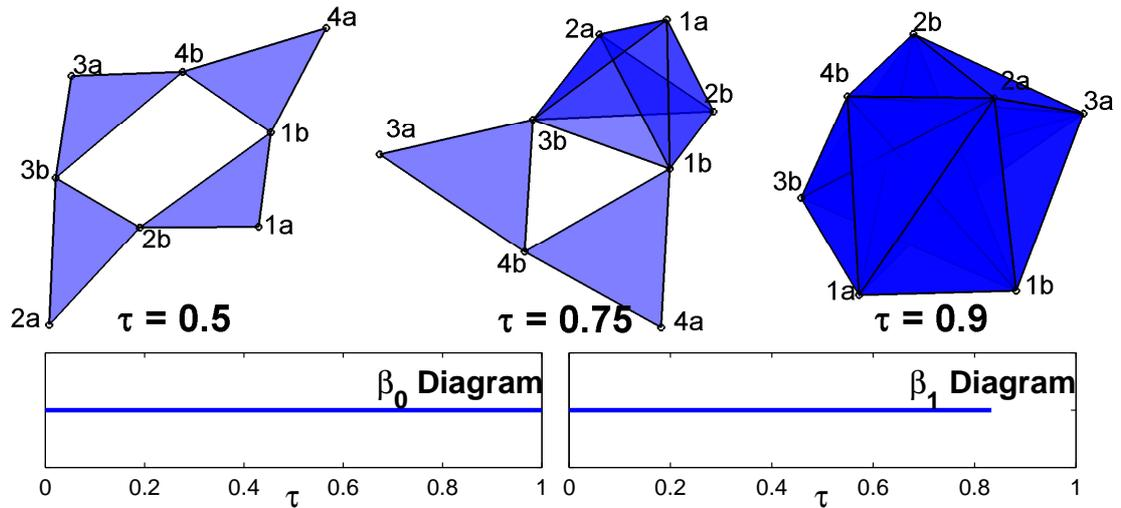
Figure 4.5: *CN*-Complexes for several values of  $\tau$  (top) and persistence diagrams (bottom) are shown for the circular corridor setup in figure 4.4. We observe that the diagram shows a persistent single connected component and a persistent loop.
