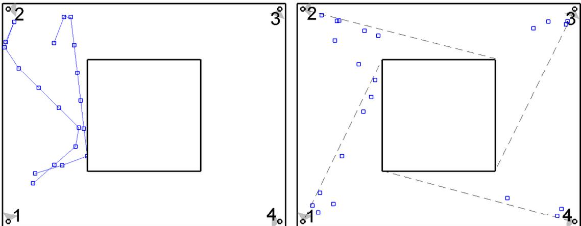
Figure 4.4: Layout of a circular corridor setup with two targets moving through the environment (left). Intersect points found, plotted as squares, for a threshold value  $\tau = 0.5$  with corresponding bisecting lines, plotted as dashed lines (right).
