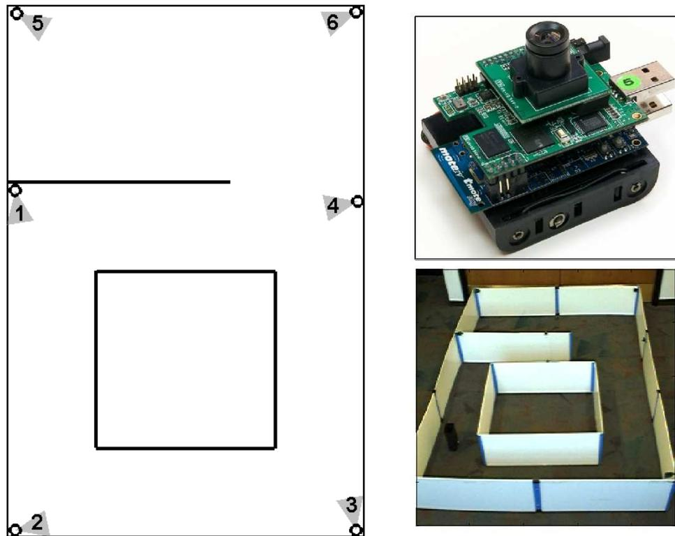
Figure 3.6: Layout used for our experiment. A diagram showing the location of the different cameras (left). A picture of our experimental maze (bottom-right). The CITRIC camera nodes used for our experiments (top-right).
