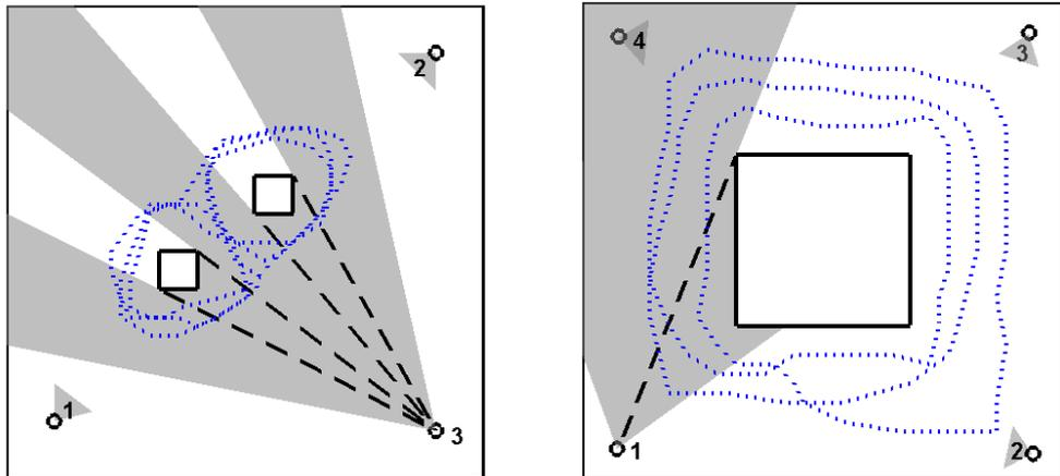
Figure 3.5: A layout with two objects where  $C_3$  is shown (left). A circular hallway configuration where  $C_1$  is shown (right). Dashed lines represent corresponding bisecting lines. Dotted curves represent the paths followed by the target during the simulation.
