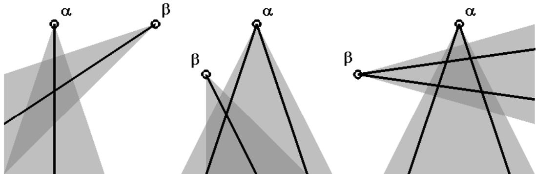
Figure 6.1: Sample configuration for one line of sight for each camera (left). Note that if we assume that these lines intersect and fix the line of sight of camera  $\alpha$ , camera  $\beta$  can be virtually anywhere. Sample configuration for two lines of sight for camera  $\alpha$  and one for camera  $\beta$  (middle). Sample configuration for two lines of sight for both cameras (right).
