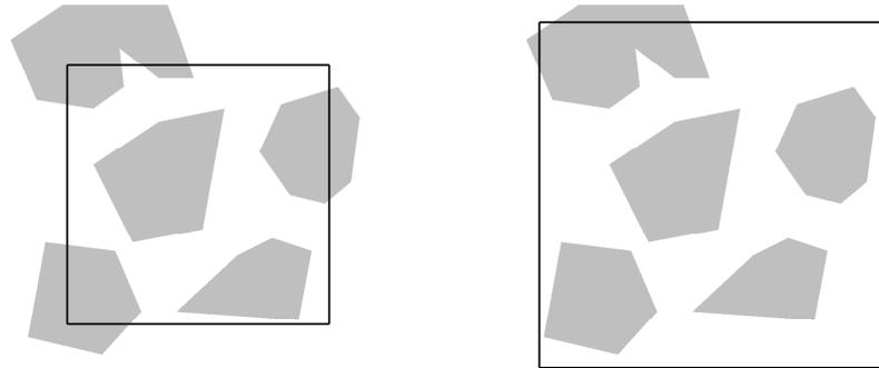
Figure 7.3: Illustration of how to count connected components for neighborhood  $K_r$  (left) and  $K_{r+C}$  (right). There are 5 connected components in  $K_{r+C}$ . There are 6 connected components in  $K_r$  and 3 connected components after boundary identification. Without boundary identification we could erroneously conclude that a set disappeared.
