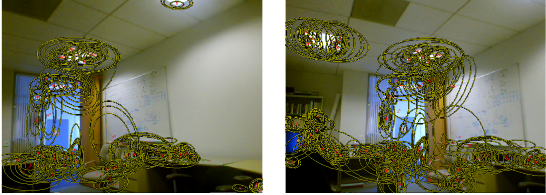
Figure 4.3. Examples of regions found by Hessian-Affine region detector. The detected interest points are plotted as red crosses, while the estimated affine region are shown as yellow ellipses.
