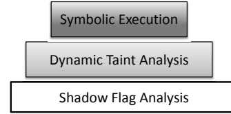
Figure 2: A Layered Approach for Annotative Execution
