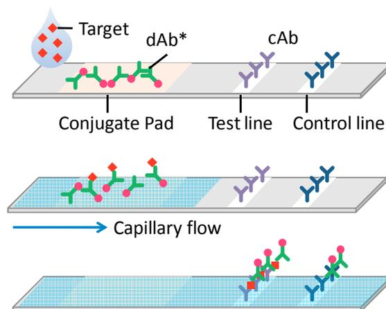
Figure 2-2. Operating principle of a lateral flow test.
