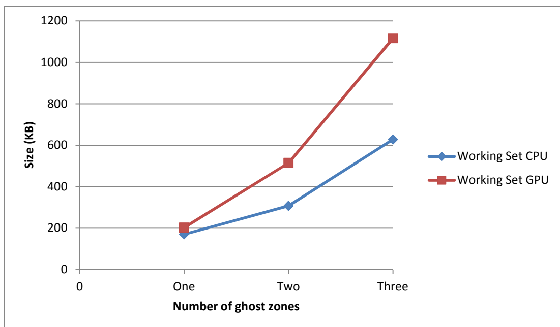
Fig 9 : Working set of memory on CPU and GPU
