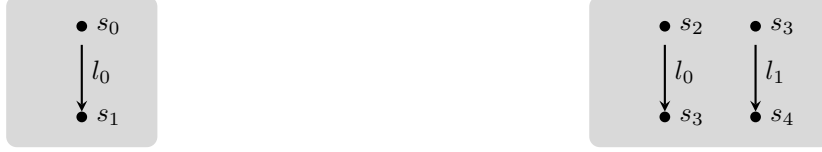
Figure 2. s_0 and s_2 are not bisimilar, even though the only execution starting from s_0 is in perfect agreement with the only execution starting from s_2 .
