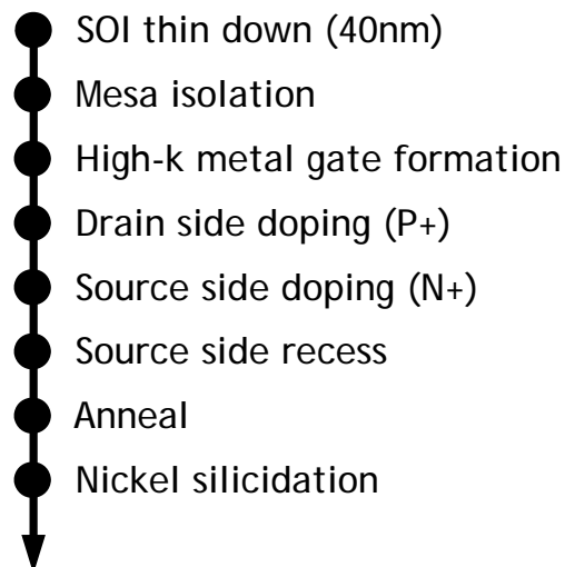
Figure 4.2 Fabrication process flow of silicided source TFET
