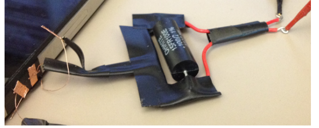
Figure 9: Close-up of the wiring rig that connects our iPhone 4S test phone with the Monsoon Power Monitor.
