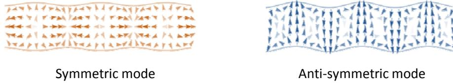
Figure 2.2 Symmetric and anti-symmetric Lamb wave modes.
