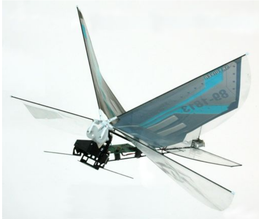
Figure 3.3: BOLT: a bipedal ornithopter capable of both aerial and terrestrial locomotion.
