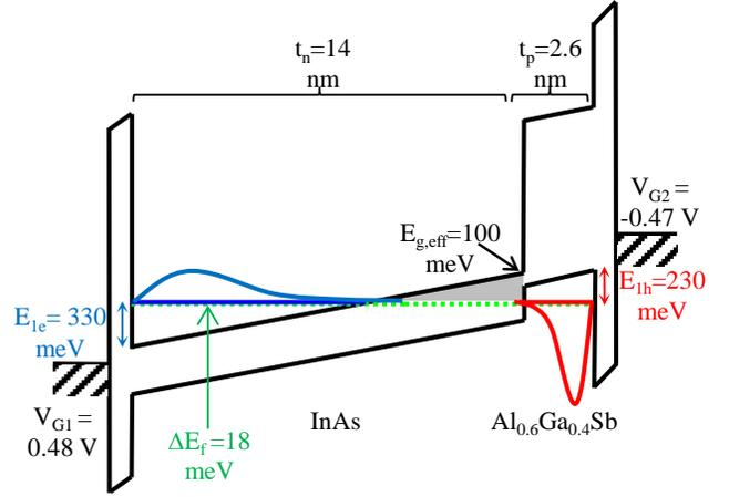
Fig. 5: The band diagram for the optimal heterojunction structure with an on state conductance of 1 mS/ $\mu$ m and maximum bias or Work Function difference < 1eV is shown. The narrow p-well eigenstate energy changes little as the bias changes, helping the gate efficiency.
