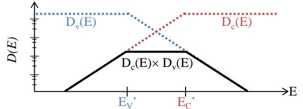
Fig. 3: The conduction and valence band density of states,  $D_C(E)$  and  $D_V(E)$ , are shown. Below the band edges the density of states falls off exponentially. The product,  $D_C(E) \times D_V(E)$  is also shown.
