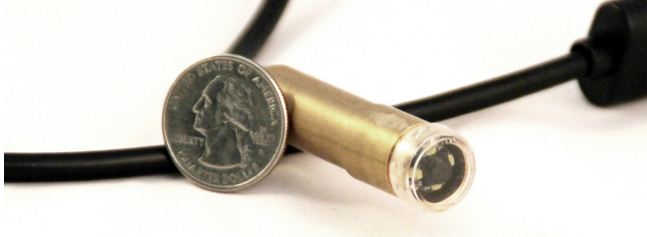
Figure 4. The hardware can be miniaturized, as in this pipe inspection camera with integrated lights.
