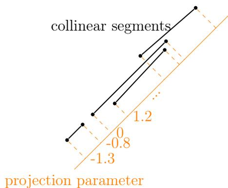
Fig. 4.6. Projection to 1D parametric space.
