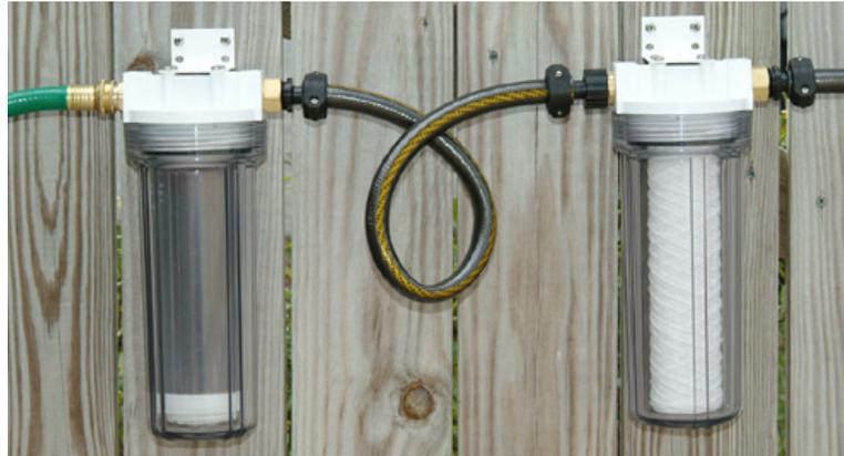
Figure 3.4: Two inline water filters in domestic use. Photo credit: [thedriversseat.com](http://thedriversseat.com).
