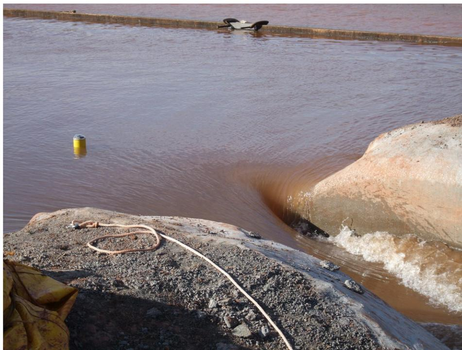
Figure 1.9: FSN drifter about to pass through the levee breach at the HERU facility.
