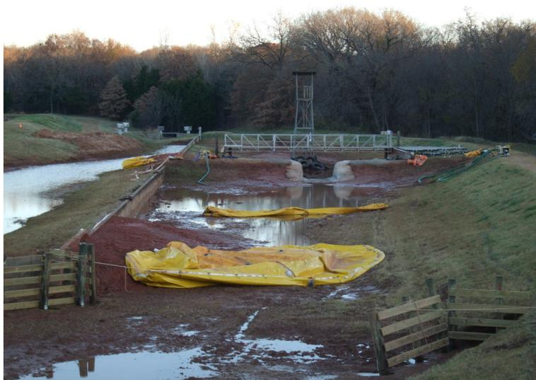
Figure 1.8: HERU facility: Hydraulic test area, empty, with test levee in background. This facility was used to test the Floating Sensor Network drifters' survivability in levee breach conditions.
