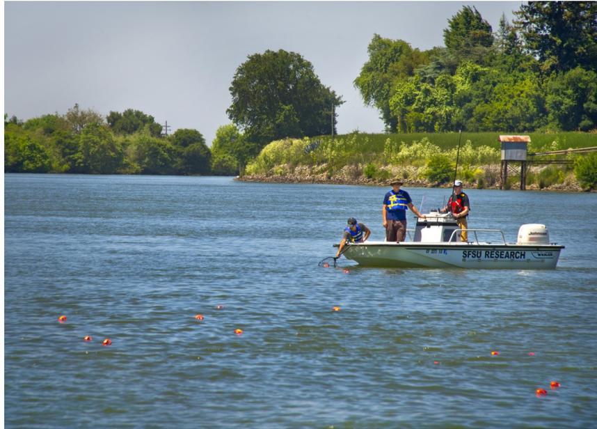
Figure 3.3: Retrieving Android drifters with small nets. Photo credit: Berkeley Lab — Roy Kaltschmidt.
