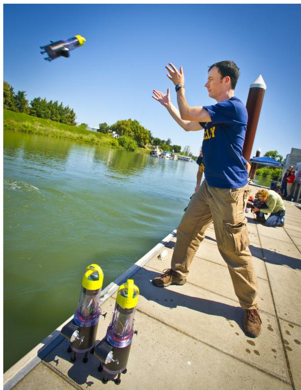
Figure 8.7: Throwing a Gen 3 drifter from the dock into the Sacramento River. Photo credit: Roy Kaltschmidt.
