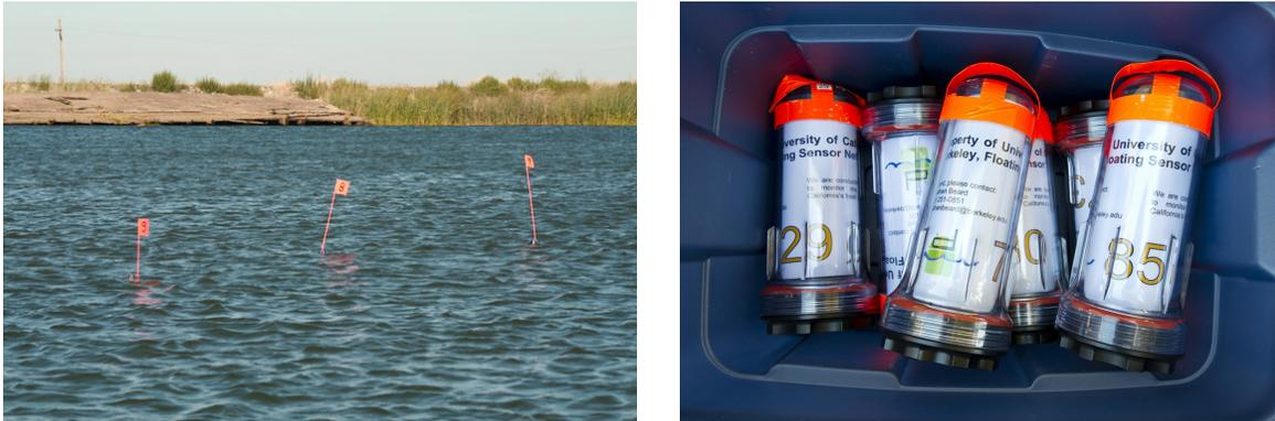
Figure 3.9: Left: three flagged drifters under wind influence. Right: Android drifters in tub, showing duct tape handle. Photo credits: Jean-Benoît Saint-Pierre, Jonathan Beard.
