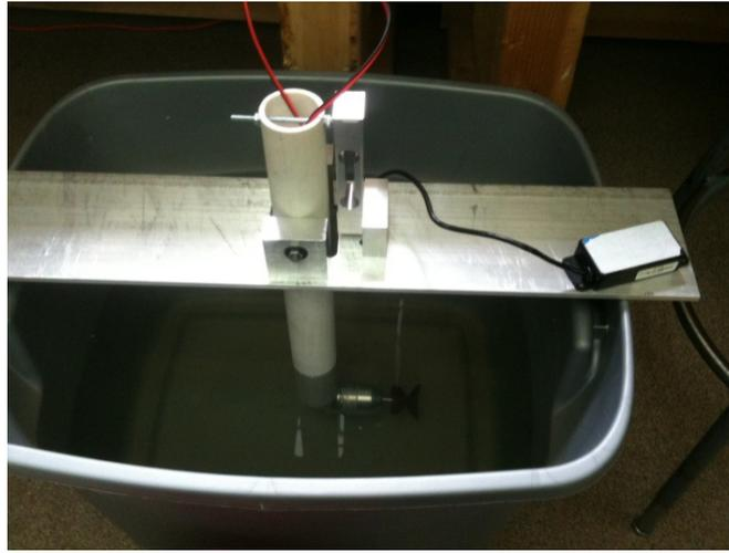
Figure 3.11: Motor force test platform: submerged motor unit is attached to an extended arm which pivots against a force transducer.
