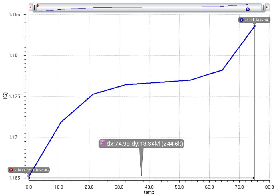
Figure 4.6: Simulation of the LO frequency across temperature
