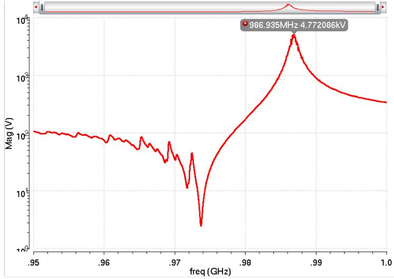
Figure 2.19: Measured impedance of a 987MHz FBAR resonator
