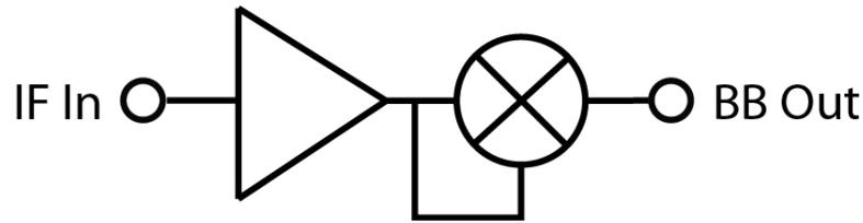
Figure 4.12: Self-mixing energy detector block diagram
