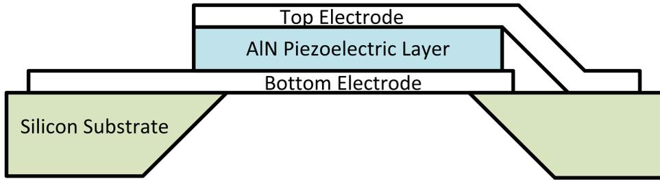
Figure 2.17: Diagram of the structure of an FBAR resonator
