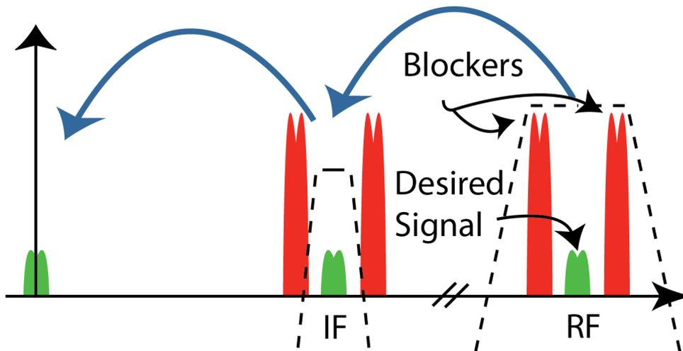
Figure 2.4: Frequency plan for a super-heterodyne receiver.
