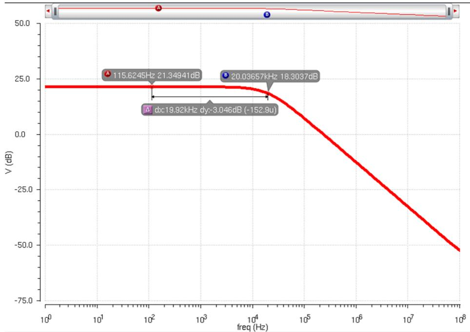
Figure 4.16: AC performance of the low-pass filter and integrator.
