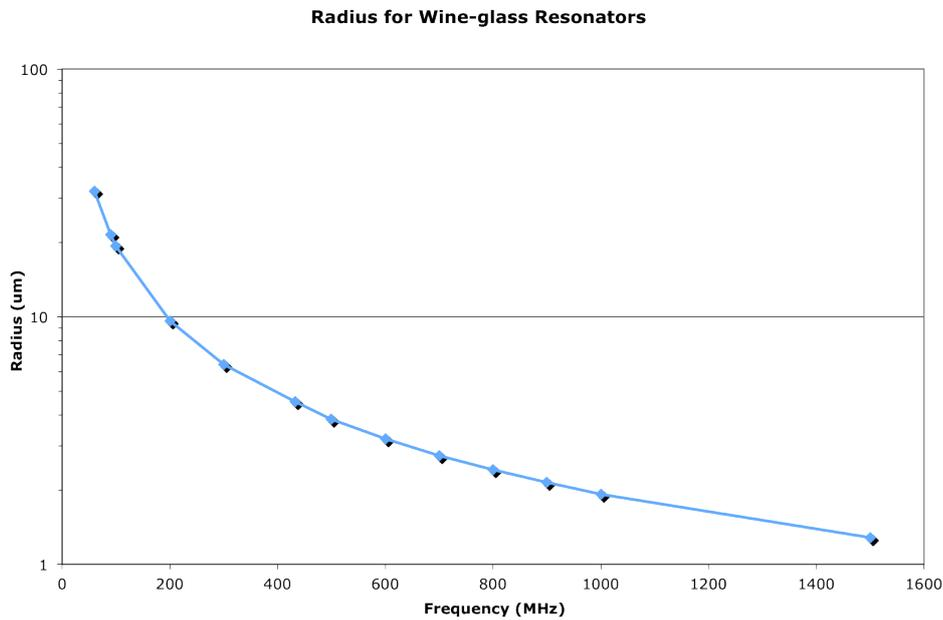
Figure 2.15: Radius required for a given resonant frequency with a wineglass disc resonator
