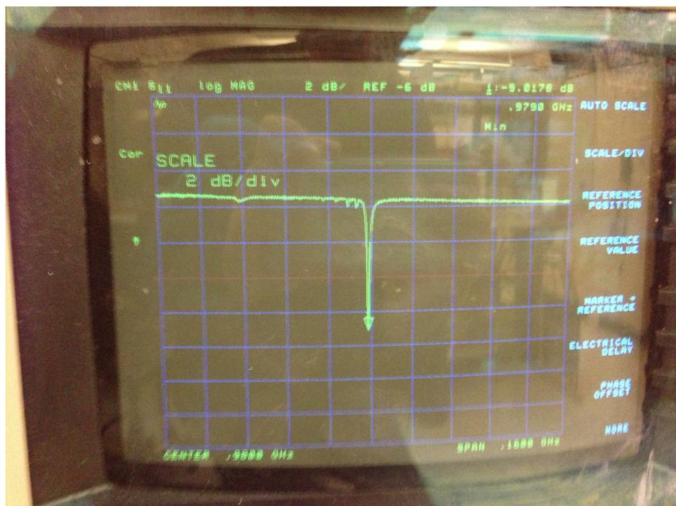
Figure 4.22: Measured S11 of Receiver
