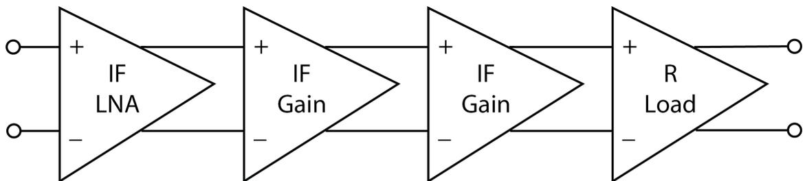
Figure 3.16: IF amplifier lineup diagram
