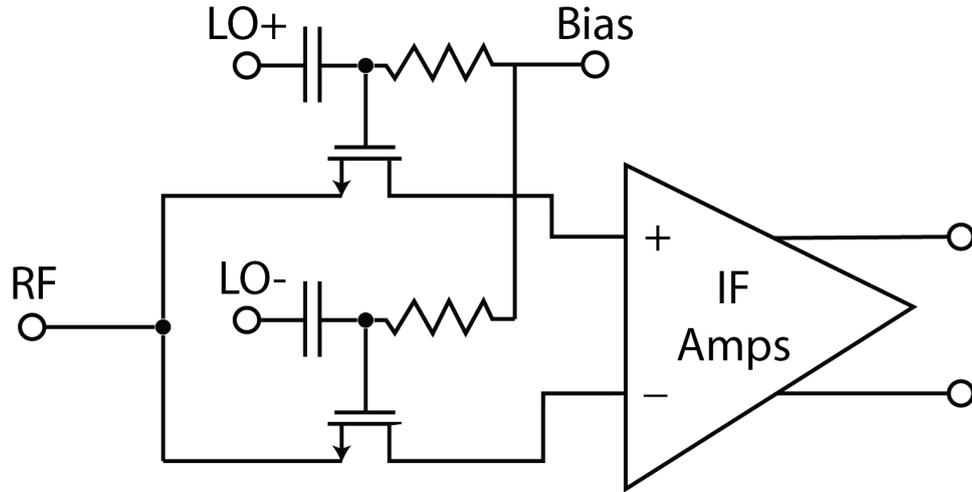
Figure 4.2: Mixer schematic
