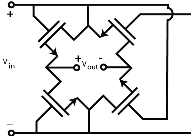
Figure 4.13: Energy detector schematic. Note that biasing details are not shown for simplicity, but all transistors are biased to be roughly at their threshold to maximize output.
