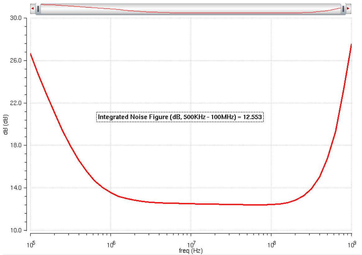
Figure 4.11: Baseband noise figure, assuming a wideband impedance match instead of a narrowband resonator match
