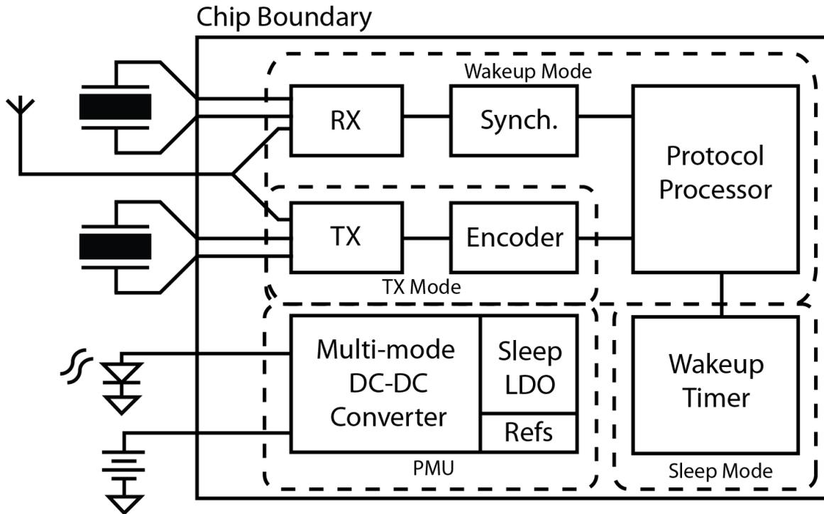
Figure 3.1: Block diagram of the Active RFID system
