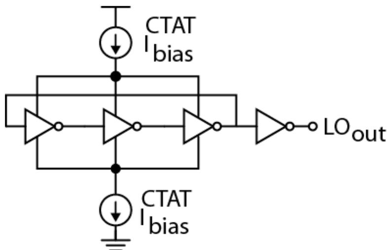
Figure 4.4: Temperature compensated ring oscillator LO
