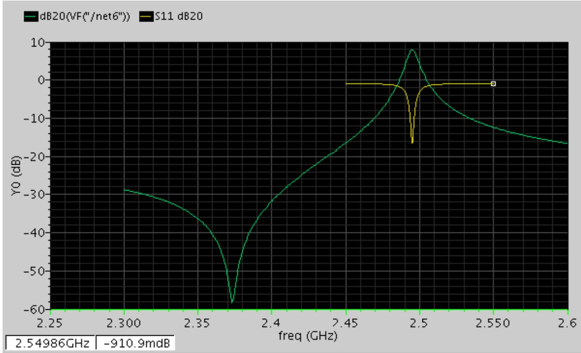
Figure 3.8: Simulated S11 and AC performance
