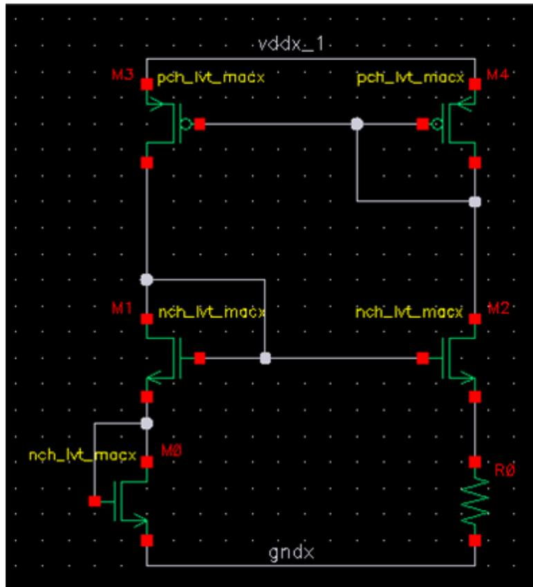
Figure 4.5: CTAT current reference used to bias the ring oscillator
