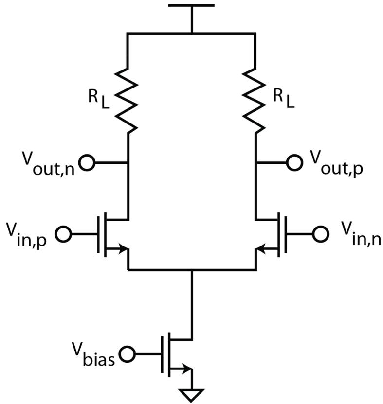
Figure 3.15: Final IF amplifier to interface with the energy detector
