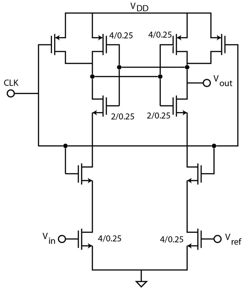
Figure 3.20: Comparator schematic
