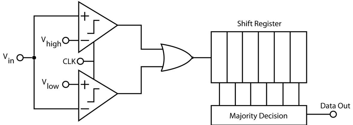
Figure 3.18: Digital Energy Detection
