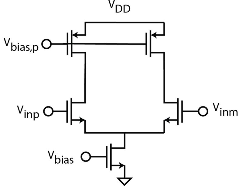
Figure 2.9: Typical analog gain stage.
