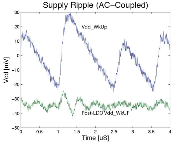
Figure 3.25: Voltage supply ripple due to integrated DC-DC converter
