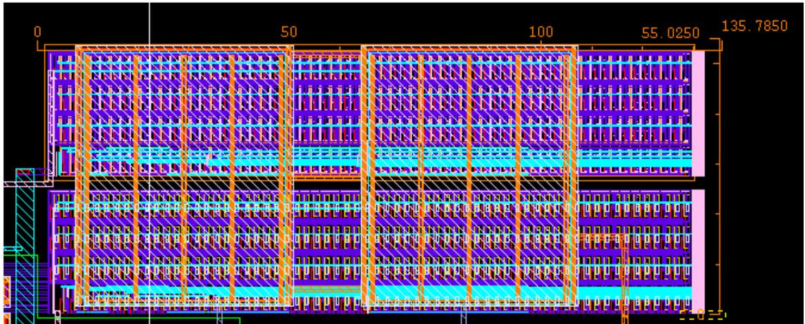
Figure 3.11: Resistor DACs used to tune the ring oscillator LO
