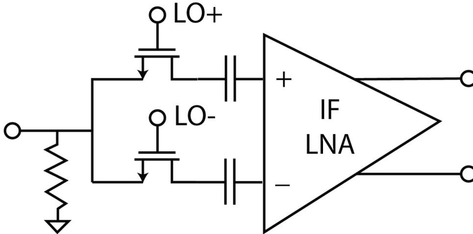
Figure 3.9: Passive mixer schematic
