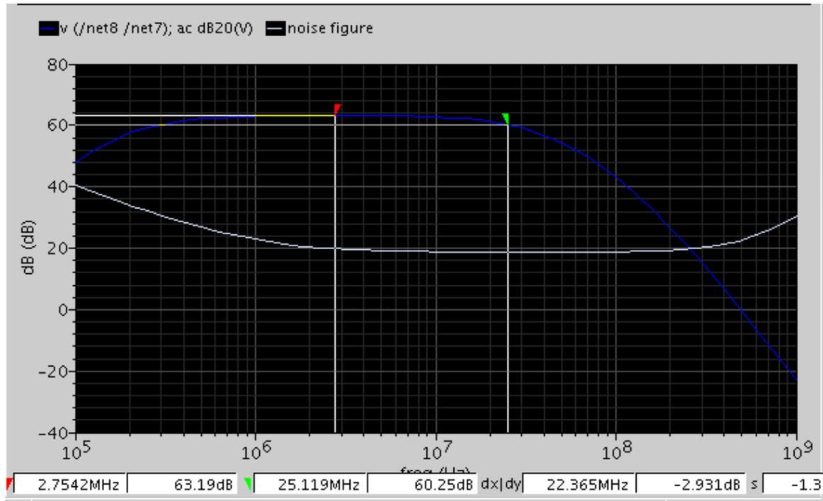
Figure 3.17: Simulated gain and noise figure for the IF amplifier chain
