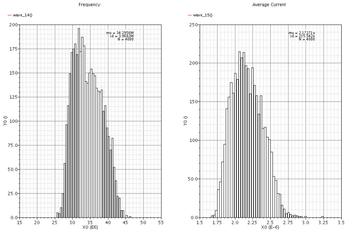
Figure 3.22: Monte Carlo simulation of the sampling clock
