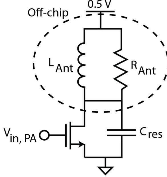
Figure 3.6: Power amplifier schematic, illustrating antenna impedance
