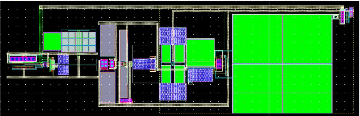
Figure 4.21: Layout view of the core always-on wake-up receiver
