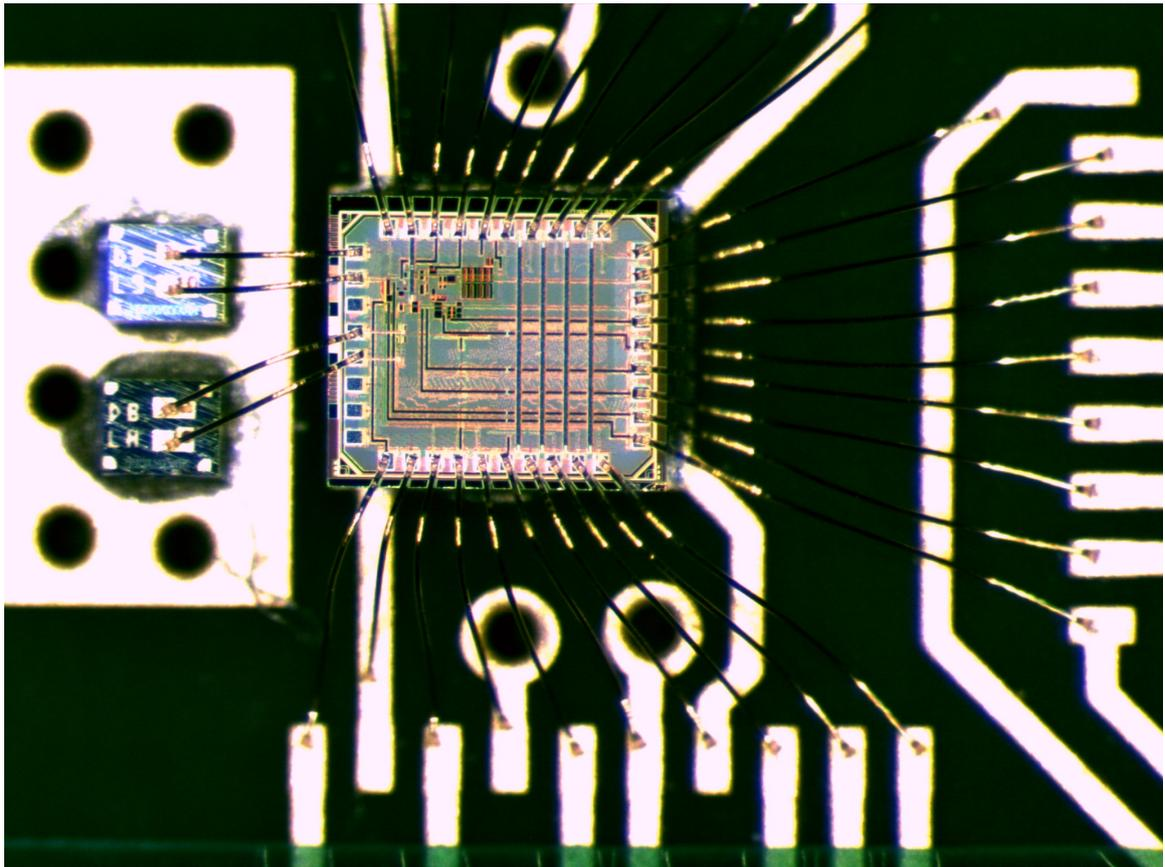
Figure 4.19: Die Photograph of Bonded Chip and FBARs
