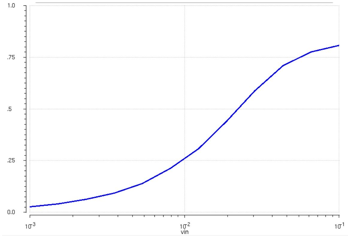
Figure 4.14: Energy detector gain. The X-axis shows the input signal level in volts, and the Y-axis shows the gain in V/V.
