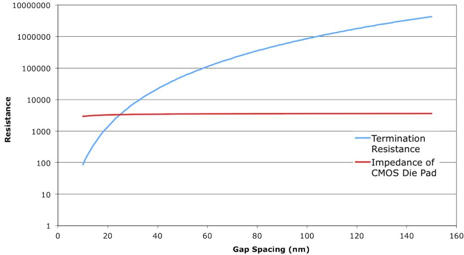
Figure 2.16: Termination impedance required for a filter with electrostatic MEMS resonators
