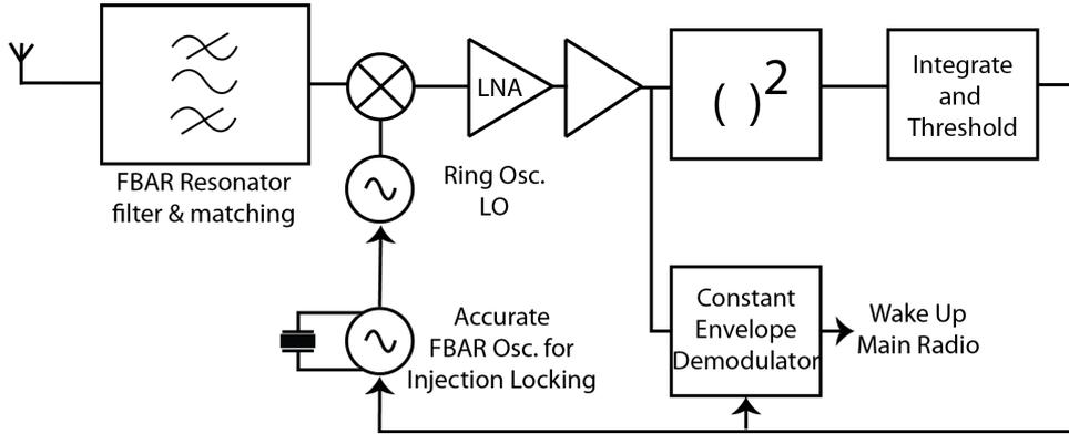
Figure 4.1: Block diagram of a complete wakeup receiver system
