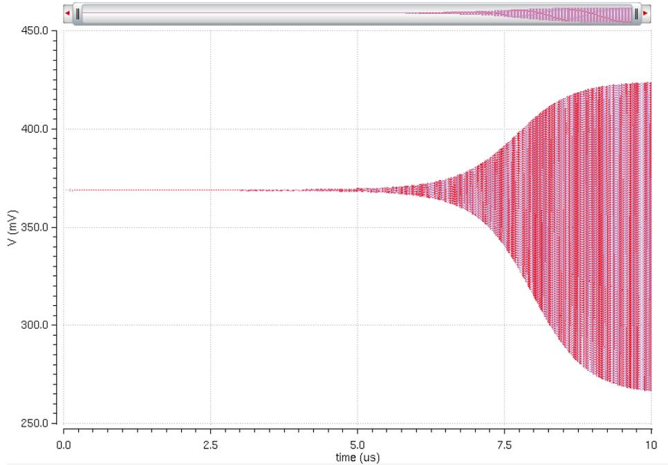
Figure 4.18: FBAR oscillator startup transient
