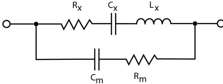
Figure 2.18: Electrical model of the FBAR resonator
