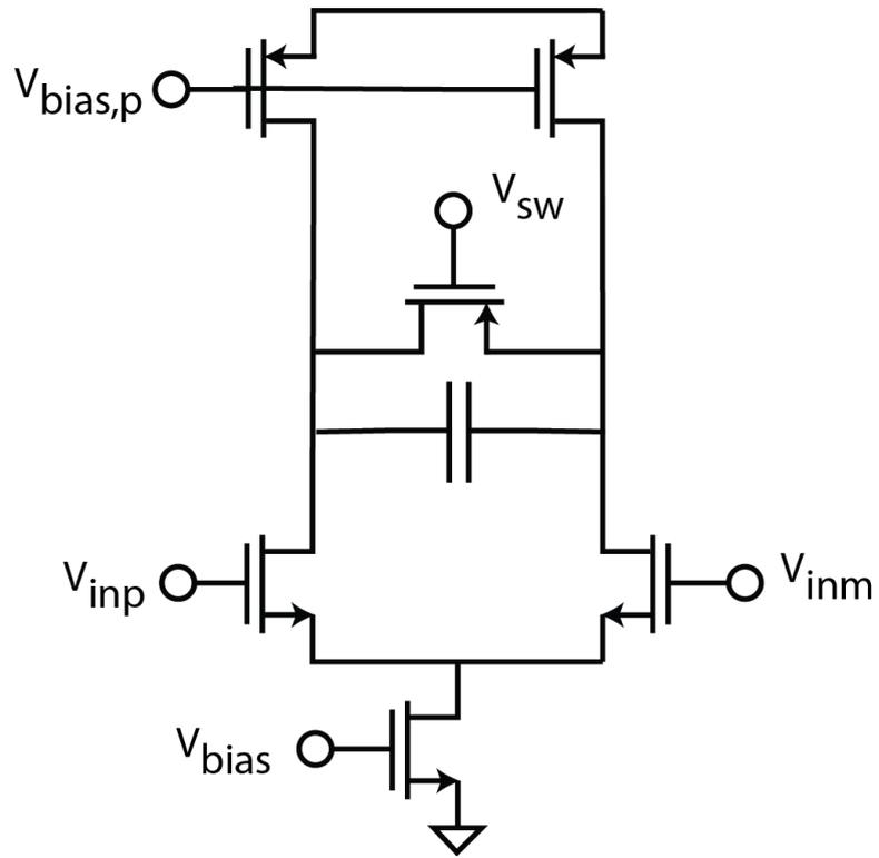
Figure 4.15: Integrator schematic
