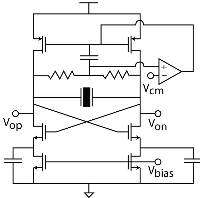
Figure 4.17: FBAR oscillator for injection locking
