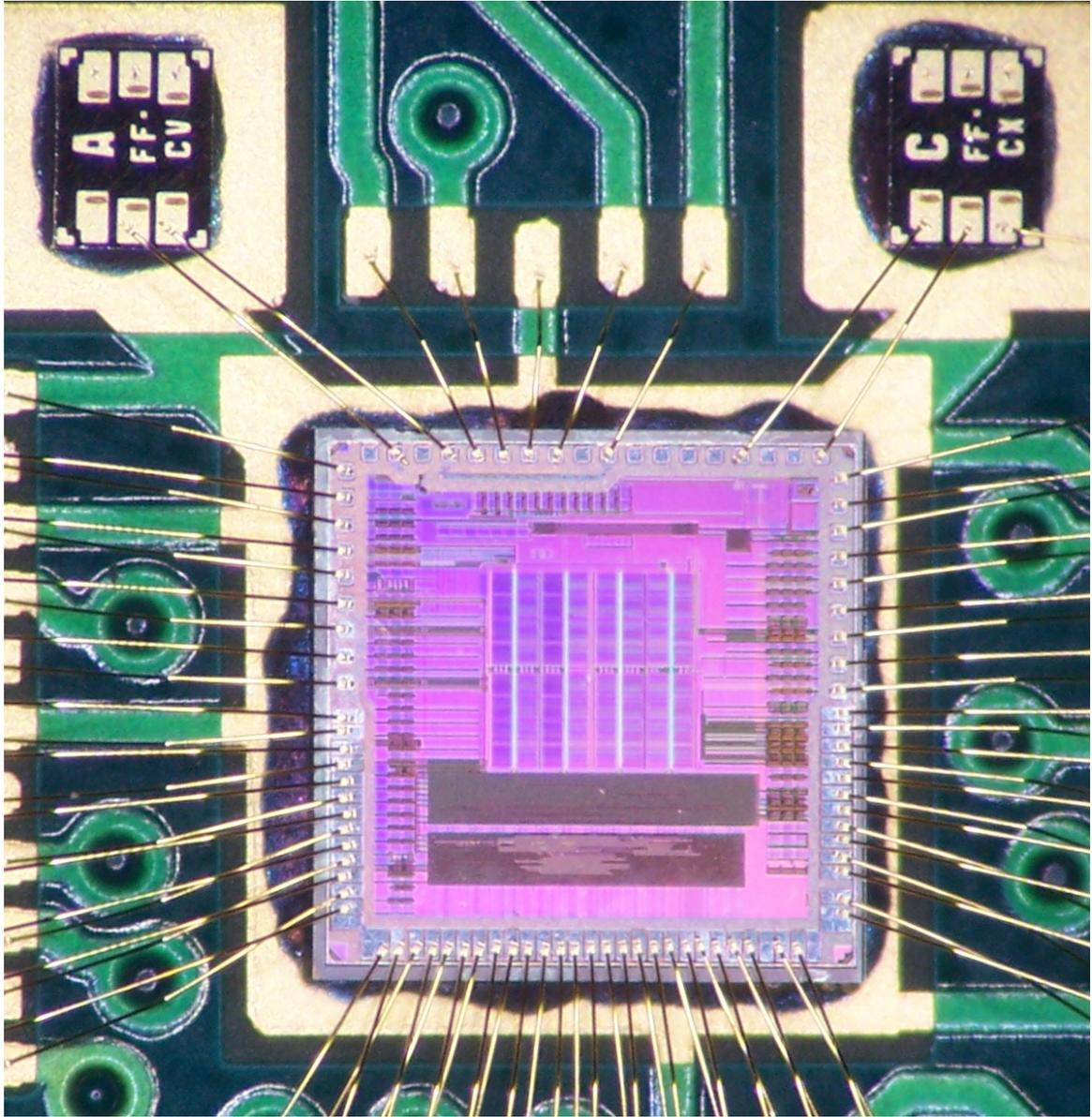
Figure 3.23: Die photo of bonded chip
