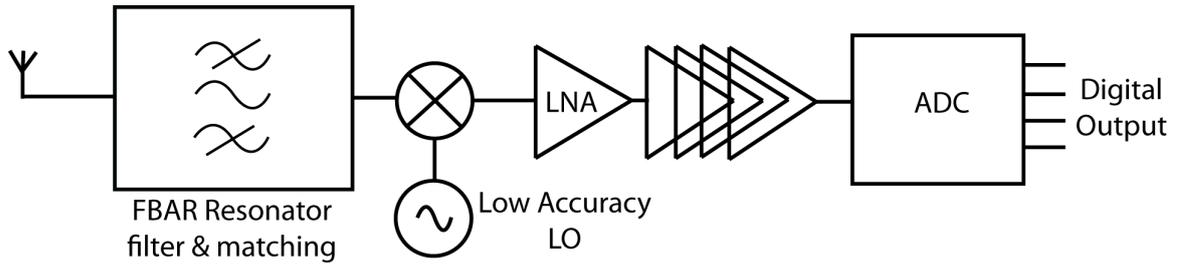
Figure 3.4: Block diagram of the Active RFID receiver
