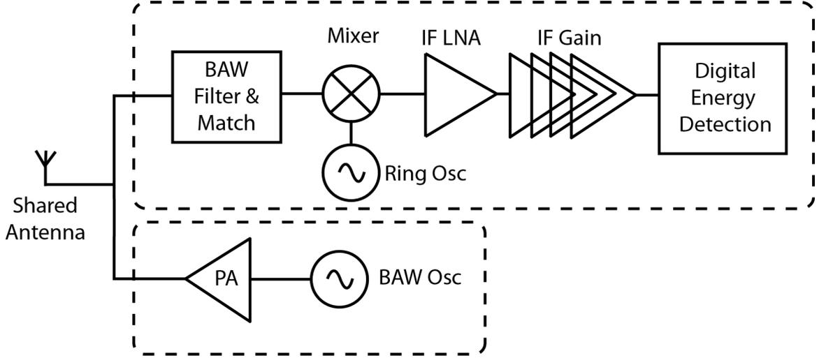
Figure 3.5: Block diagram of the complete transceiver
