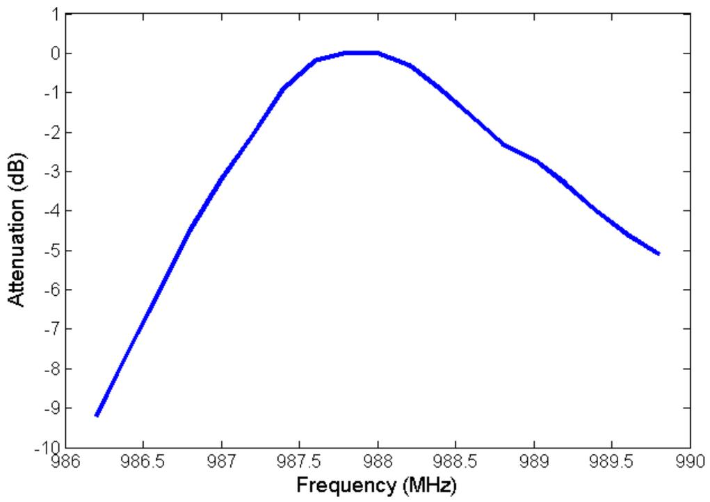
Figure 4.27: Measured Bandwidth
