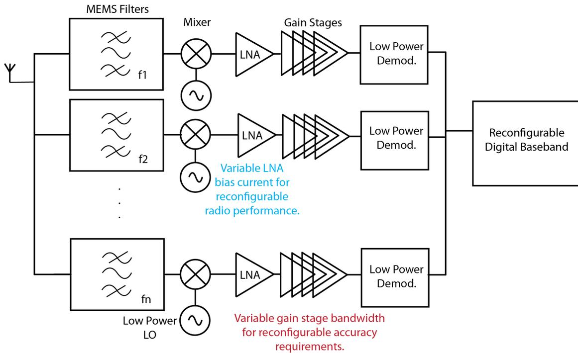
Figure 5.2: Multi-channel MEMS-based Receiver
