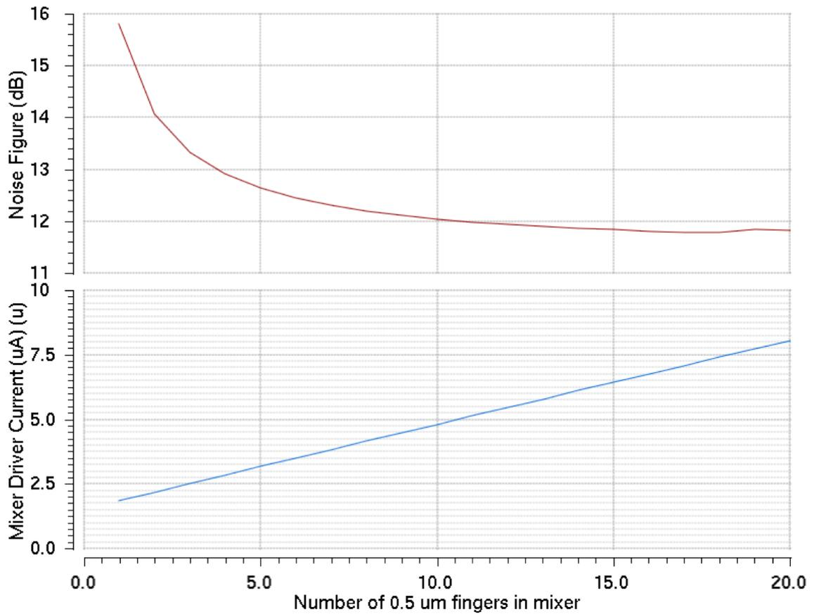
Figure 4.3: Noise figure and current versus the mixer size
