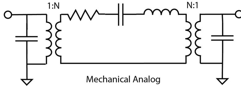
Figure 2.10: General model of a MEMS resonator.
