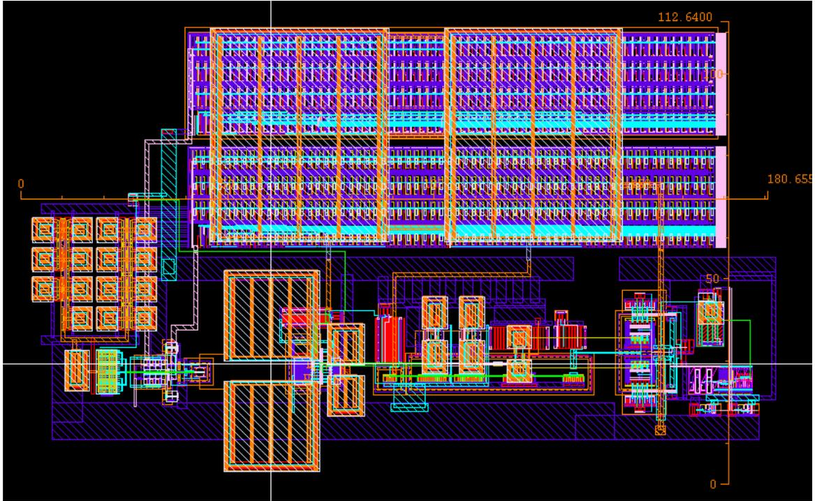
Figure 3.24: Layout of the receiver core
