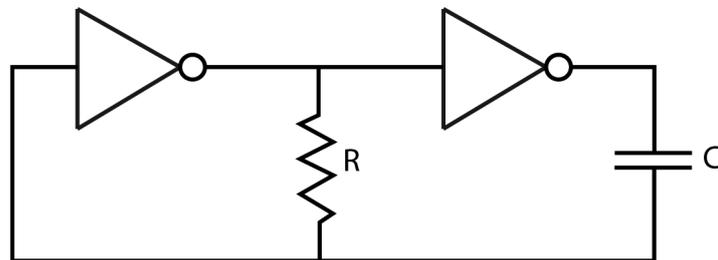
Figure 3.21: Relaxation oscillator for sampling clock
