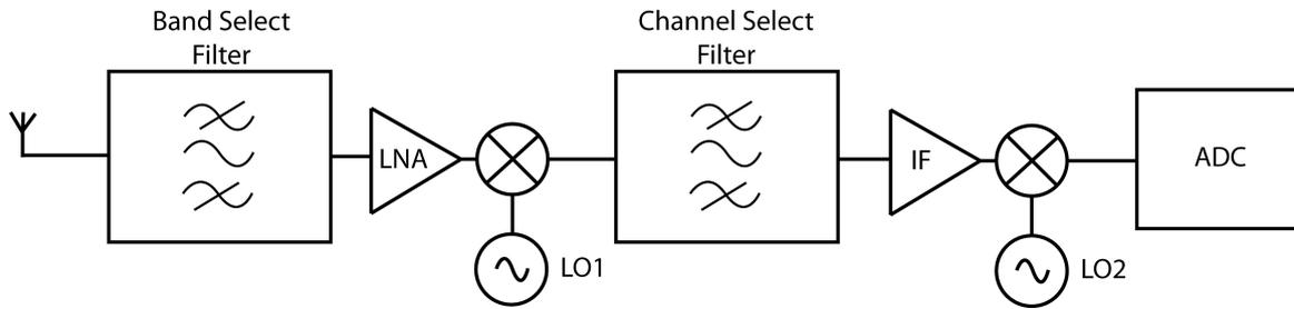
Figure 2.3: Traditional super-heterodyne architecture
