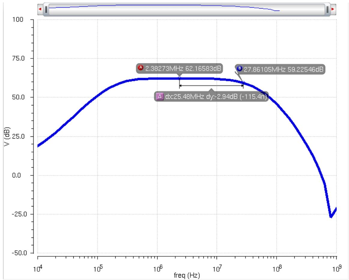
Figure 4.10: Simulated gain and bandwidth of IF amplifiers
