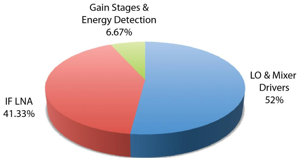
Figure 5.1: Power Consumption Breakdown for Wake-Up Radio from Chapter 4
