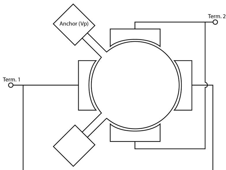
Figure 2.13: Basic design of a wineglass-mode vibrating disc resonator
