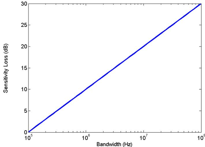
Figure 2.8: Sensitivity loss due to excess bandwidth, given a 100kbps data rate
