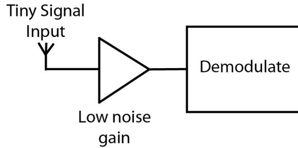
Figure 2.1: General digital receiver architecture
