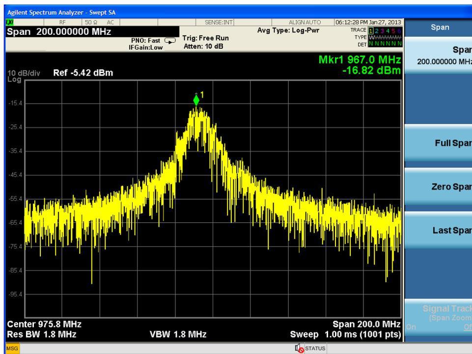
Figure 4.24: Measured ring oscillator output spectrum
