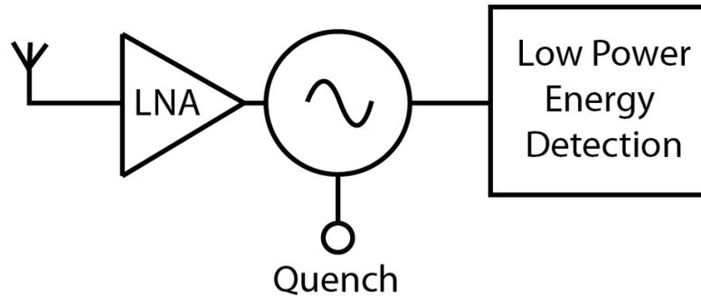
Figure 2.2: Super-regenerative Receiver Architecture
