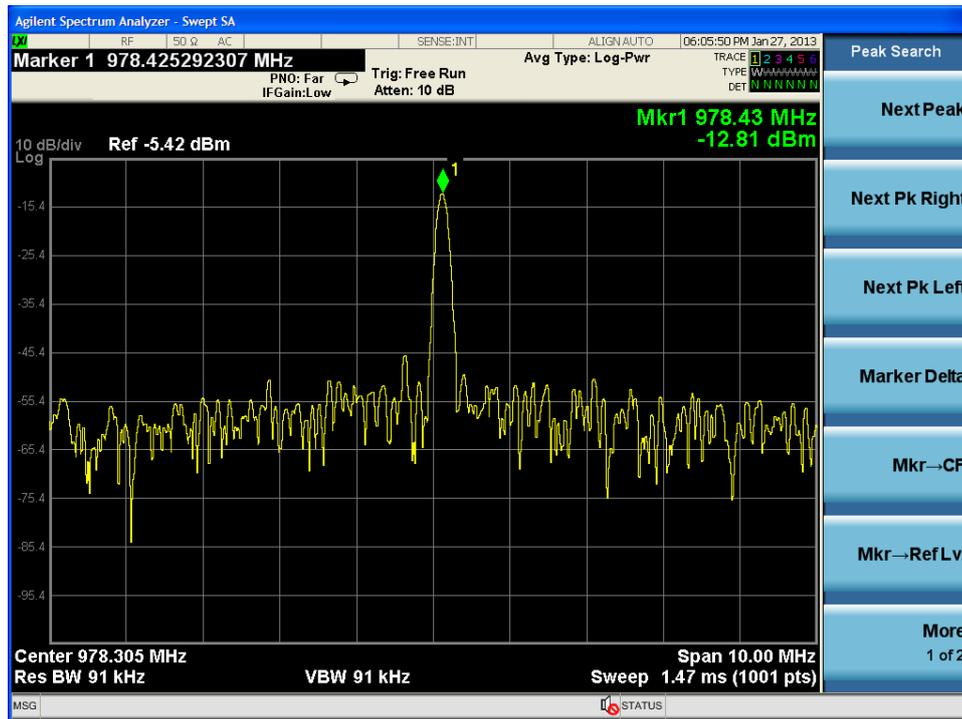
Figure 4.25: FBAR oscillator output spectrum
