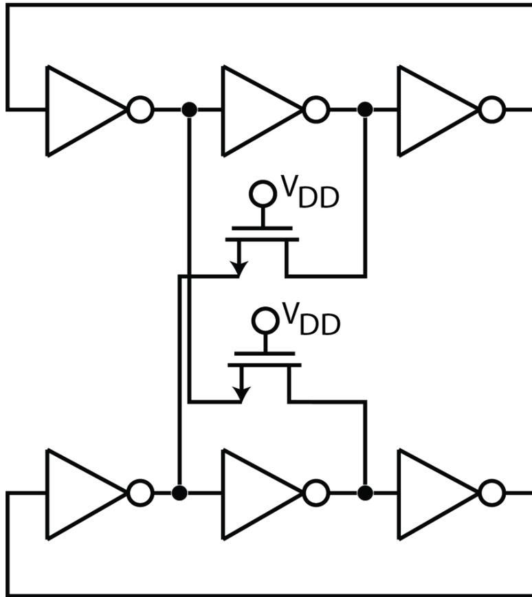
Figure 3.12: Ring oscillator core schematic, showing differential coupling
