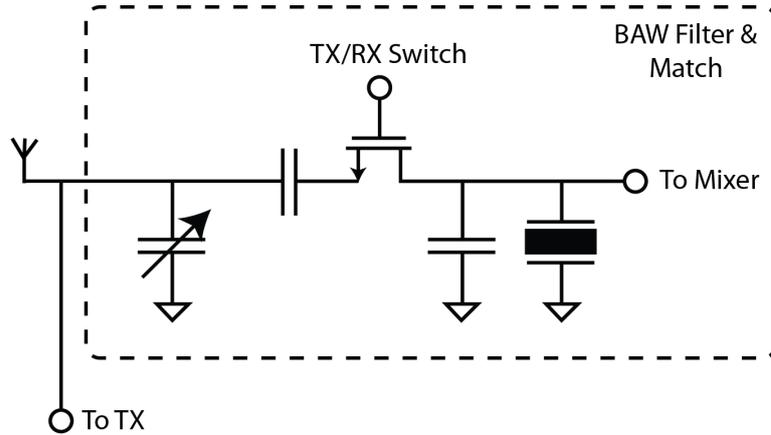
Figure 3.7: Matching network and TX/RX switch
