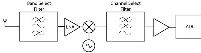
Figure 2.5: Direct conversion or low-IF receiver block diagram.
