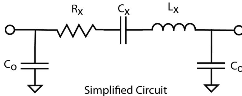
Figure 2.11: Simplified MEMS model
