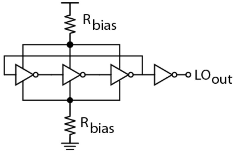
Figure 3.10: Ring oscillator for LO generation
