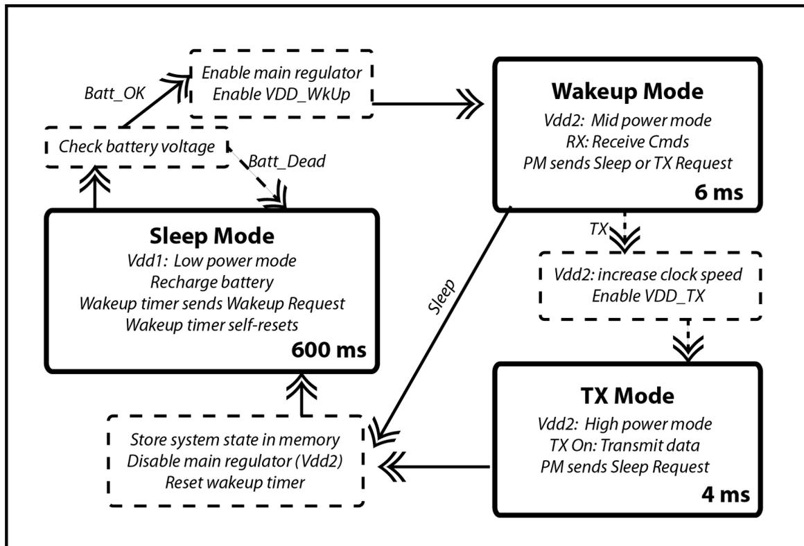
Figure 3.2: Operational modes of the Active RFID system
