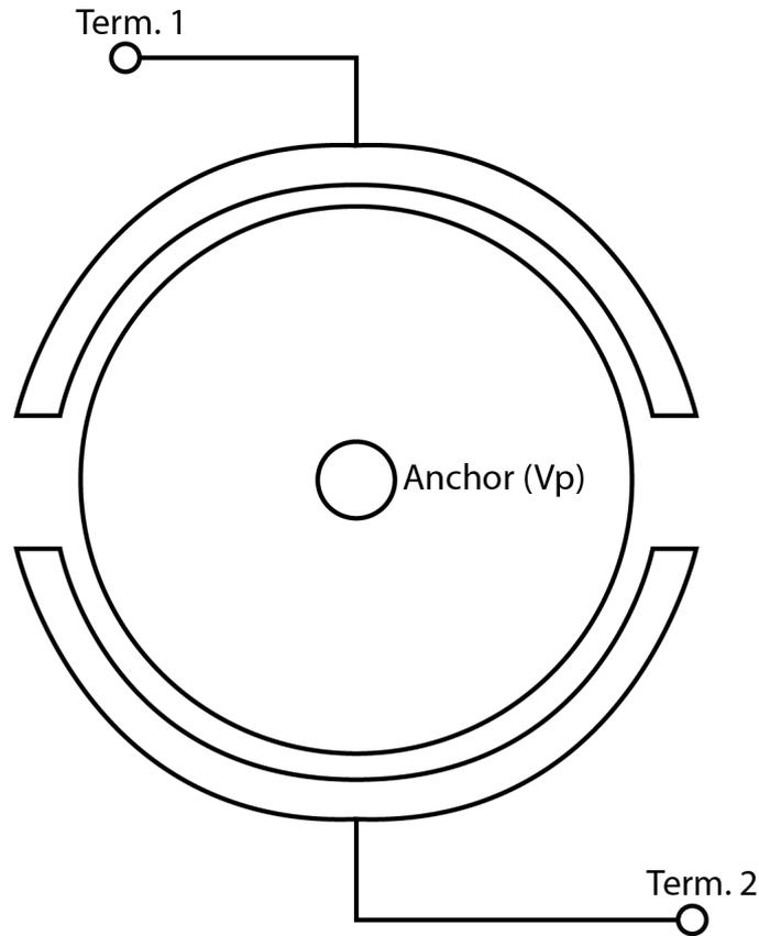
Figure 2.12: Basic design of a vibrating radial disc MEMS resonator
