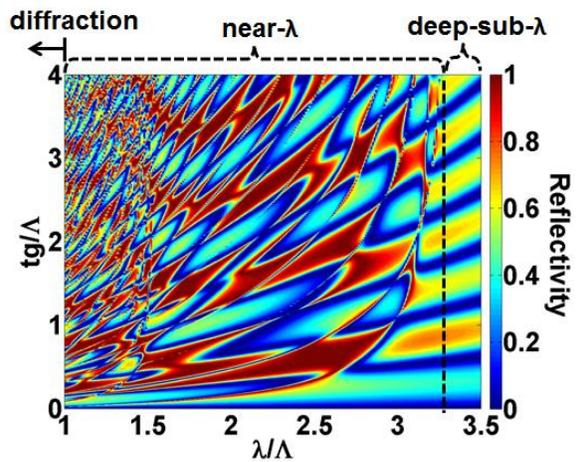
Figure 2.3 Reflectivity contour of HCGs as a function of wavelength and grating thickness. A fascinatingly well-behaved, highly ordered, checker-board pattern reveals its strong property dependence on both wavelength and HCG thickness, which indicates an interference effect. Surface normal incidence, oblique incidence for transverse HCG and oblique incidence for longitudinal HCG are shown.
