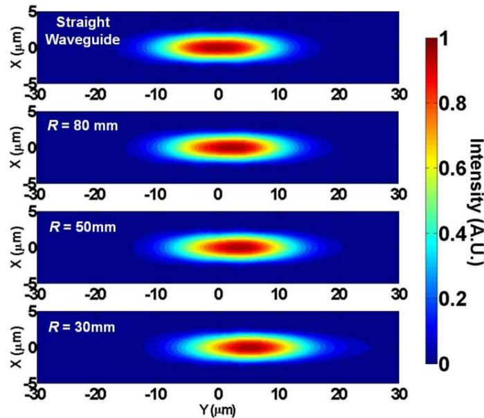
Figure 3.11 Mode profile for straight HCG HCW and curved HCG HCW with different radius of curvature  $R$ , simulated in FEM. The waveguide bends towards  $-y$  direction, with the center of the bending curvature at  $y = -R$ . The HCW height  $d = 6 \mu\text{m}$ .
