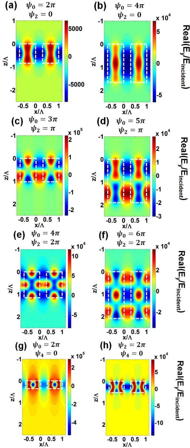
Figure 2.16 Field profile [ $\text{real}(E_y/E_{\text{incident}})$ ] of various HCG resonance at anti-crossings. The resonance conditions are labeled in the figures. HCG parameters:  $\eta=0.70$ ,  $n_{\text{bar}}=3.48$ , TE polarization light, surface normal incidence.
