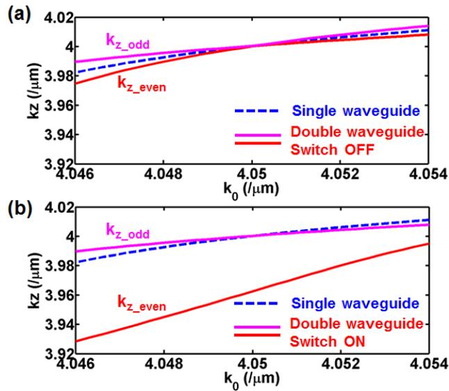
Figure 3.23  $\omega$ - $k$  diagram of the HCG-HCW extracted from Figure 3.22. The blue dashed curve is the  $\omega$ - $k$  diagram of the fundamental mode of a single HCW. When two such identical HCWs run in parallel, this mode splits into an odd mode and even mode, indicated by the magenta and red curves. (a) Switch OFF state; (b) Switch ON state.
