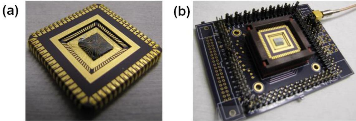
Figure 4.9 Image of an assembly of the optical phased array system. The chip is bonded on the chip carrier (a), which is hosted by a printed circuit board (b).
