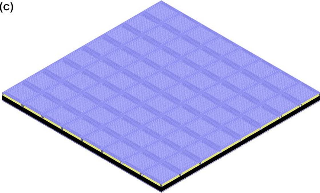
Figure 4.7 (a)(b) Schematic of an individual pixel of the optical phased array (with one-dimensional HCG). The  $\text{Al}_{0.6}\text{Ga}_{0.4}\text{As}$  HCG and 22 pairs of  $\text{GaAs}/\text{Al}_{0.9}\text{Ga}_{0.1}\text{As}$  DBR serve as the top and bottom reflector of the Fabry-Perot etalon. The incident light is surface normal to the etalon, and polarized parallel to the grating bar. (c) Schematic of an 8x8 optical phased array.
