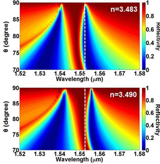
Figure 3.20 Reflectivity contour of an HCG resonance design as a function of incident angles  $\theta$  and wavelengths, for the grating bar refractive index of 3.483 (a) and 3.490 (b). At the same wavelength (1.553  $\mu\text{m}$ , indicated by the white dashed line), the HCG can change from highly transparent to highly reflective, with the grating bar index change from 3.483 to 3.490.
