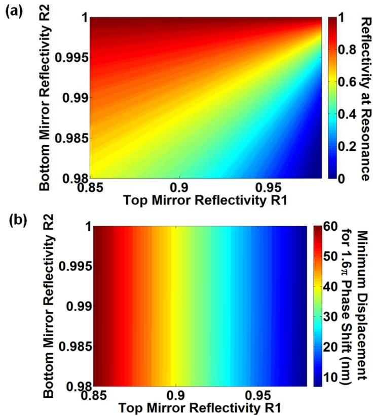
Figure 4.6 (a) Reflectivity contour of the FP cavity at resonance as a function of the top mirror reflectivity  $R_1$  and bottom mirror reflectivity  $R_2$ . (b) Minimum mirror displacement to reach a reflection phase shift of  $1.6\pi$ , as a function of  $R_1$  and  $R_2$ .
