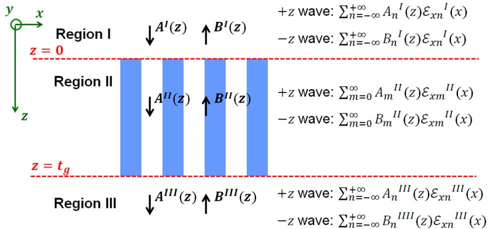
Figure 2.9 General formulation of the electric field in Region I, II and III of the HCG.
