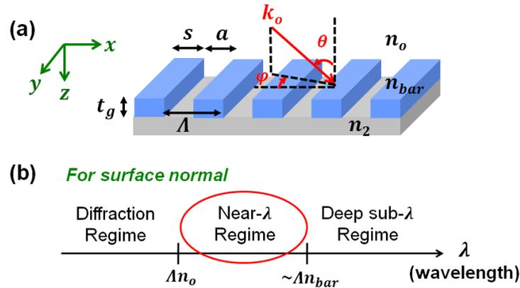
Figure 1.1 (a) Generic HCG structure. The grating comprises of simple dielectric bars with high refractive index  $n_{bar}$ , surrounded by a low index medium  $n_o$ . A second low-index material  $n_2$  is beneath the bars. (b) The three operation region for gratings. High contrast grating operates at the near-wavelength regime.
