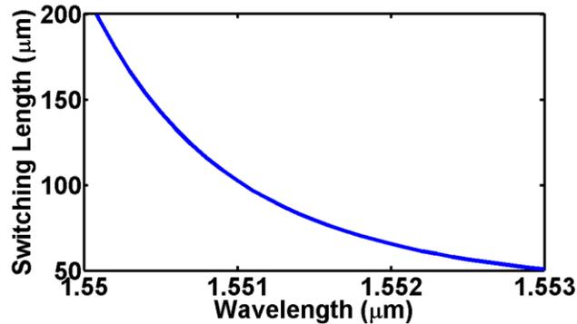
Figure 3.26 Switching length versus different wavelength for the HCG HCW switch.
