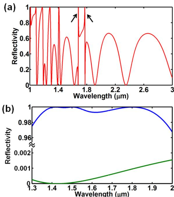
Figure 2.2 Examples of three types of extraordinary reflectivity / transmission features of HCG. (a) High-Q resonances (red). (b) Broad-band high reflection (blue), and broad-band high transmission (green).
