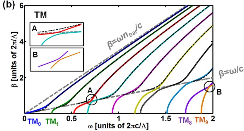
Figure 2.5 Dispersion curves ( $\omega$ - $\beta$  diagram) of a waveguide array (solid) and a single slab waveguide (dash), for the same bar width  $s$  and index  $n_{bar}$ ,  $\beta$  being the  $z$ -wavenumbers. In this calculation,  $\eta=0.6$ ,  $n_{bar}=3.48$ ,  $\theta=50^\circ$ .
