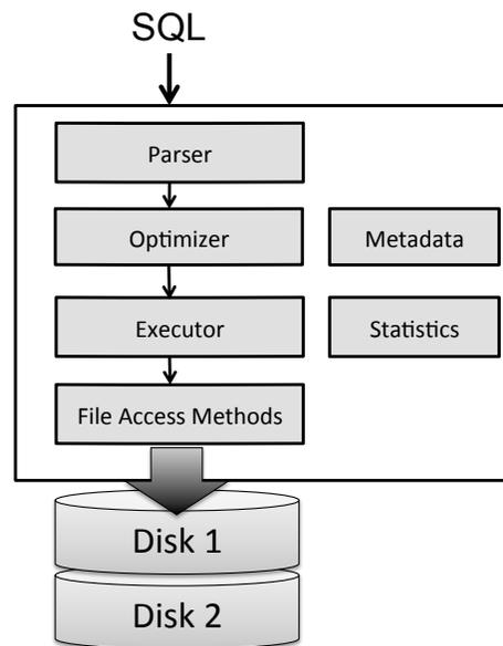
Figure 3.1: Architecture of a RDBMS with core components related to query processing
