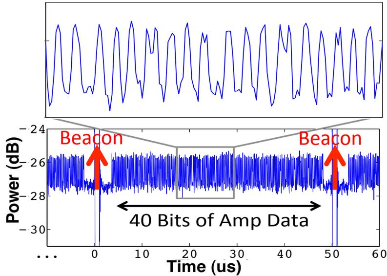
Figure 3.18: A wireless packet encoded with Miller modulation. Backscatter communication of 40 bits of signal acquisition data is initiated by a pulse from the transmitter (seen on either side of the packet).
