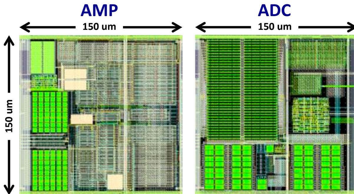
Figure 4.15: Layout of the amplifier and ADC.
