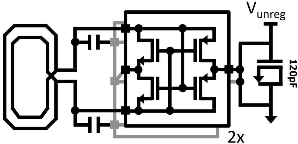
Figure 3.8: A high- $R_p$  on-chip coil increases the open circuit voltage and maximizes the efficiency of the self-synchronous rectifier. 120 pF of on-chip decoupling capacitance is implemented with thick-oxide native devices.
