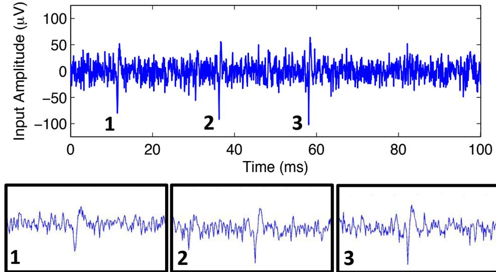
Figure 3.24: One example trial of wirelessly powered *in vivo* neural data from a live rat. The LFP feedback cancellation high-pass corner was set and measured to be approximately 500 Hz.
