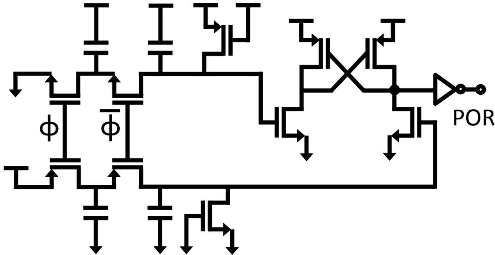
Figure 3.12: Power-on reset schematic. Switched-capacitor resistors pull up against pseudo-resistors, disabling the reset signal after several clock cycles.
