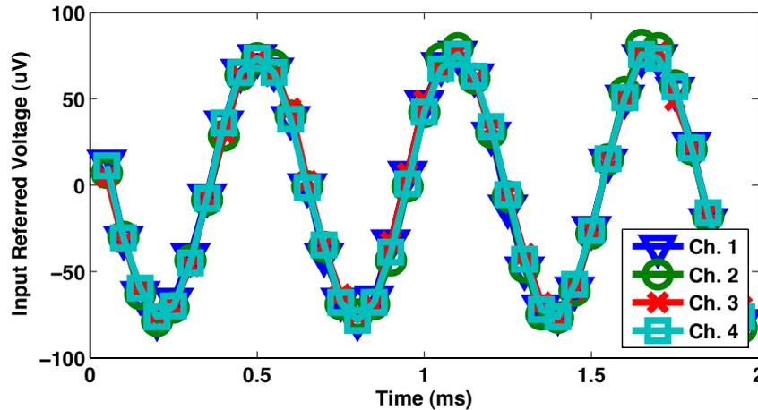
Figure 3.22: A wirelessly-powered system recording and transmitting a 1.6 kHz, 150  $\mu\text{V}$  sine wave input from all channels simultaneously.
