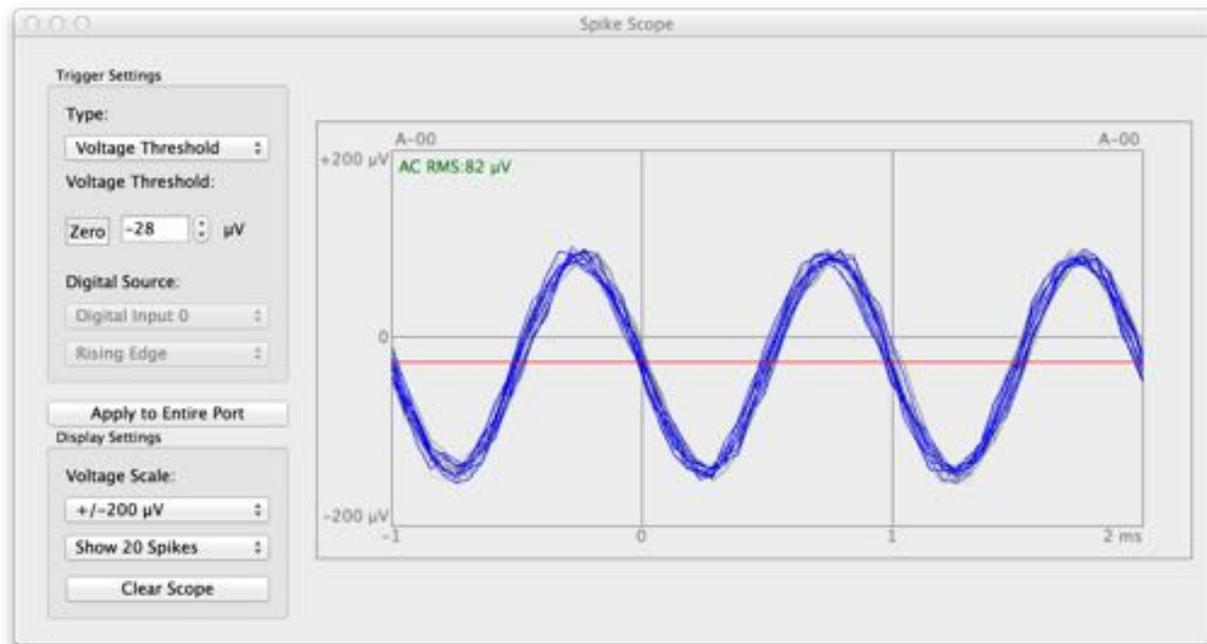
Figure 4.29: A screen capture of the GUI in overlay mode with test signals present. The GUI is able to display detected spike overlays using data from either the chip epochs or from full-streams using NEO or threshold-based software spike detection.
