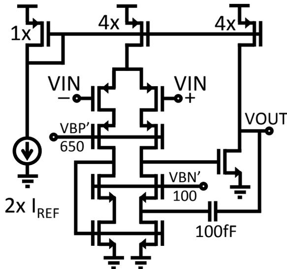
Figure 4.9: ADC buffer core schematic.
