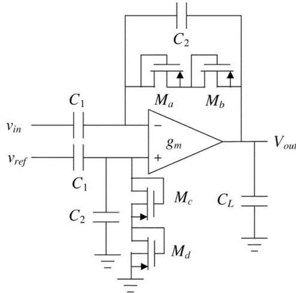
Figure 1.9: Widely-used amplifier topology proposed in 2002 by Harrison [48].
