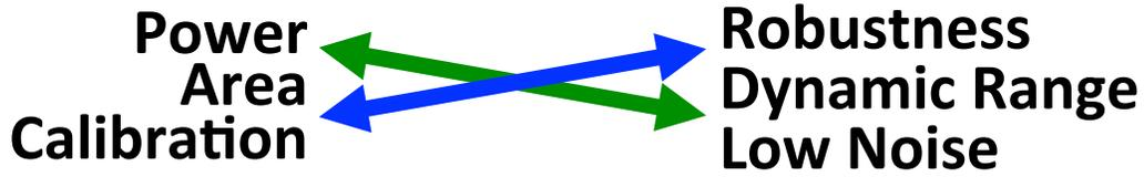
Figure 1.10: Design tradeoffs for a neural acquisition channel.
