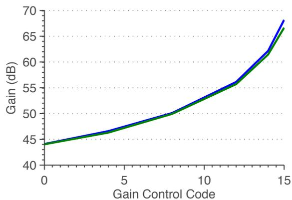
Figure 4.21: Measured (green) and simulated (blue) LNA & VGA gain vs. control code.
