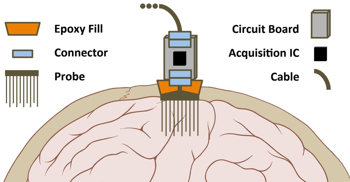
Figure 1.6: A conventional wired neural interface. Adapted from [24].
