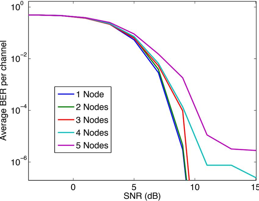
Figure 3.21: Simulated BER vs. SNR for 1-5 simultaneous nodes.
