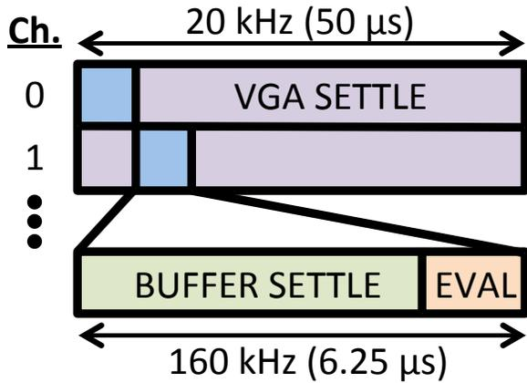
Figure 4.11: Buffer and ADC timing diagram.
