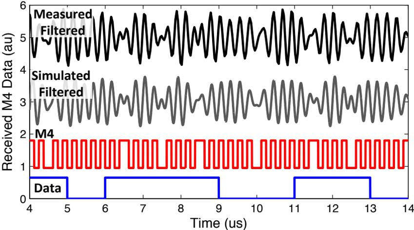
Figure 3.20: The measured time domain waveform after filtering of M4 during a multi-node interrogation test. Results are compared to an ideal filtered waveform, and the equivalent Miller waveform with decoded data is shown.
