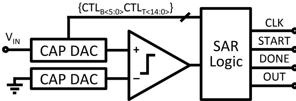
Figure 4.13: ADC top level schematic.
