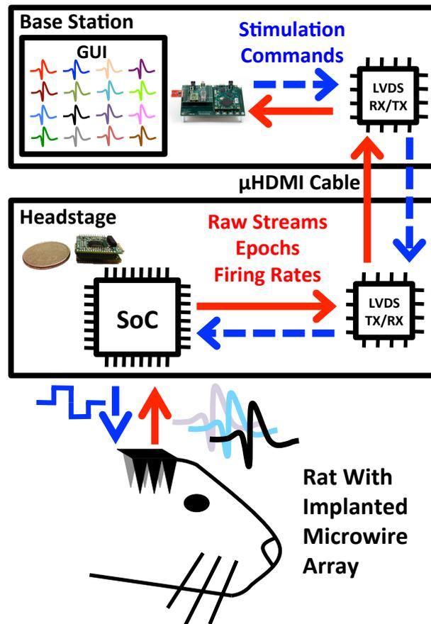
Figure 4.27: The *in vivo* neuromodulation test system is composed of a microwire implanted array, a compact headstage containing the SoC, a base station, and a Graphical User Interface (GUI).
