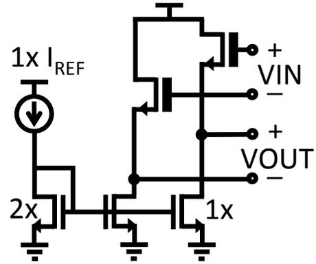
Figure 4.7: LNA & VGA DC feedback level shifter schematic.
