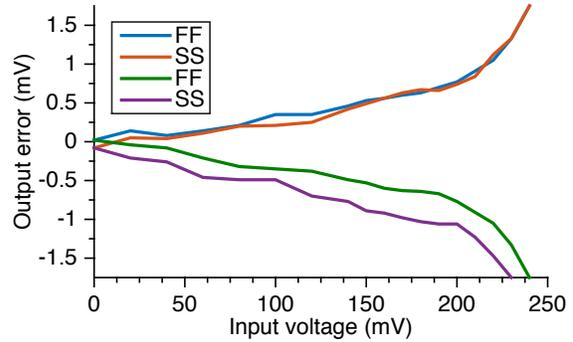
Figure 4.12: Simulated ADC buffer settling error versus input voltage (full scale input = 250 mV).
