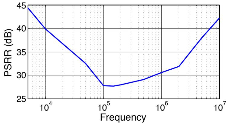
Figure 3.11: The measured discrete-time LDO regulator supply rejection across frequency.
