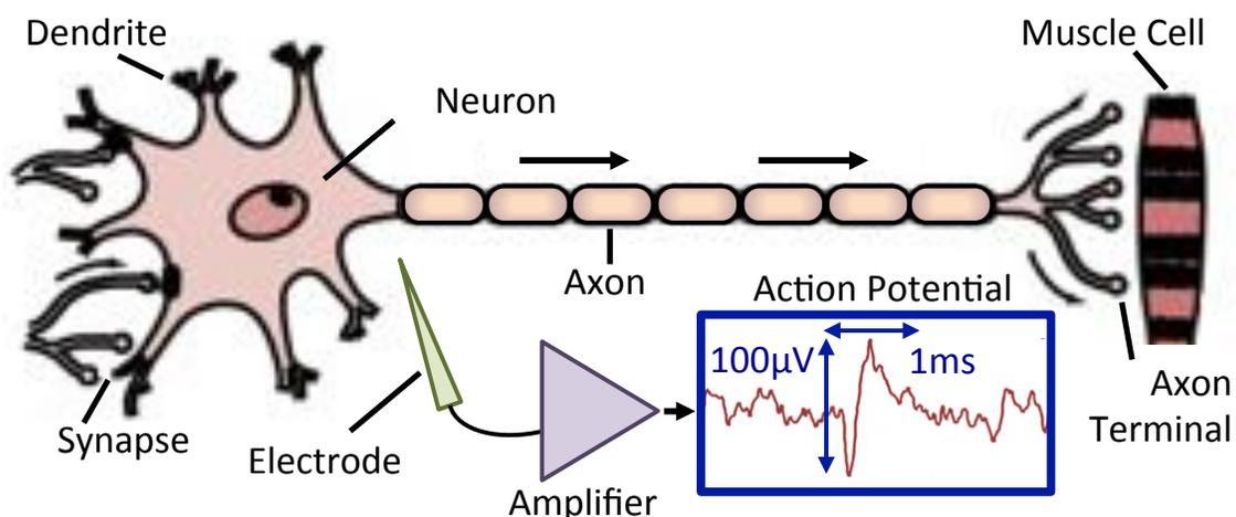
Figure 1.1: A neuron transmits action potentials through its axon to other neurons as well as organs such as muscles. A low-noise amplifier magnifies the electrical potential as measured by an extracellular electrode. Adapted from [2].
