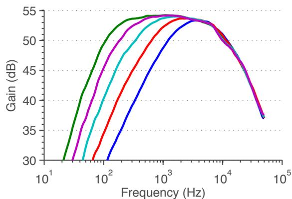
Figure 4.19: Measured bode plot LNA & VGA with gain set to 500 vs. selected high-pass corner settings.
