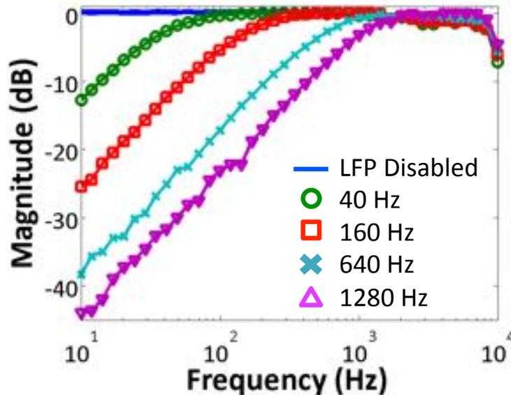
Figure 3.14: Measured amplifier frequency response over various high-pass corners, normalized to peak gain.
