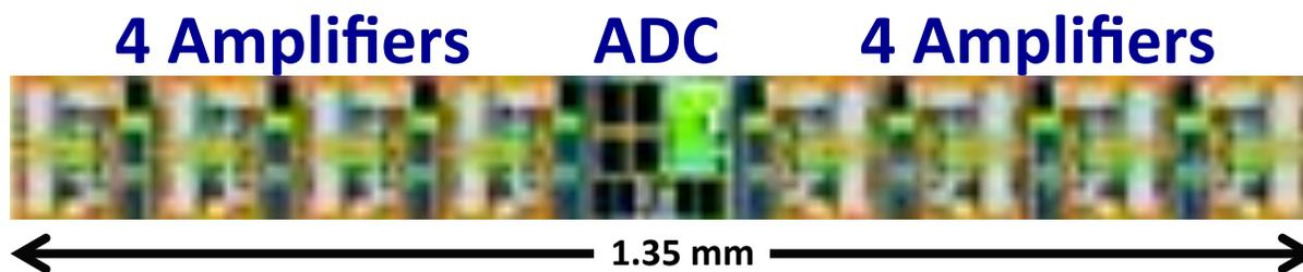
Figure 4.16: Layout of a row of 8 amplifiers and 1 ADC.
