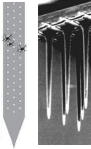
Figure 1.7: Planar (left) and needle (right) neural probes. A rough scale for the size of a neuron can be seen in the planar probe, where the exposed electrodes are  $30\ \mu\text{m}$  in diameter. Probes range from 1-5 mm in length. Images adapted from [36] and [41].
