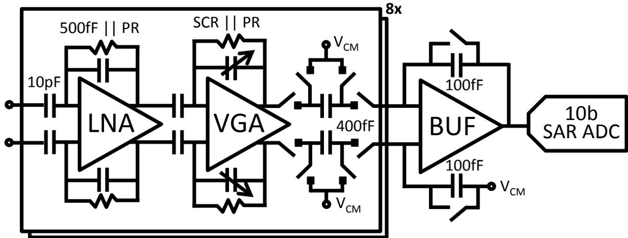
Figure 4.3: Block diagram of a recording channel row. Eight rows, each containing 8 amplifiers time-multiplexed onto a 10-bit SAR ADC, comprise the 64 channel array.
