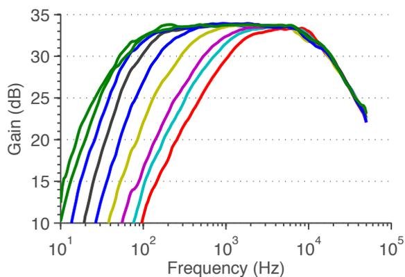
Figure 4.18: Measured bode plot of LNA & VGA with gain set to 50 vs. selected high-pass corner settings.
