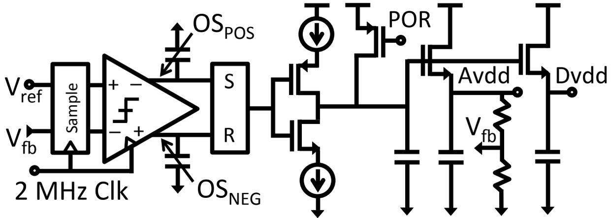
Figure 3.10: Discrete-time LDO regulator schematic utilizing a comparator with capacitive offset cancellation and a charge pump loop filter.
