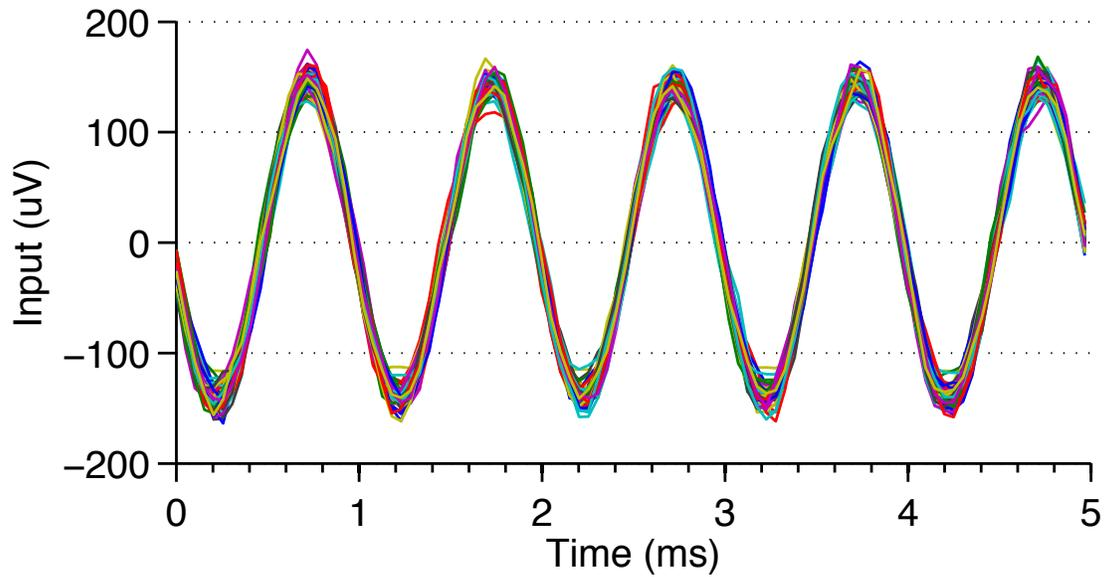
Figure 4.22: Gain matching for the array, at the highest gain setting.
