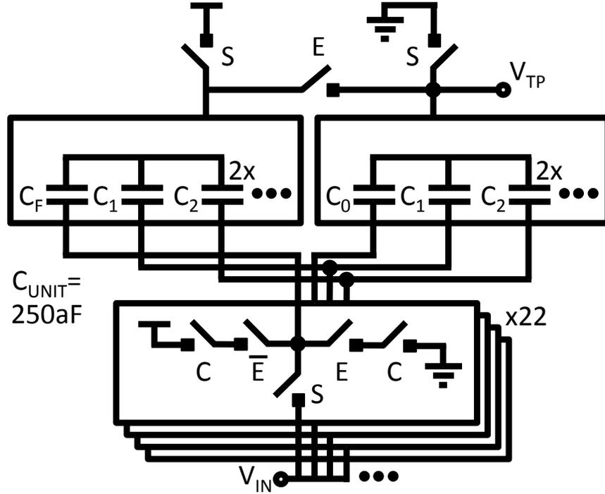
Figure 4.14: Bottom-plate sampled ADC capacitor array with sampling and evaluation switches. The array is composed of unit capacitors; half of the unit capacitors for each bit are sampled with respect to VDD and GND, respectively, which creates an effective 500 mV reference.
