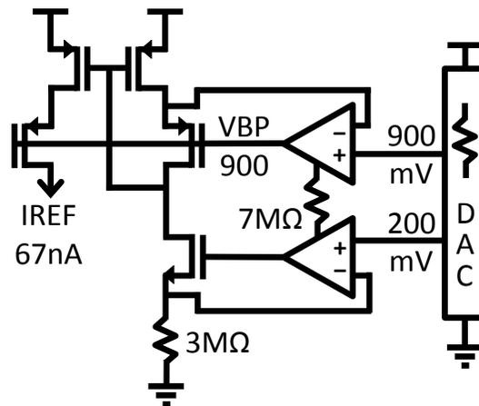
Figure 4.8: Bias current and 900mV cascode bias (“VBP900”) generation.
