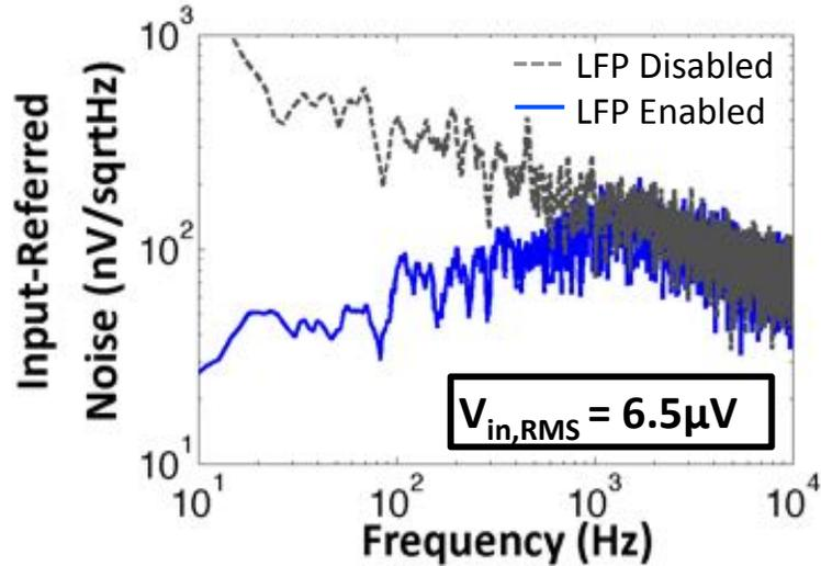
Figure 3.16: Measured amplifier noise spectrum with and without the LFP loop enabled.
