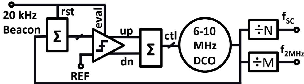
Figure 3.7: Frequency-locked loop for subcarrier generation. Recovered beacons reset the accumulator (*rst*) and evaluate the comparator (*eval*). The comparator increments or decrements the second accumulator (*up/dn*), which in turn controls the DCO tuning bits (*ctl*). Finally, programmable dividers generate the output Miller subcarrier ( $f_{sc}$ ) and internal 2 MHz clock ( $f_{2MHz}$ ).
