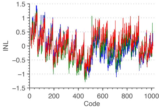
Figure 4.26: Measured ADC INL for 4 chips, with a peak of approximately 1.5 bits. The average INL for the 4 samples is overlaid as a dark blue trace.
