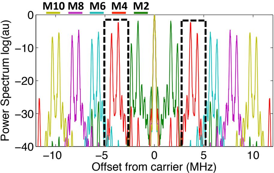
Figure 3.3: Theory of a Miller encoded communication scheme for multi-node interrogation showing the resulting frequency spectrum from 5 nodes communicating simultaneously.
