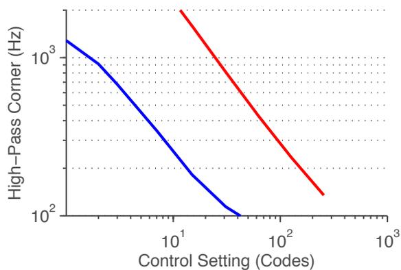
Figure 4.20: Measured VGA high-pass corner vs. control code at gain of 50 (blue) and 500 (red) V/V.
