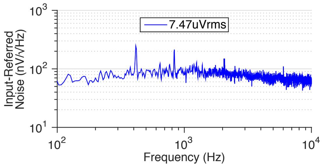
Figure 4.23: Measured amplifier input referred noise spectral plot.
