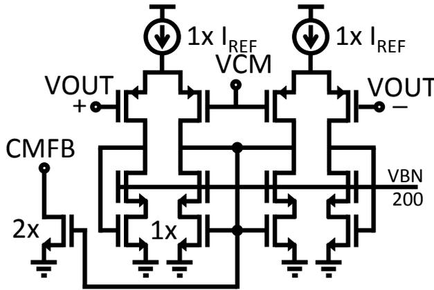
Figure 4.6: LNA & VGA CMFB schematic.
