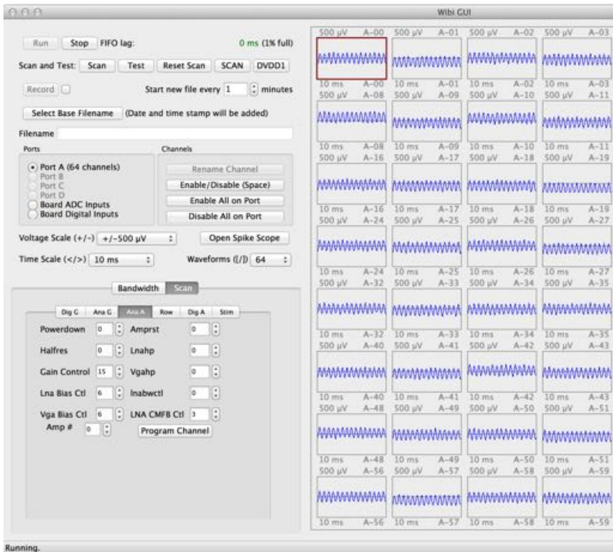
Figure 4.28: A screen capture of the GUI with test signals present. The GUI is able to display waveforms in real time as well as log data to a file.
