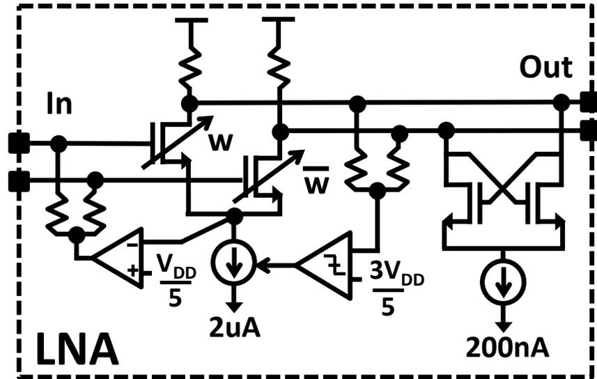
Figure 3.15: Amplifier front-end calibration, input and output common mode biasing, and cross-coupled gain boost.
