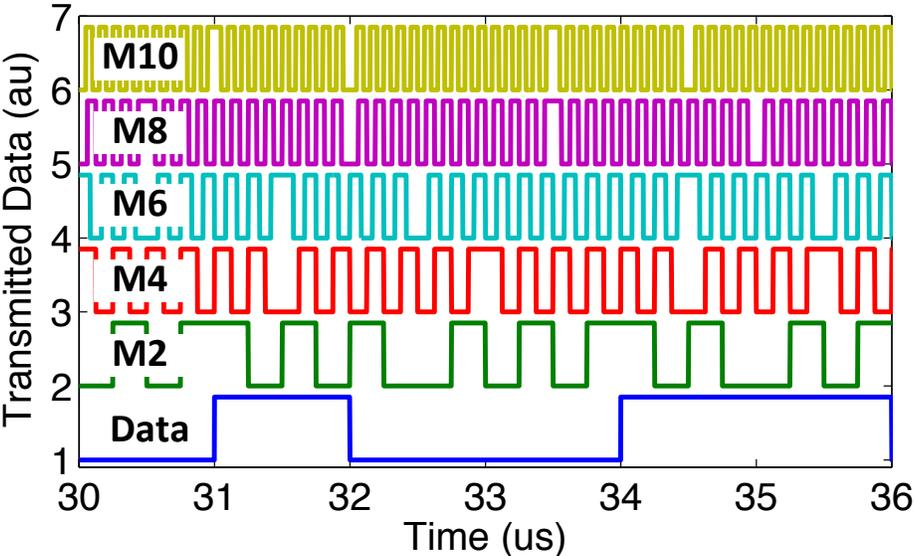
Figure 3.2: Theory of a Miller encoded communication scheme for multi-node interrogation showing miller encoded waveforms (2,4,6,8,10 MHz) for a data set.
