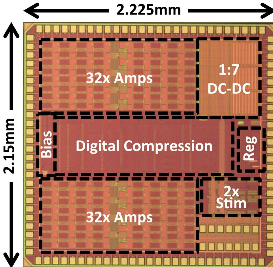
Figure 4.17: Die photo of the 64-channel recording, dual stimulation and integrated compression IC.
