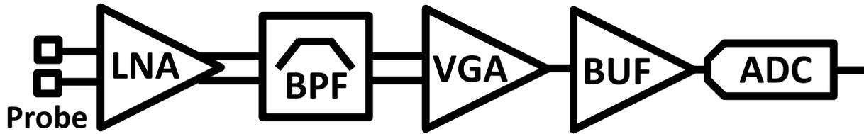
Figure 1.8: Typical components of a neural acquisition channel.
