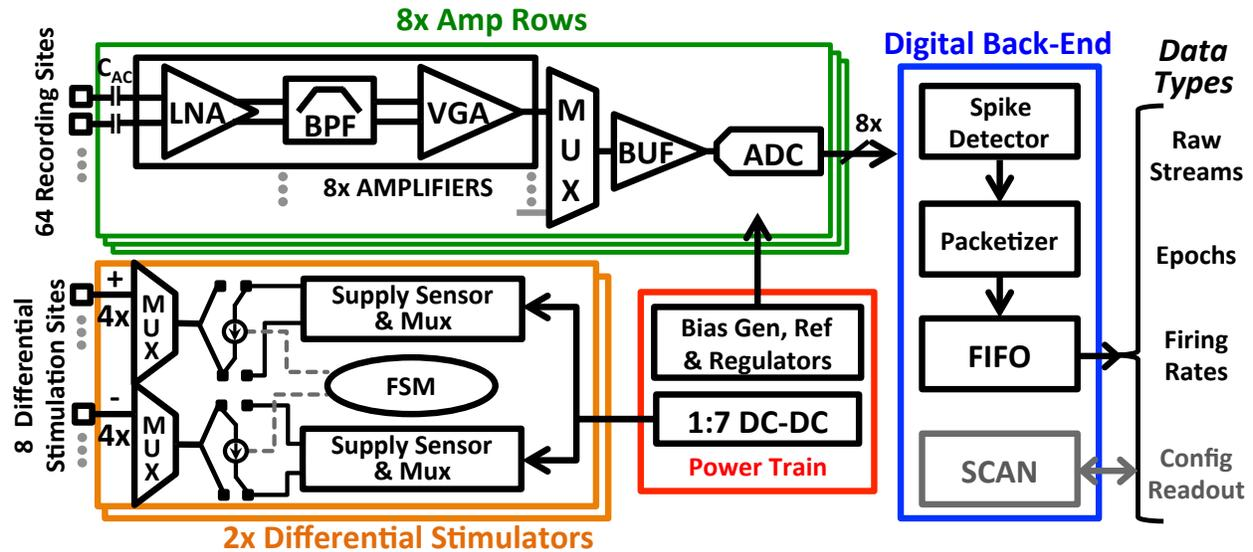
Figure 4.2: Berkeley wireless neural interface chip block diagram.
