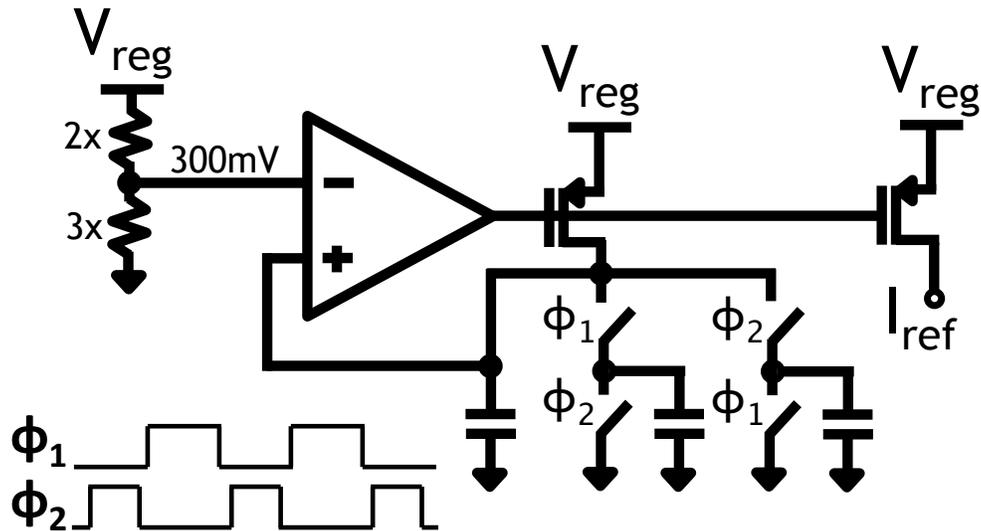
Figure 3.9: Switched-capacitor bias current generation schematic, utilizing two-phase non-overlapping clocks.
