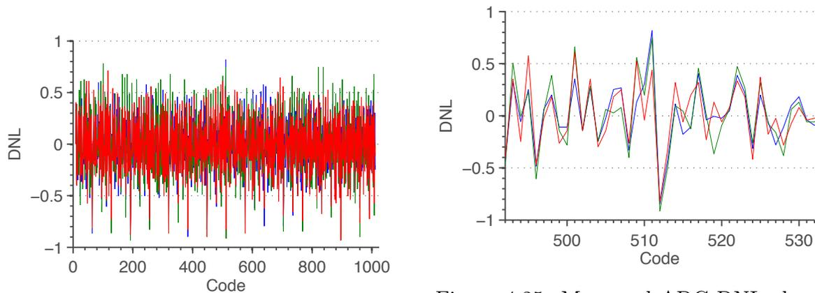
Figure 4.24: Measured ADC DNL for 4 chips, with a peak of 1 bit.
