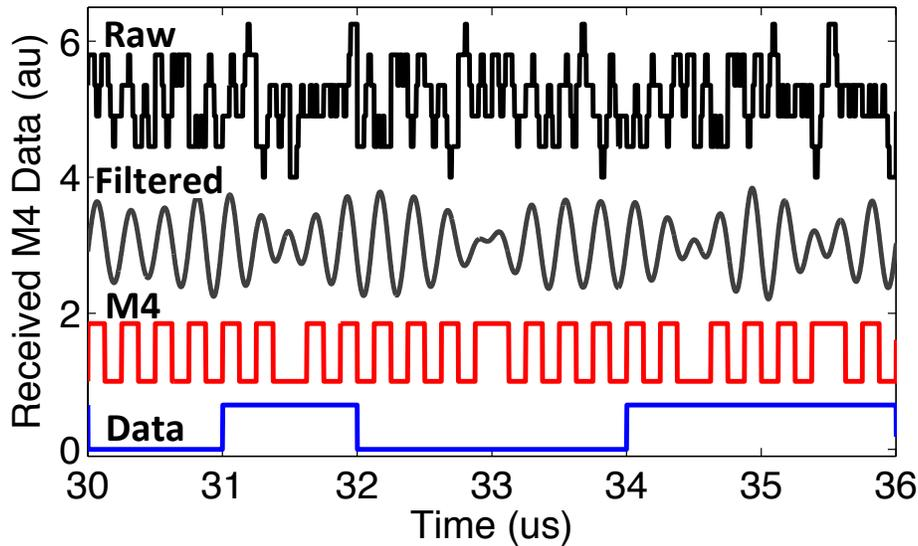
Figure 3.4: Theory of a Miller encoded communication scheme for multi-node interrogation showing the recovered raw waveform before and after bandpass filtering, and the recovered original transmitted M4 signal and equivalent data.
