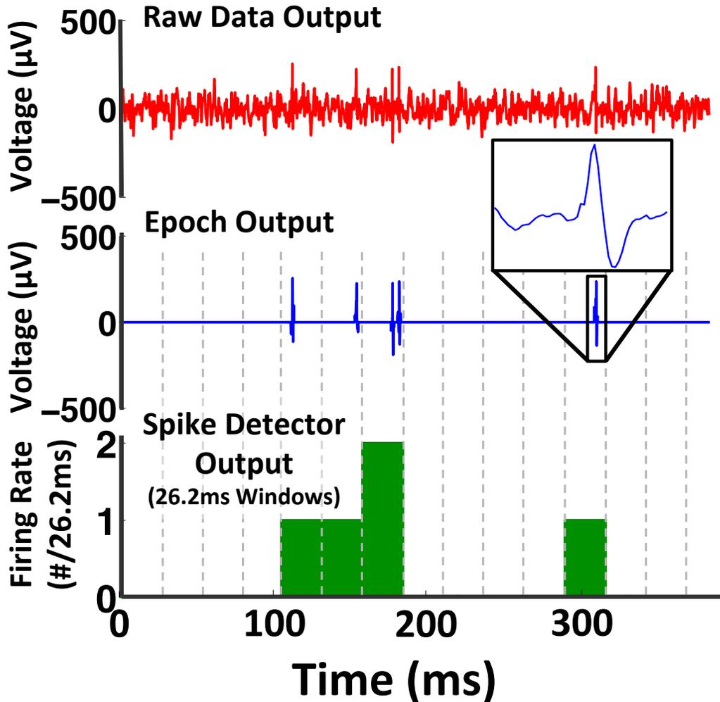
Figure 4.31: Raw streams, epochs, and firing rates of *in vivo* recorded data.
