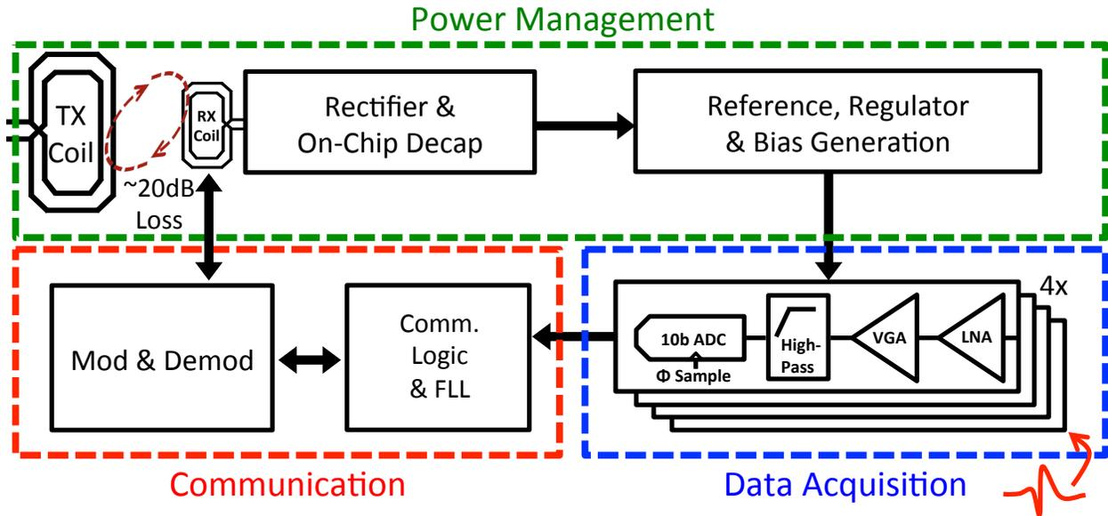
Figure 3.5: System diagram, subdivided into three primary circuit blocks: Power management, communication circuitry, and data acquisition.
