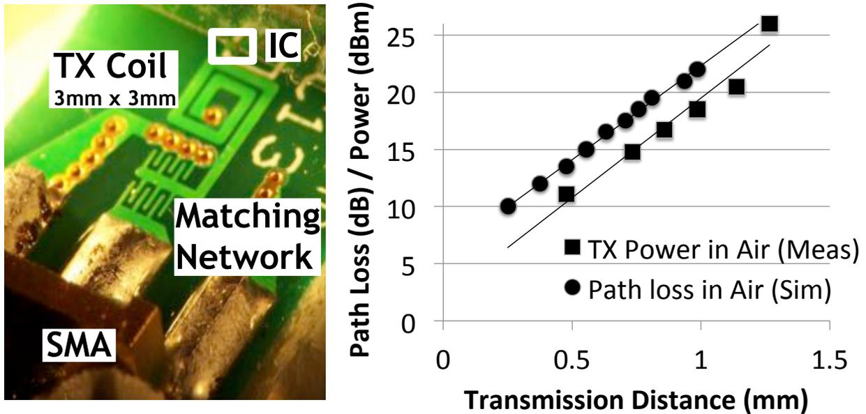
Figure 3.17: Left: Setup for wireless operational range testing. The IC is attached to a micro-manipulator using double-sided tape. Right: Simulated path loss compared to the measured minimum TX power required for operation in air.
