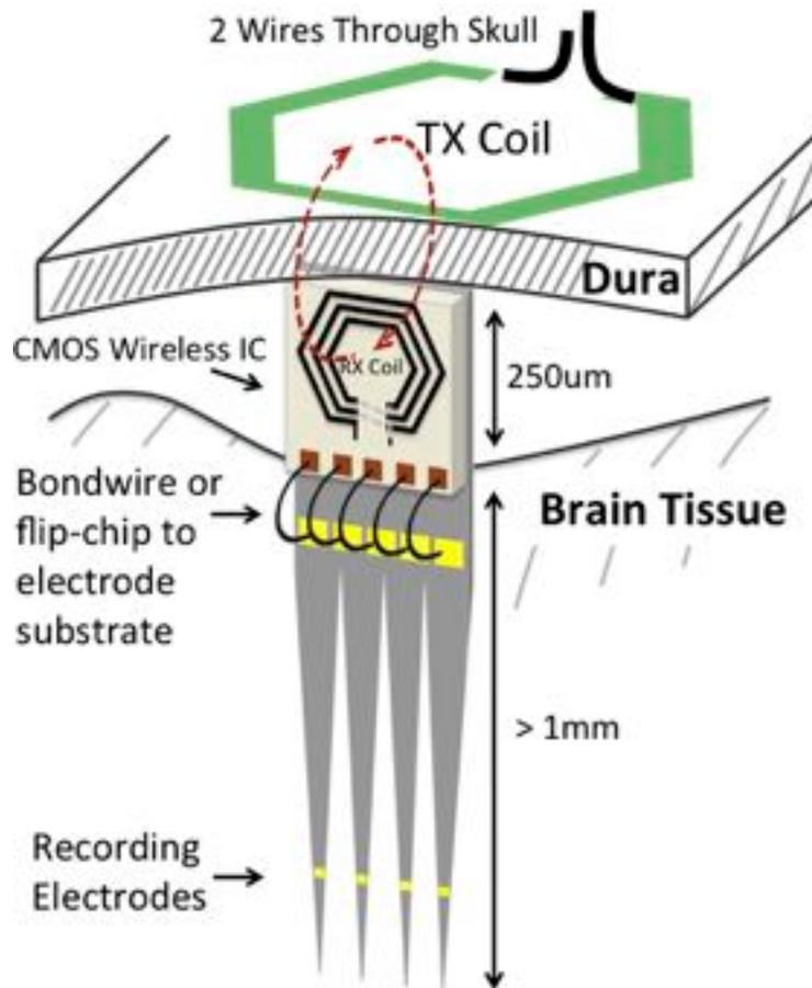
Figure 3.1: A conceptual diagram of the implementation of a BMI utilizing the developed wireless neural sensor. The sensor free-floats under the dura, while receiving power from and communicating to an interrogator beneath the skull.
