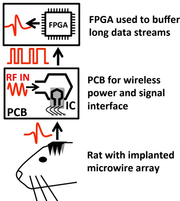
Figure 3.23: The setup for *in vivo* recording trials utilized a rat which was implanted with a microwire array. The system was die-attached to a PCB to facilitate wireless powering and signal interfacing. In order to gather long data streams, a FPGA was used to buffer the on-chip Miller-encoded neural data.
