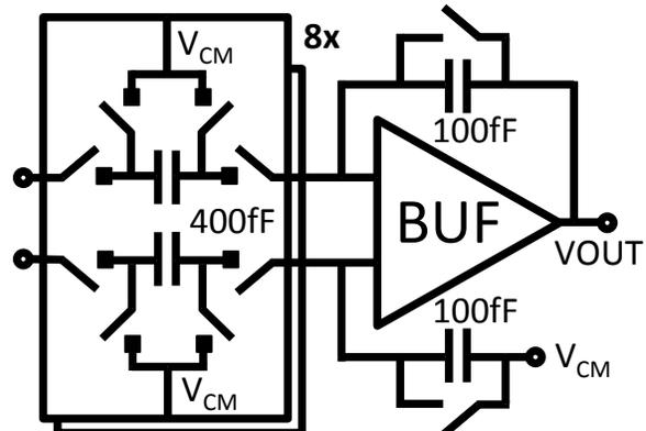
Figure 4.10: Buffer feedback schematic.
