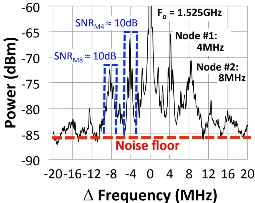
Figure 3.19: Frequency spectrum of two wirelessly powered nodes, communicating simultaneously with the same interrogator at different sub-carrier frequencies.
