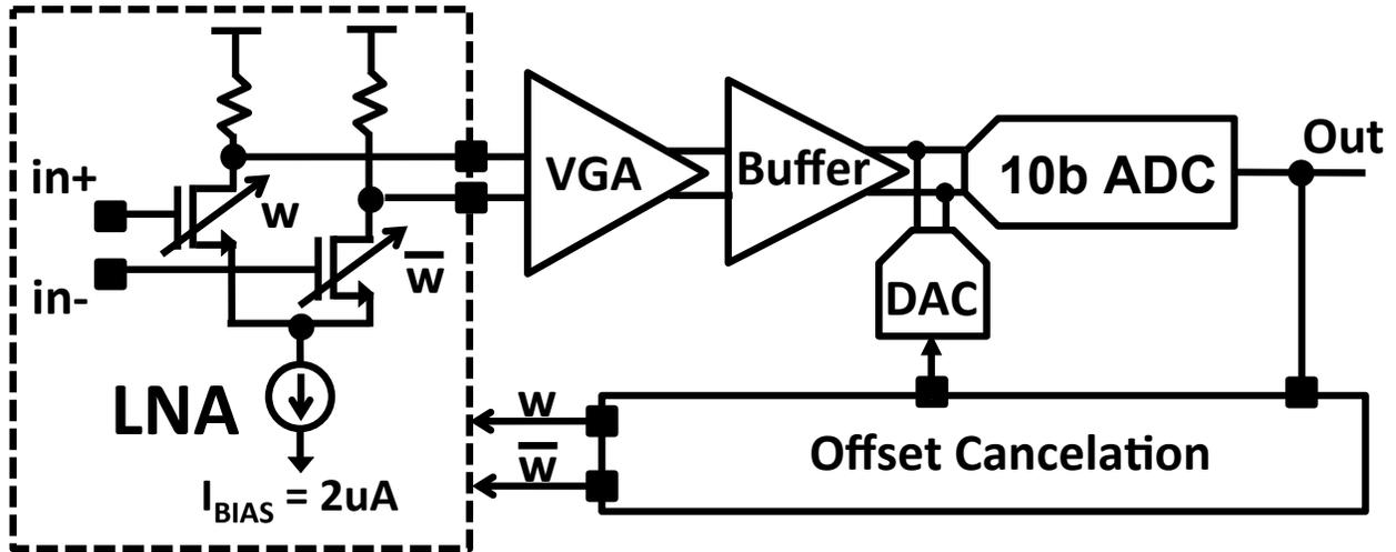
Figure 3.13: Amplifier block diagram utilizing mixed signal feedback to cancel DC offset and LFP signal.
