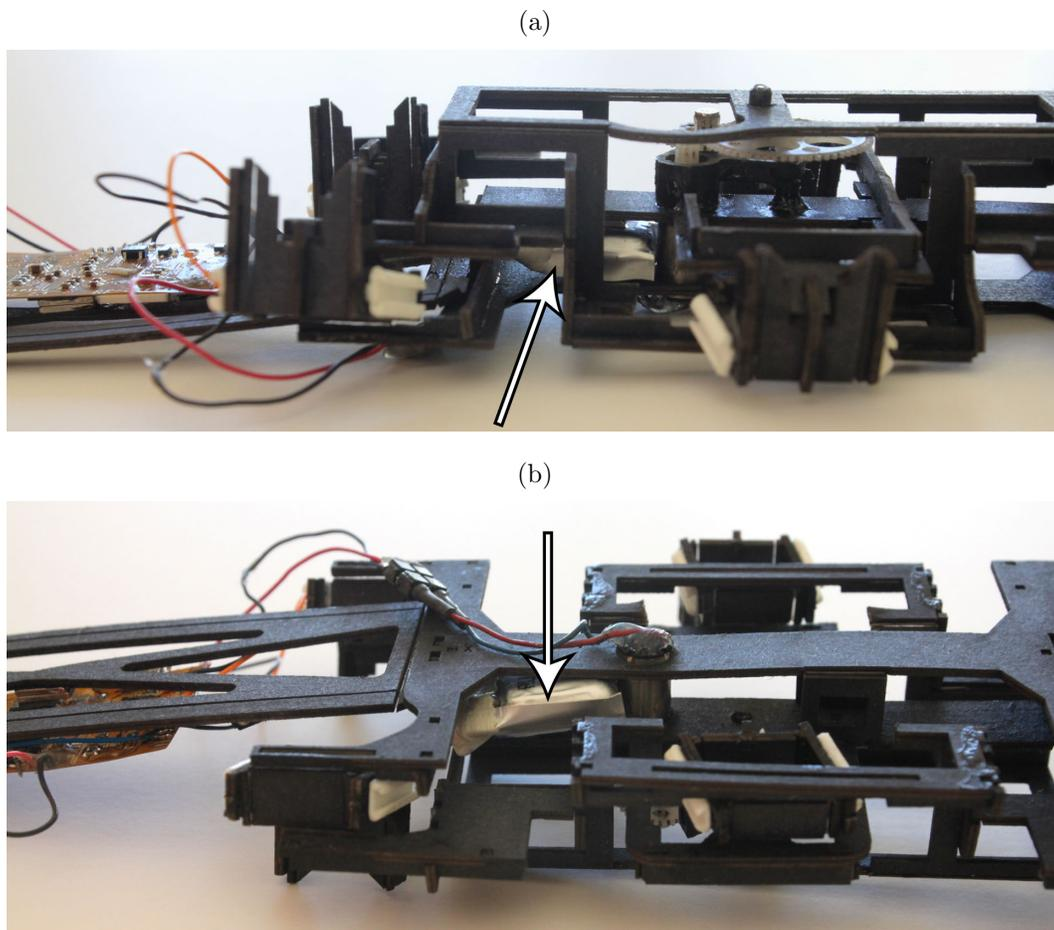
Figure 3.6: Battery placement in CLASH. There is space along the spine of CLASH to house a 60mAh lithium polymer battery to power the system. The battery placement is low and toward the rear of the system to promote a lower pitching moment and passive heading stability. (a) looks at the battery from the side of the system. (b) looks at the battery from the bottom of the robot. Arrows highlight the battery in the structure.
