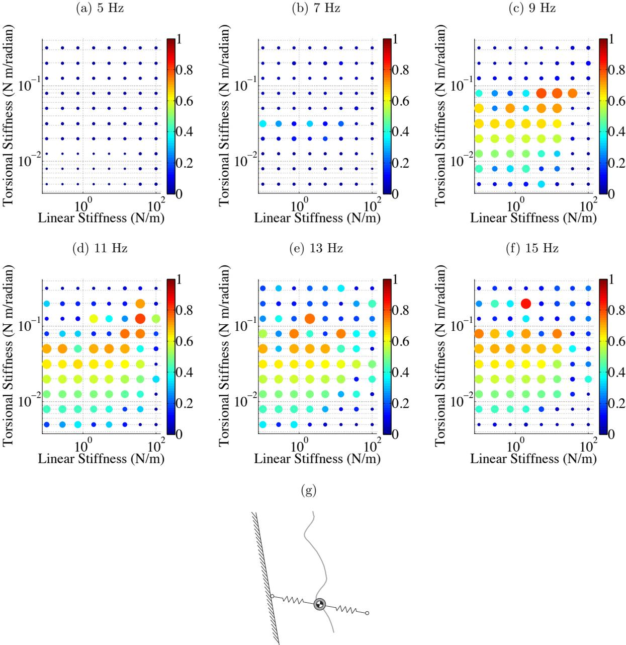
Figure 2.13: Normalized climbing speed of model on 85 degree incline with a gecko-inspired adhesive with properties similar to that used in Chapter 5. Velocities are normalized by the product of the angular velocity of the legs and the leg length. Larger, warmer dots indicate a faster normalized average climbing velocity.
