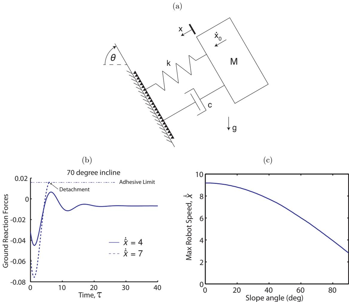
Figure 5.14: (a) Model used showing robot mass,  $m$ , and leg stiffness and damping,  $k$  and  $c$ , at the instant a tripod contacts the ground. (b) Non-dimensionalized impact forces upon touchdown for two different running speeds, with one resulting in loss of contact. (c) Given a certain maximum adhesive force, the climbing velocity,  $\hat{x}$ , must decrease as slope increases to maintain contact with the wall.
