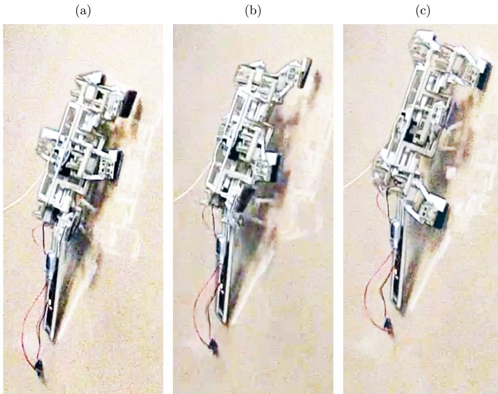
Figure 5.13: Contrast-enhanced frames from high-speed video of CLASH climbing a 70 degree incline at  $10 \text{ cm second}^{-1}$  showing (a) one leg tripod touching the ground, (b) an aerial phase, and (c) the second leg tripod touching down.
