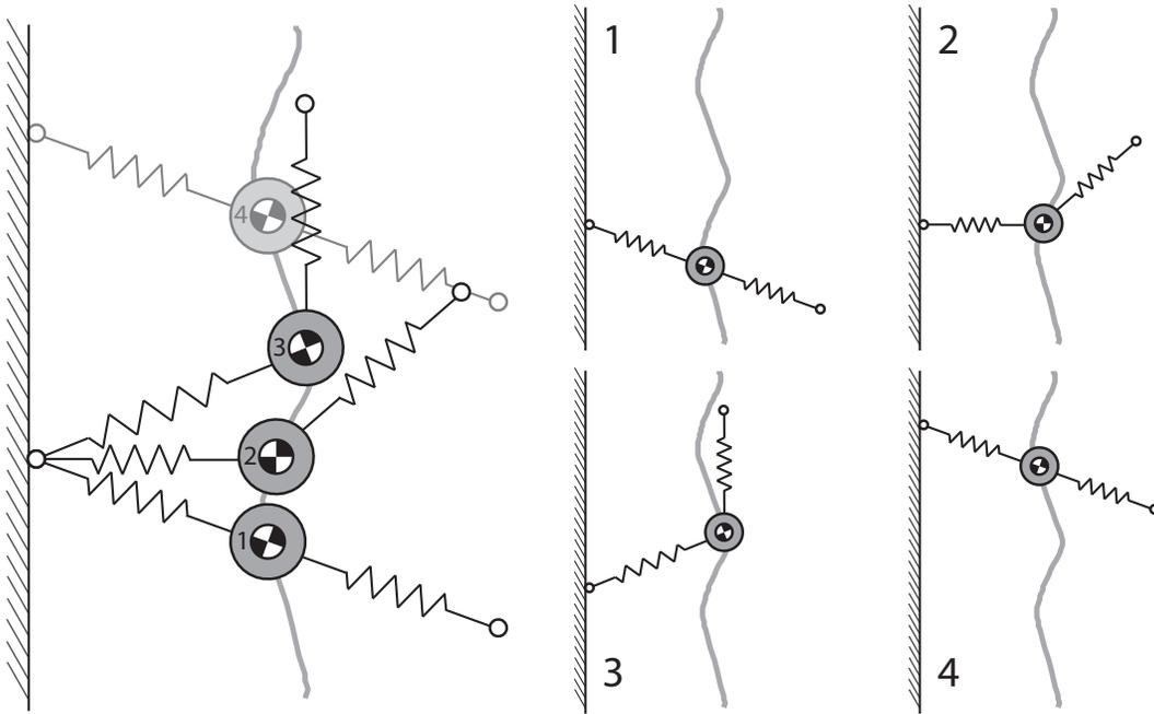
Figure 2.5: A stride of the SLAP model climbing a vertical surface ( $\gamma = 0$ ). (1) The system at touchdown. (2) The system at mid-stance. The unloaded foot continues to follow the prescribed foot trajectory while the foot in stance deflects under load. (3) The system at liftoff. The loaded foot has continued to deflect during stance. (4) The system at the next touchdown. The system is in an aerial phase between (3) and (4).
