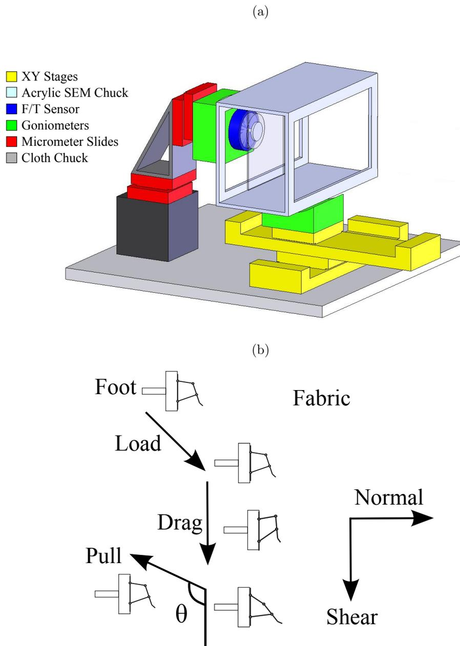
Figure 4.5: (a) The force-displacement apparatus used to test the different foot designs. Feet were mounted on a force sensor and simulated steps were performed on a cloth substrate under displacement control. (b) The simulated step taken by the foot showing the varying pull-off angles that correspond to different running speeds.
