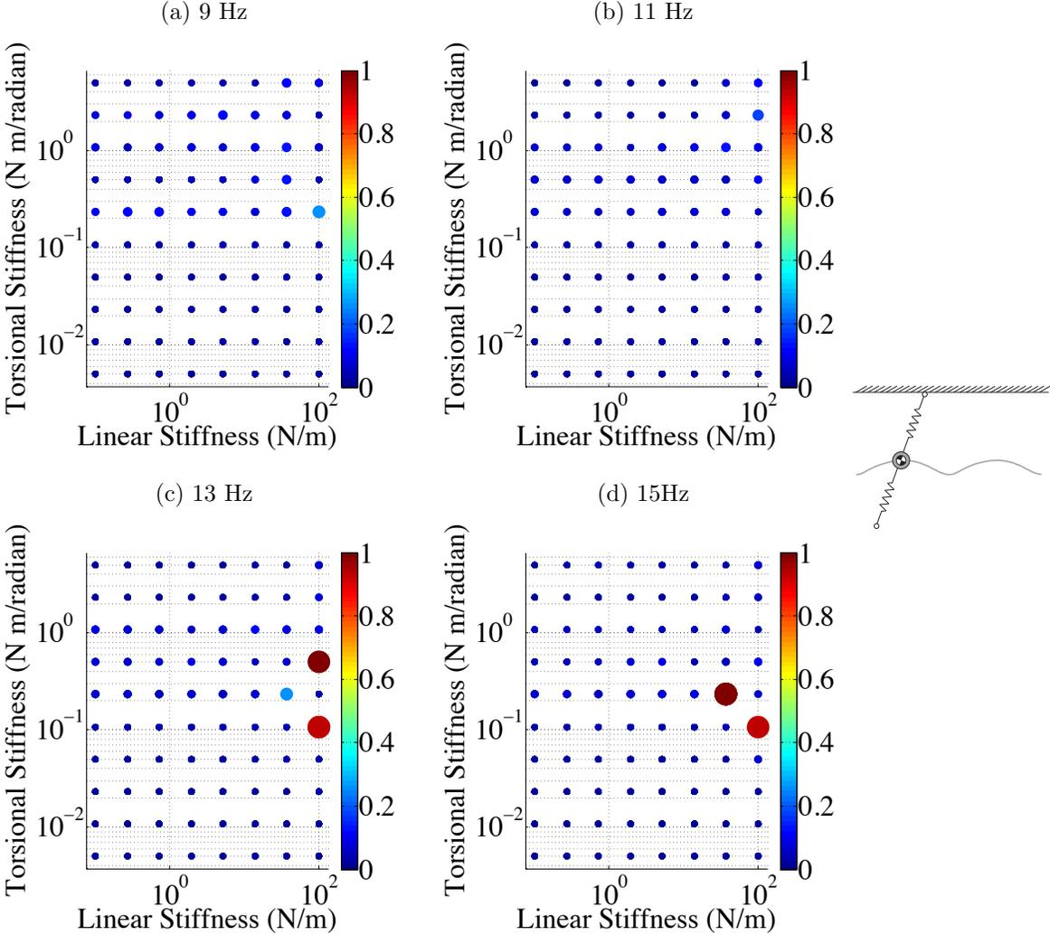
Figure 2.21: Normalized climbing speed of model on an inverted with a controllable adhesive with original parameter set for  $\theta_{release}$ . Velocities are normalized by the product of the angular velocity of the legs and the leg length. Larger, warmer dots indicate a faster normalized average running velocity.
