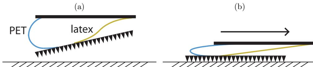
Figure 5.8: Side view of the CLASH foot. (a) The polyethylene terephthalate polymer loop offers a compliant constraint that keeps the rigidly-backed adhesive attached to the RCM ankle but complies in the normal and pitch directions. (b) When loaded, this polymer loop shears with high compliance, allowing the latex tendon to bear most of the load during stance.
