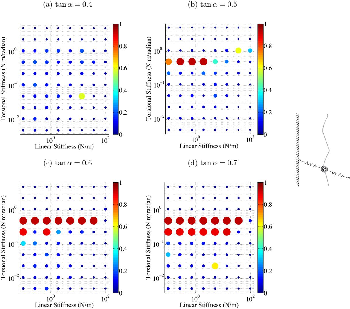
Figure 2.12: A comparison of the performance of the SLAP model on a vertical surface as the shear-to-normal ratio defined by  $\tan \alpha$  is increased for  $\dot{\theta}$ . Velocities are normalized by the product of the angular velocity of the legs and the leg length. Larger, warmer dots indicate a faster normalized average climbing velocity.
