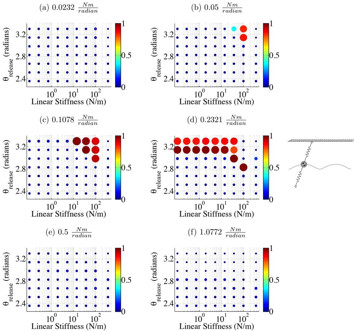
Figure 2.23: Normalized running speed of model on an inverted surface with the clock-based controllable adhesive vs torsional stiffness, linear stiffness, and  $\theta_{release}$ . Velocities are normalized by the product of the angular velocity of the legs and the leg length. Larger, warmer dots indicate a faster normalized average running velocity.
