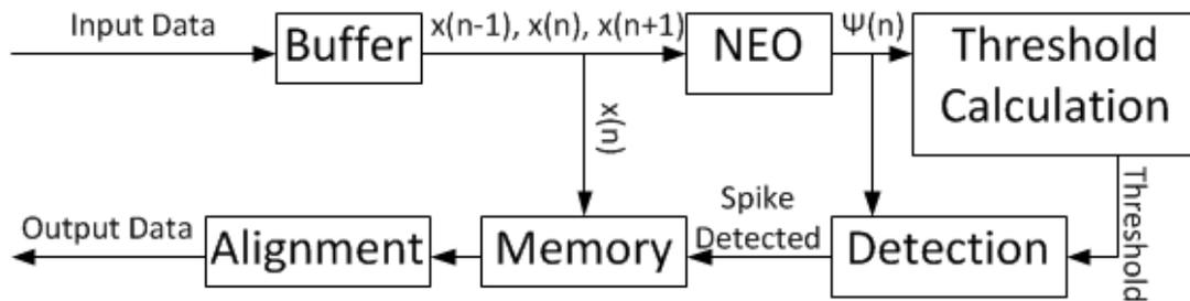
Figure 2. Spike Sorting Block Diagram (Quoted from [5])
