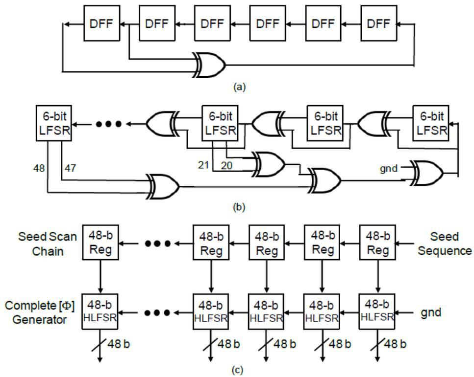
Figure 6. Hybrid Linear Feedback Shift Register Architecture (**Quoted from [1]**)
