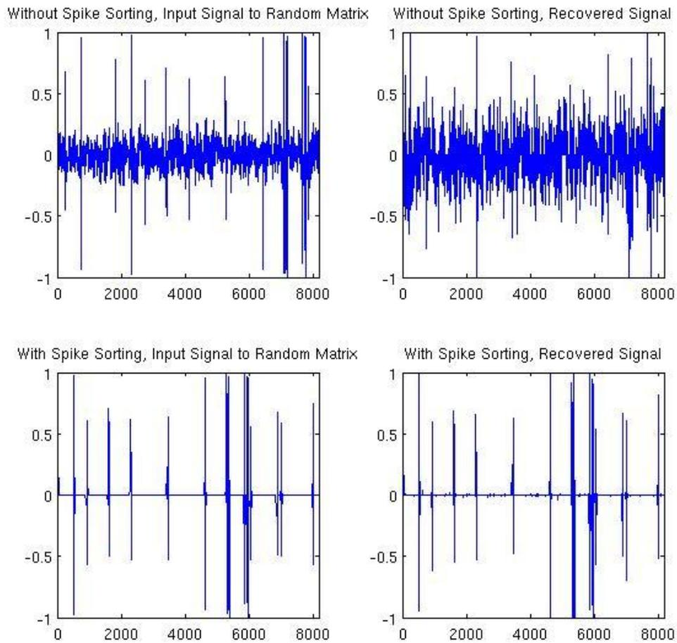
Figure 4. (a) Input signal to random matrix without spike sorting block (b) Recovered signal without spike sorting block (c) Input signal to random matrix with spike sorting block (d) Recovered signal with spike sorting block
