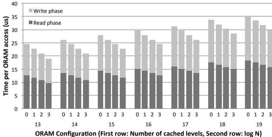
**Figure 7.1:** Average time per ORAM access for different ORAM configurations. The numbers were gathered on the real hardware, performing 1M accesses per experiment with block size 4KB. The 18 and 19 level design points are split across 3 FPGAs.
