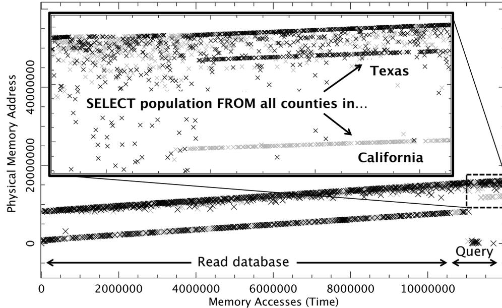
**Figure 2.2:** Visible information leakage in memory address traces from SQLite, running on a RISC-V processor model with caches. Two queries running on the same SQLite database yield clearly discernible memory accesses.
