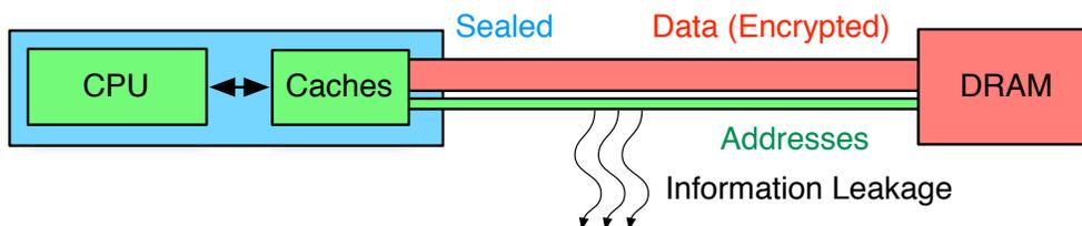
**Figure 2.1:** The basic attack model - we exploit the indicated information leakage. Red indicates encrypted data while green indicates plain-text. An attacker has physical access to every part of the system except the sealed part indicated in blue.
