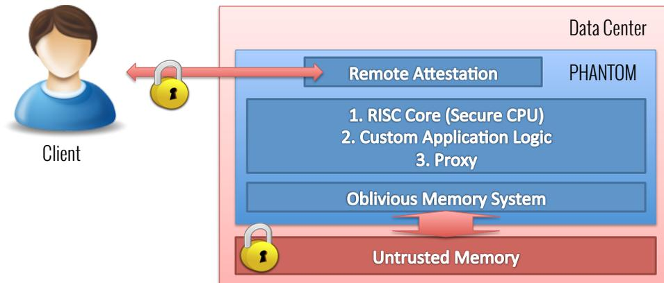
**Figure 4.1:** The different possible usage scenarios for PHANTOM. The ORAM controller can either be used with a Secure CPU, a custom domain-specific accelerator or forward requests from a remote client.
