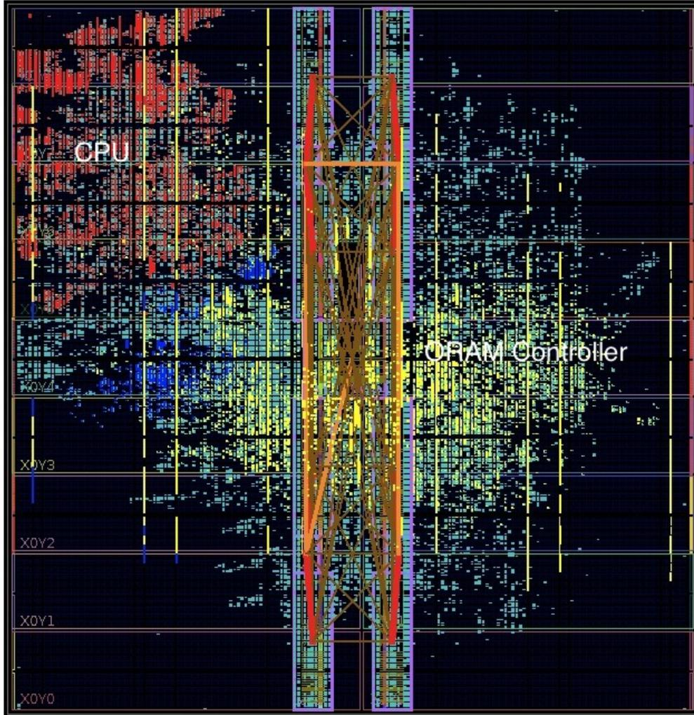
**Figure 7.4:** Synthesized design on a Virtex-6 LX760 FPGA.
