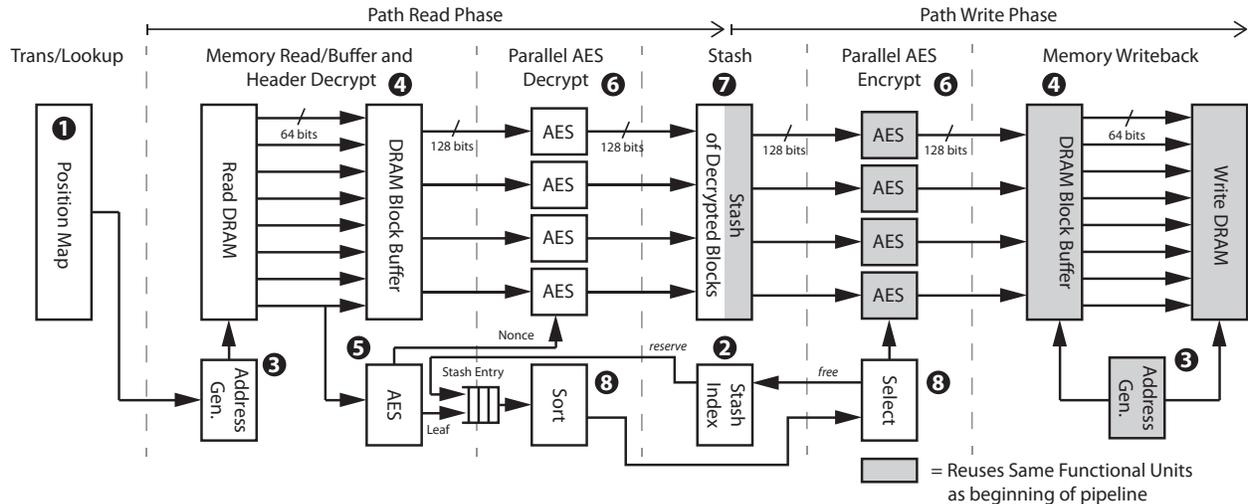
**Figure 5.2:** The data path in PHANTOM’s ORAM controller: Data is read, decrypted and written to the stash. It is then read from the stash, encrypted and written back to memory, using the same functional units.
