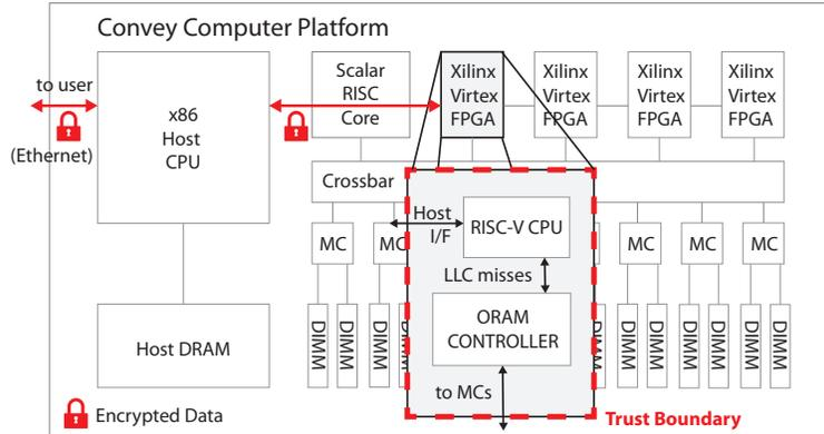
**Figure 4.4:** High-level System Design. PHANTOM comprises a CPU, non-volatile memory, and an ORAM controller implemented on a single FPGA. All *digital* signals outside the PHANTOM chip are assumed to be visible to an adversary.
