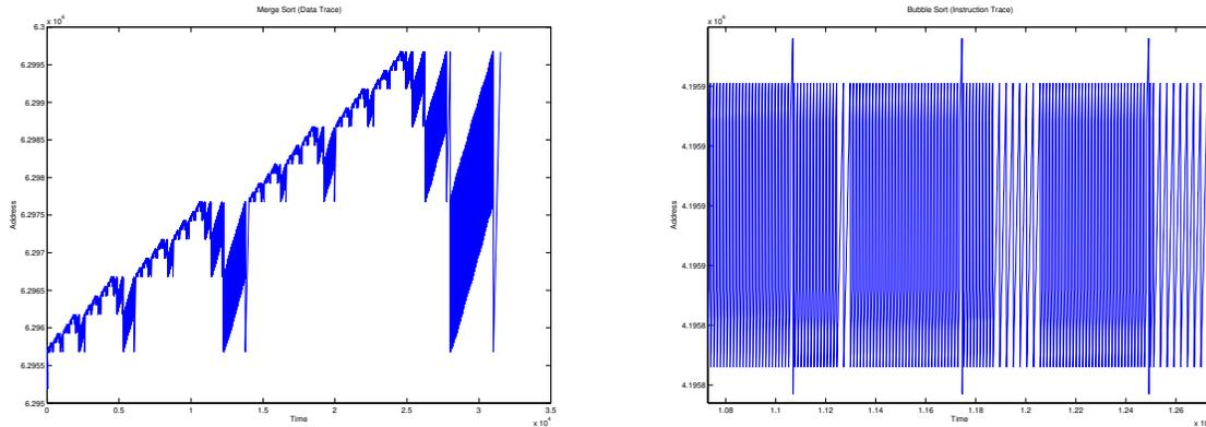
**Figure 2.3:** An example of a data trace and an instruction trace. The data trace stems from an execution of the merge sort algorithm, the instruction trace from a bubble sort implementation. In both cases, the trace indicates which algorithm is being executed.
