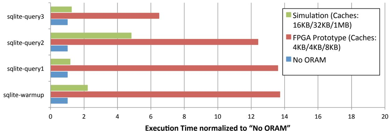
**Figure 7.5:** Performance numbers on our real FPGA hardware and in simulation. All numbers are for a 1GB ORAM and are normalized to the same application running on the real hardware with the RISC-V processor directly connected to the Convey memory system.
