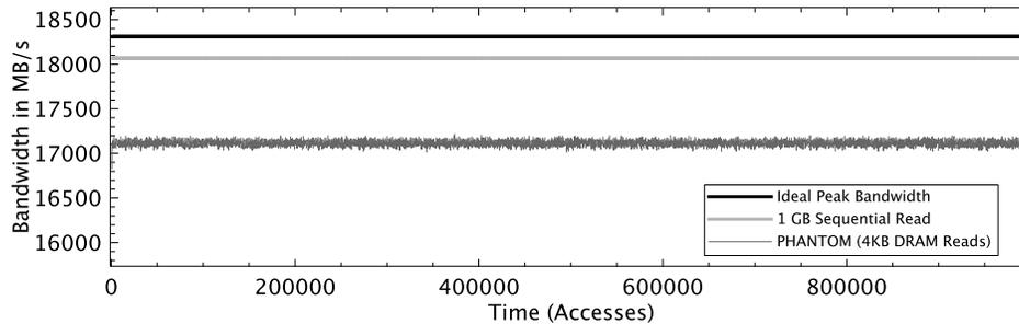
**Figure 7.2:** DRAM bandwidth utilization over time.
