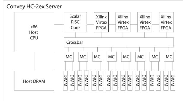
**Figure 4.3:** The Convey HC-2ex Heterogeneous Computing Platform
