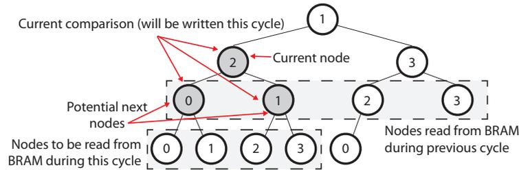
**Figure 5.6:** Min-Heap implementation using the FPGA’s BRAMs. The numbers represent the BRAM each node is stored in. The four second-degree children of each node are put into four separate BRAMs, so that they can be prefetched in parallel.
