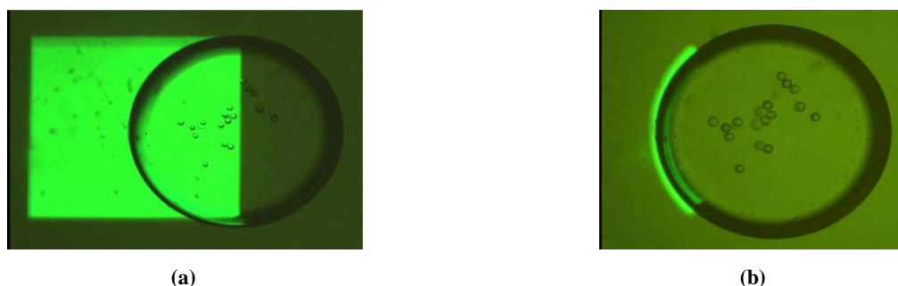
Fig. 4.10 (a) Square-shaped light pattern projected on a droplet. Hydrogel microspheres are contained within the droplet. Temperature increase of 5.3^\circ\text{C} is observed. The scale bar is 1mm; and (b) quarter-ring-shaped light pattern projected on a droplet. Hydrogel microspheres are contained within the droplet. Temperature increase of 0.35^\circ\text{C} is observed. The scale bar is 1mm.
