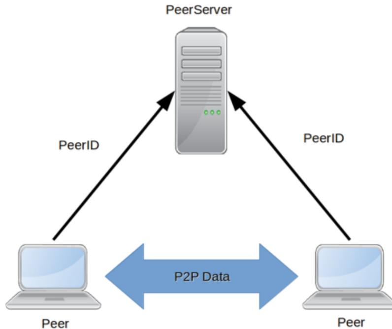
Figure 3: The PeerServer only brokers a connection between the users. Actual data exchange is entirely peer-to-peer.
