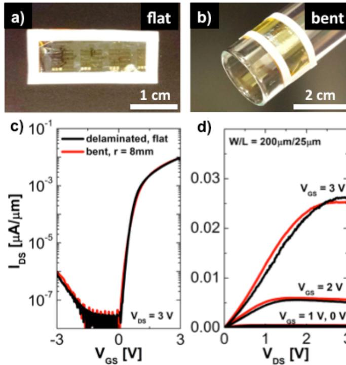
**Fig. 4: Flexible TFT Bending Tests** Images of the substrate while (a) flat and (b) bent around a test tube with  $r = 8$  mm. (c)  $I_{DS}$ - $V_{GS}$  and (d)  $I_{DS}$ - $V_{DS}$  curves for a device on free-standing polyimide with  $W/L = 200 \mu\text{m}/25 \mu\text{m}$  while flat (black) and bent at  $r = 8$  mm (red).
