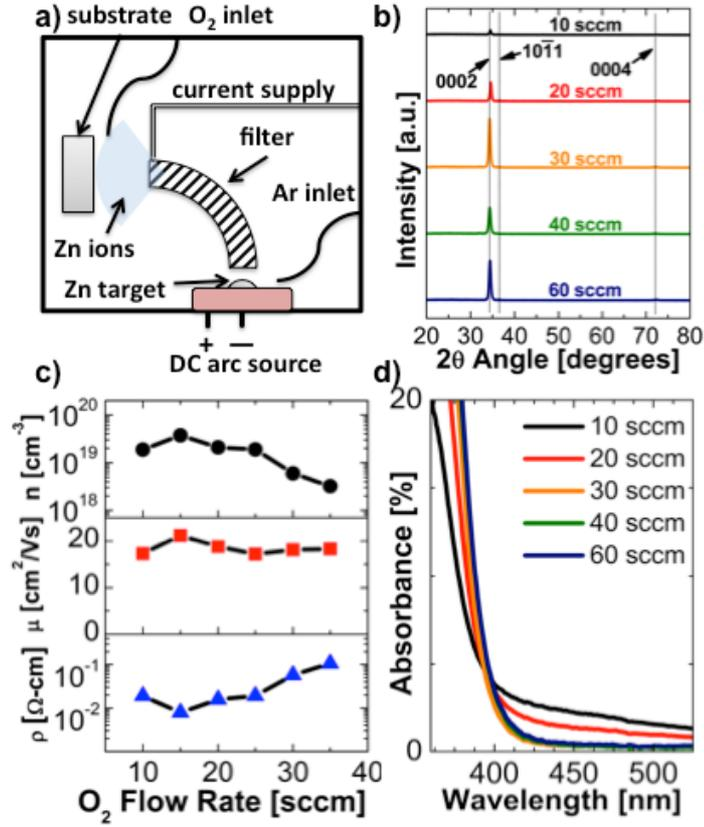
**Fig. 2: Cathodic Arc Setup and ZnO Film Characterization** (a) Schematic of cathodic arc deposition chamber. The permanent magnet is denoted in red. (b) XRD pattern for ZnO film and varying O<sub>2</sub> flow rates. (c) Electron concentration ( $n$ ), Hall mobility ( $\mu$ ), and resistivity ( $\rho$ ) as a function of O<sub>2</sub> flow rate. (d) Dependence of optical absorption with O<sub>2</sub> flow rate.
