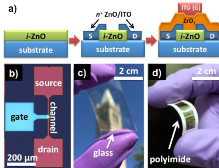
**Fig. 1: Process Flow and Images of Devices** (a) Process schematics of ZnO TFT
