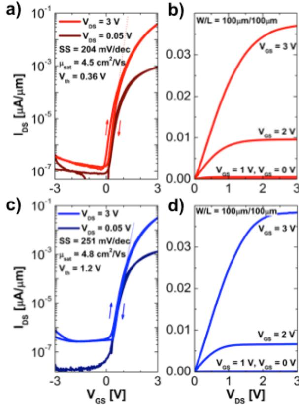
**Fig. 3: TFT Performance**  $I_{DS}$ - $V_{GS}$  and  $I_{DS}$ - $V_{DS}$  curves for  $W/L = 100\ \mu\text{m}/100\ \mu\text{m}$  device on (a, b) alkali-free glass and (c, d) polyimide. The arrows on the transfer curves indicate the direction of the double sweep measurement.
