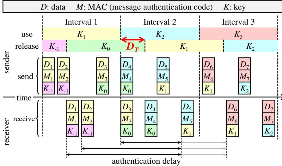
Figure 5.6: Given the worst-case transmission delay  $D_T$ , an approach to reduce the authentication delay, where the key-using and key-releasing intervals are not aligned.
