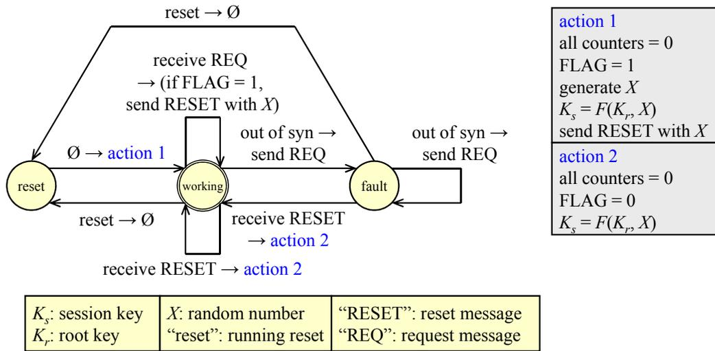
Figure 3.4: The finite state machine of a node in the dynamic network-wide reset.
