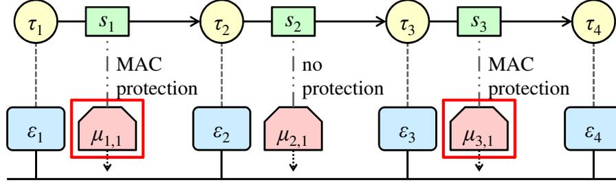
Figure 4.4: Security should be modeled by a path-based security constraint considering possible attacks triggering an actuator. Protecting  $\mu_{1,1}$  and  $\mu_{3,1}$  is not enough because an attacker can still attack  $\mu_{2,1}$  and result in triggering  $\tau_4$  on  $\epsilon_4$ .
