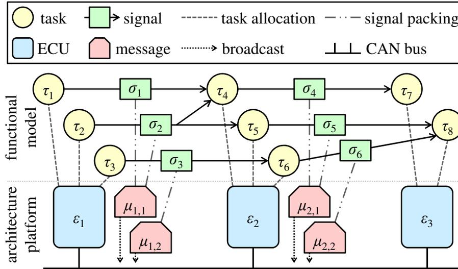
Figure 4.1: The system model of a CAN-based system.
