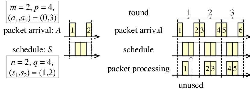
Figure 5.7: An example for synchronous messages with tree rounds. The second packet (#2, #4, or #6) of each round is an unscheduled packet after its corresponding round, and the second time slot of the first round is an unused time slot. The second round and the third round have the same packet processing pattern.
