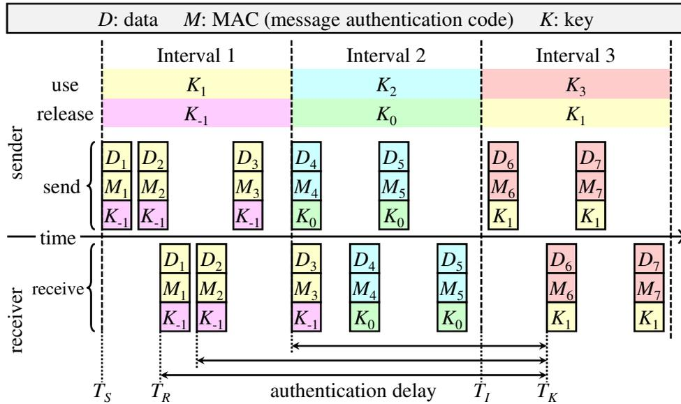
Figure 5.2: The time-delayed release of keys.  $T_S$ ,  $T_R$ , and  $T_K$  are the sending time, the receiving time, and the key-receiving time of the packet  $(D_1, M_1, K_{-1})$ , respectively.  $T_I$  is the starting time of Interval 3.
