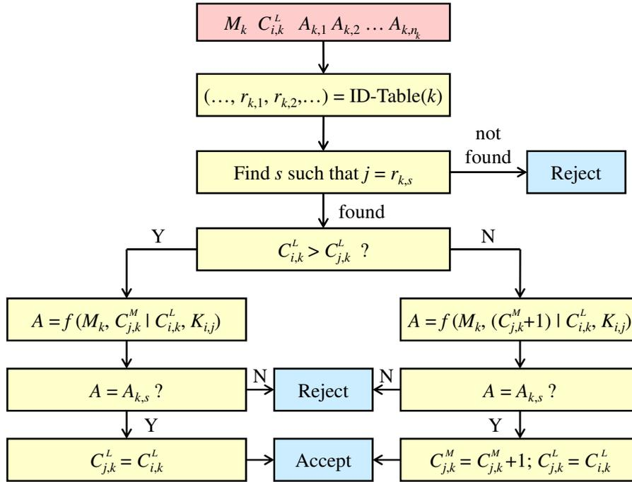
Figure 3.3: The steps performed by a receiver  $N_j$  of a message  $M_k$  sent by a sender  $N_i$ .
