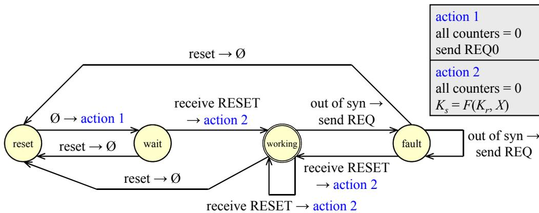
Figure 3.6: The finite state machine of a non-master node in the static network-wide reset.
