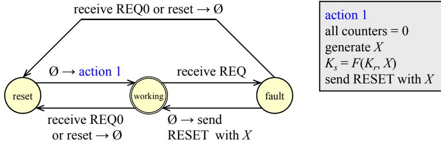
Figure 3.5: The finite state machine of a master node in the static network-wide reset.
