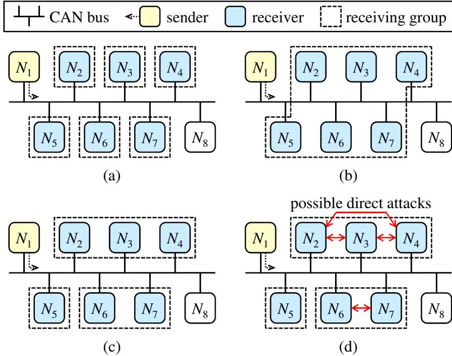
Figure 4.2: Given a message sent by node  $N_1$  and received by  $N_j$  ( $2 \leq j \leq 7$ ), (a) the pair-wise key distribution, where 6 MACs are required to be sent with the message, and there is no possible direct attack; (b) the one-key-for-all key distribution, where only 1 MAC is required, but there are possible direct attacks between any pair of receivers; (c) another key distribution, where 3 MACs are required, and (d) there are some possible direct attacks.
