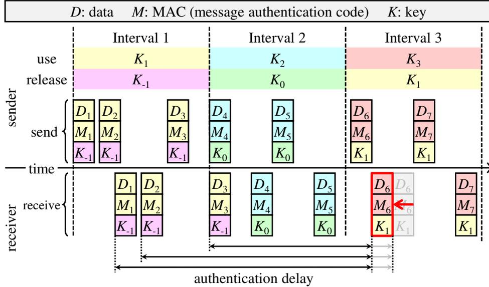
Figure 5.4: An approach to reduce the authentication delay.
