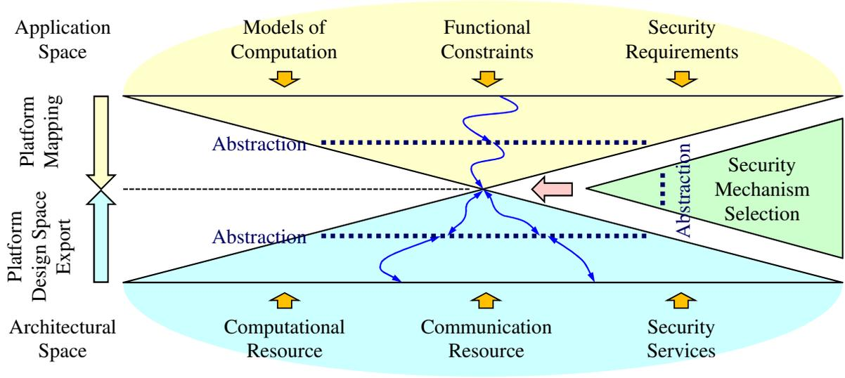
Figure 2.1: The security-aware mapping. A functional model, an architectural platform, and a security mechanism are initially captured separately as abstractions and brought together through a mapping process so that all constraints are satisfied and the design objective is optimized.
