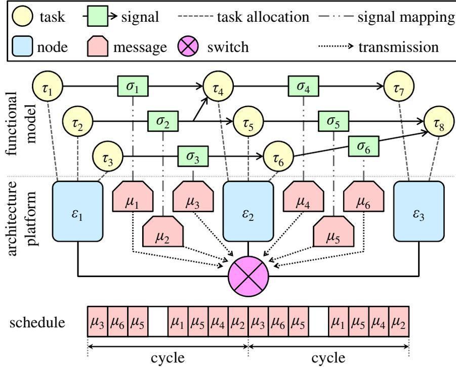
Figure 5.1: The system model of a TDMA-based system.
