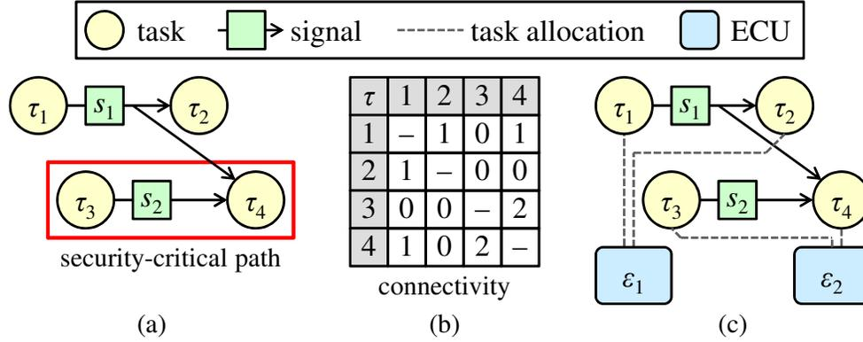
Figure 4.5: (a) Given the task graph, (b) compute the connectivity with both weights being 1 and (c) allocate the tasks to the ECUs.
