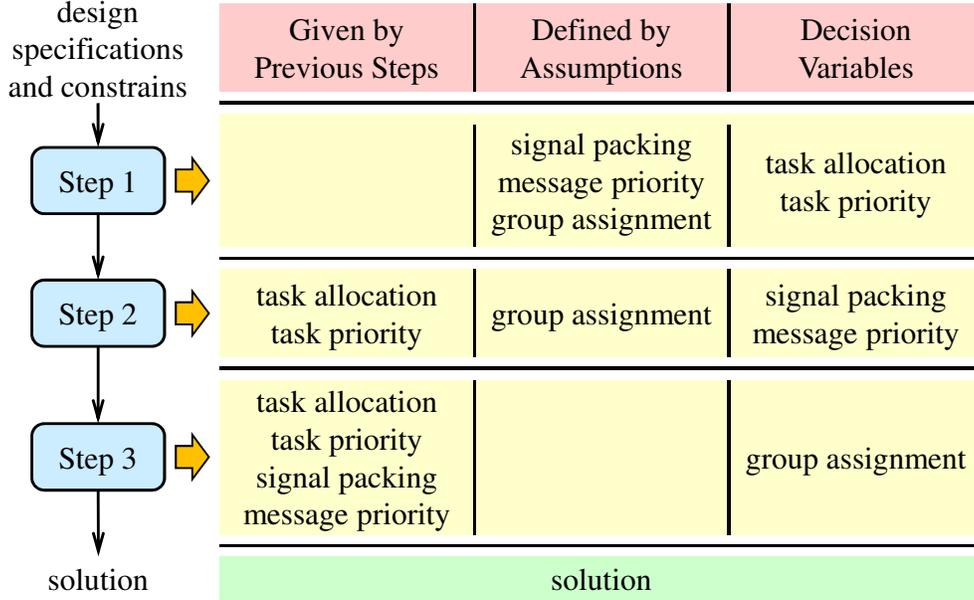
Figure 4.3: The flow of three-step MILP-based algorithm, where “group assignment” means “receiving group assignment.” The task allocation and the task priority are solved in Step 1; the signal packing and the message priority are solved in Step 2; the receiving group assignment is solved in Step 3.
