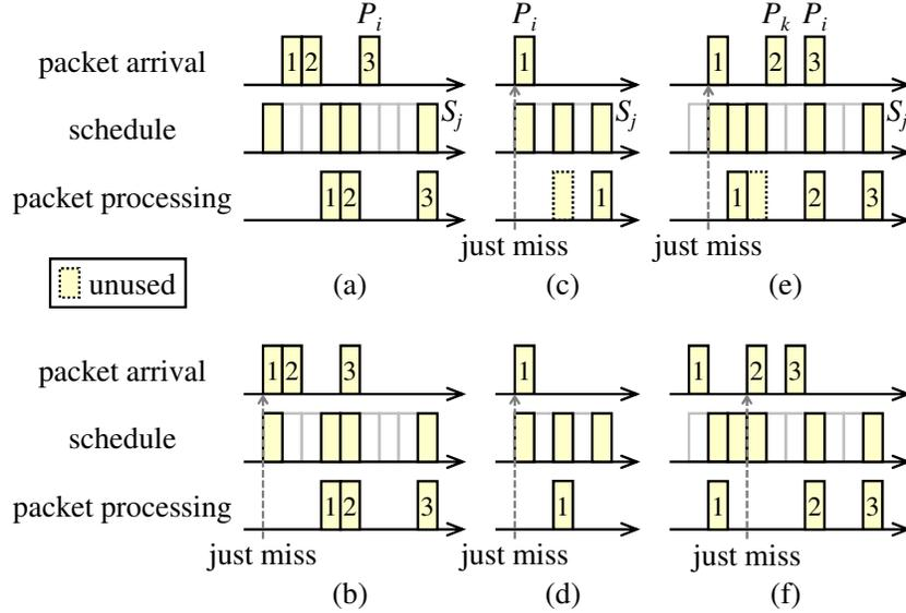
Figure 5.8: For asynchronous messages, if the worst-case transmission delay happens when packet  $P_i$  is assigned to time slot  $S_j$ , then (a–b) one of  $P_i$  itself and the packets arriving before  $P_i$  must just miss a time slot, and (c–f) there must be no unused time slot between the arriving time of the packet just missing a time slot and the starting time of  $S_j$ .
