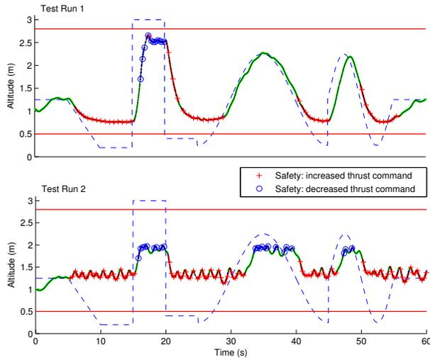
Figure 3: Altitude trajectory of the quadrotor while learning the disturbance and tracking a reference. Run 1 is performed with a conservative disturbance model, while Run 2 is performed with an inferred model that fails to predict the true disturbance in certain regions of the state space.
