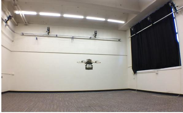
Figure 2: A STARMAC quadrotor during the flight test.
