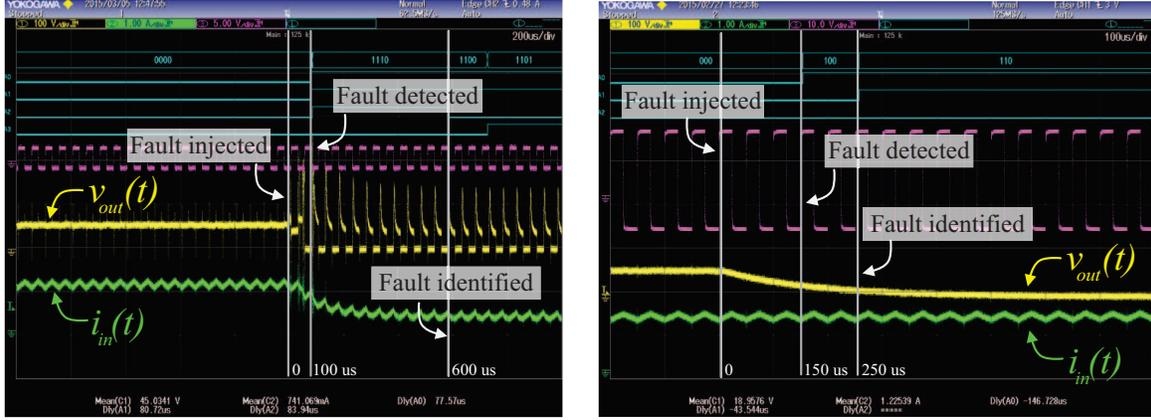
(a) Fault detection and identification for a component fault in  $C$ . (b) Fault detection and identification for a sensor fault in  $v_{out}$ .
