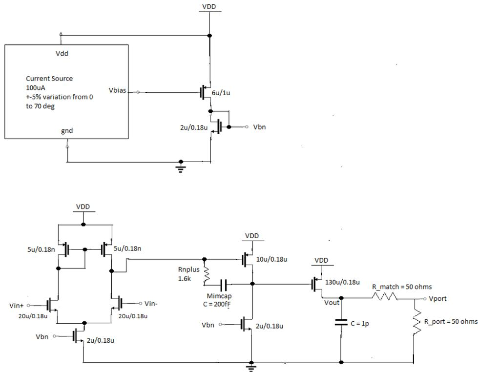
**Figure 8: Final Schematic of Wideband Op Amp using NMOS input pair.**
