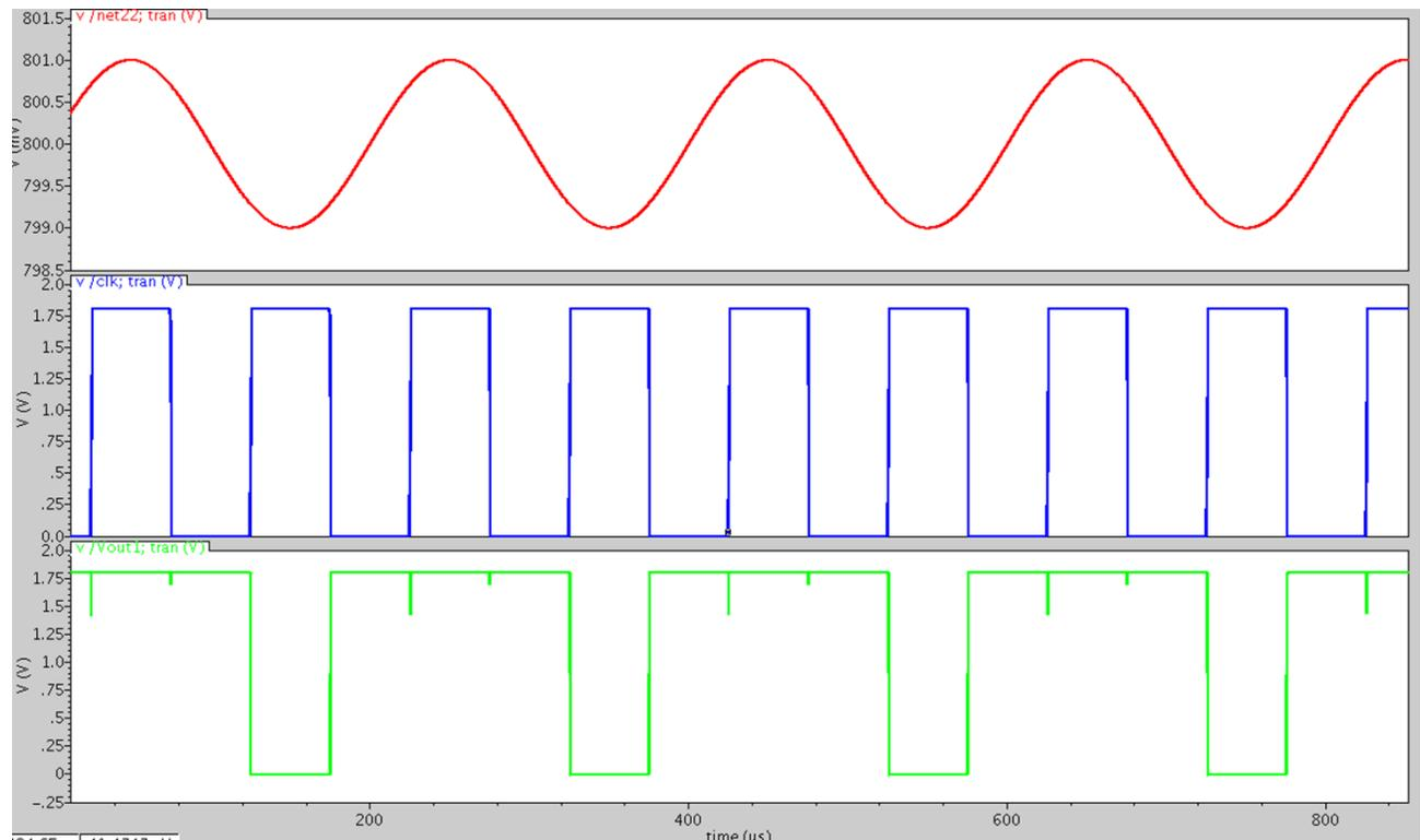
**Figure 15. Comparator Functionality**
