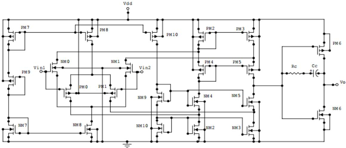
**Figure 7: Transistor-level schematic of a Complementary Differential Pair with a cascoded NMOS load followed by a push-pull inverter output stage.**
