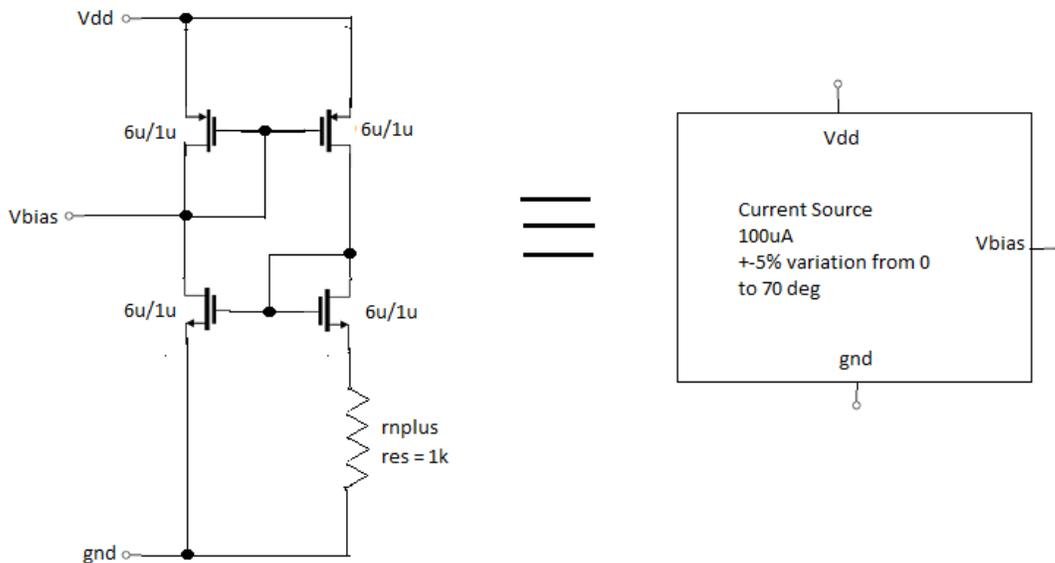
**Figure 11: Cadence Virtuoso schematics of biasing circuitry for the Comp-Casc op-amp.**
