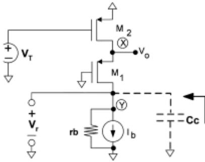
**Figure 4: Flipped Voltage Follower (FVF) Configuration**
