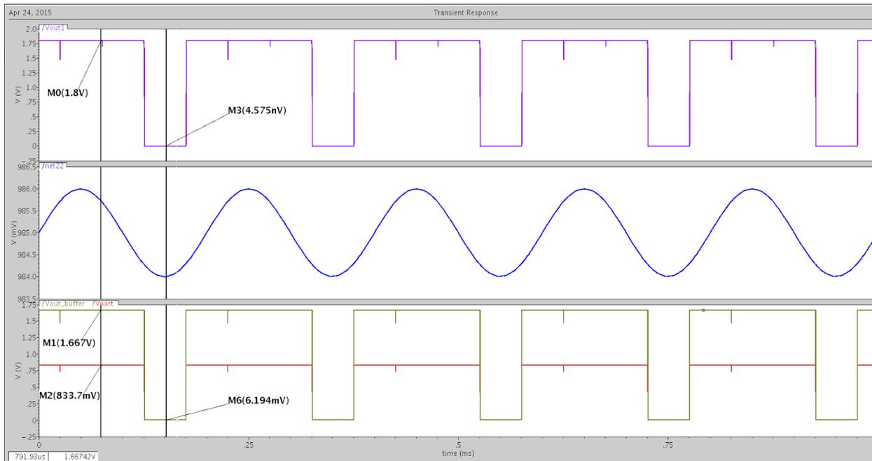
**Figure 29: Test Setup (part a) and Transient Response (part b) for comparator and rail-to-rail buffer. Blue trace is the test signal (output of envelope detector), purple trace shows output of the comparator, green trace shows the output of the voltage buffer, and red signal shows the signal being sent to the load after matching.**
