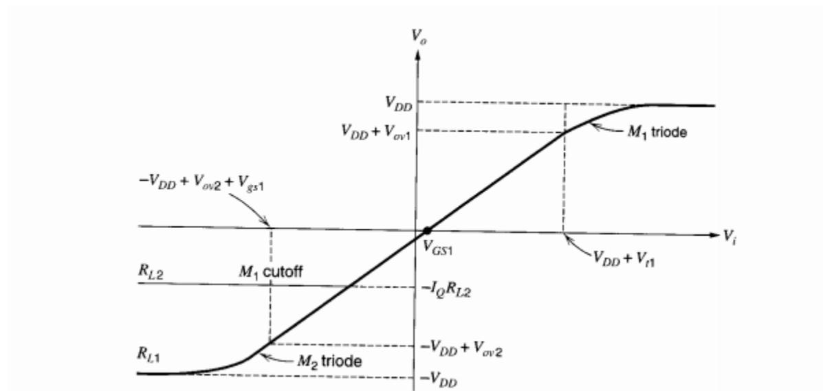
Figure 2: Source Follower Configuration with (a) showing the topology and (b) showing the voltage transfer characteristics from input to output.
