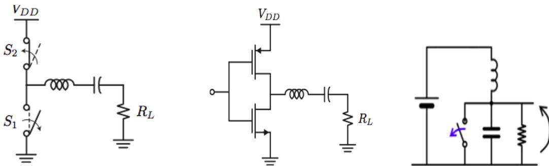
Figure 18. Class D & E Amplifier models [10]
