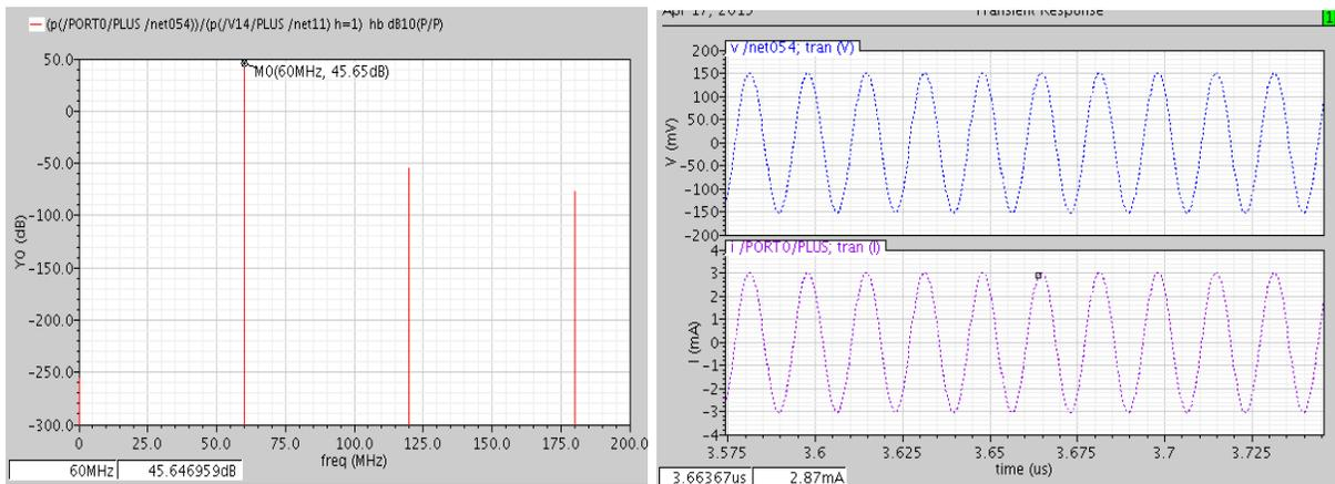
Figure 22: measured power gain & simulated output waveforms
