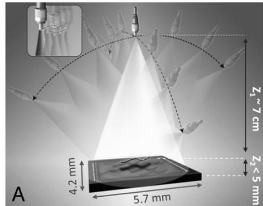
Figure 3: Multiple-axis tomography. The light source (top of image) rotates about the imaging plane in multiple directions for improved quality (Isikman, p. 2).
