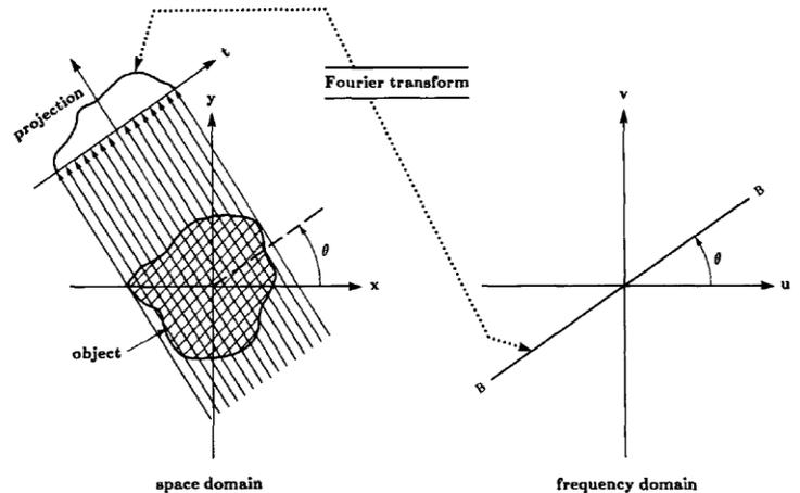
Figure 1: Parallel beam projection calculation (left) and the mapping of its transform to Fourier space (right) (Kak and Slaney, p. 57).
