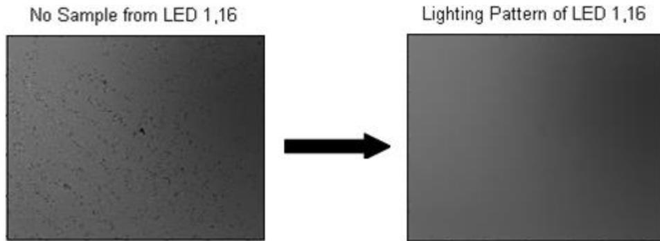
Figure 9: A blank image taken from LED with coordinates (1,16) on the LED grid, and its corresponding illumination pattern obtained after processing with the local thresholding algorithm.
