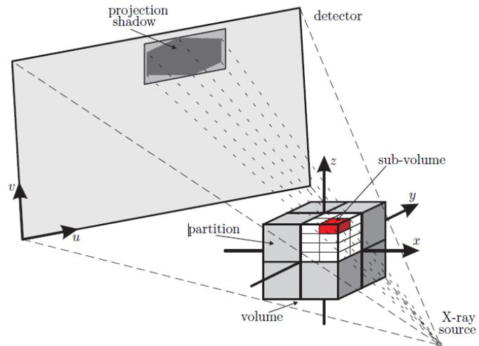
**Figure 2: Cone-beam projection by an X-ray source. The object space is broken down into voxels to be assigned values during the reconstruction (Scherl et al., 2007, p. 3).**
