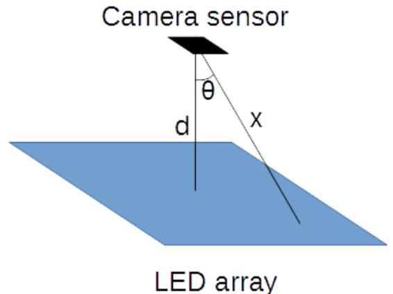
Figure 6: Geometric setup showing path length differences between the camera sensor and different LEDs as related by the central angle  $\theta$ .
