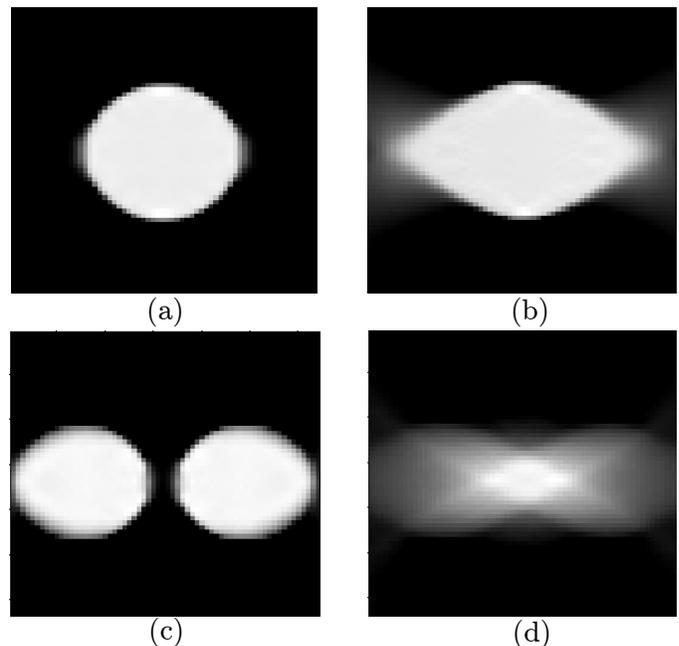
Figure 11: Simulated reconstruction results for central slices of spheres. (a) Forward-facing central slice of single sphere. (b) 90° rotation of image (a). (c) Two spheres with source-detector axis out of the page. (d) Two spheres with horizontal source-detector axis.
