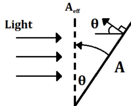
Figure 5: Effective surface area of a CCD with incident light at an angle of  $\theta$ .
