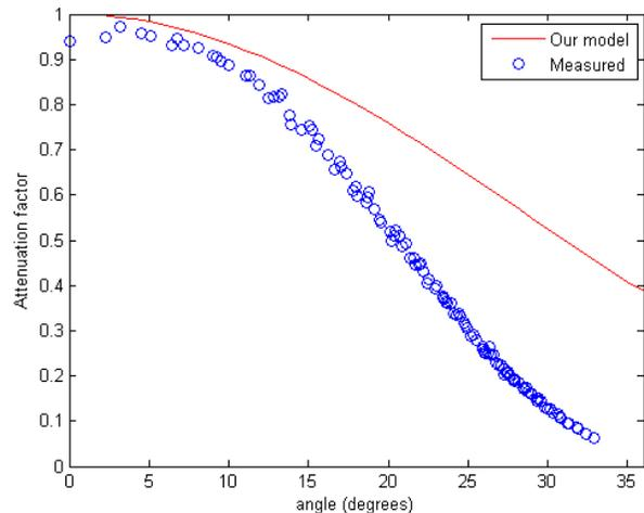
Figure 8: Light falloff vs. angle from center. The measured falloff was calculated by taking the averages of blank images at various illumination angles.
