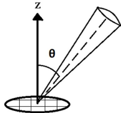
Figure 4: LED array (bottom plane) emitting light in a solid angle at angle  $\theta$  from the perpendicular.
