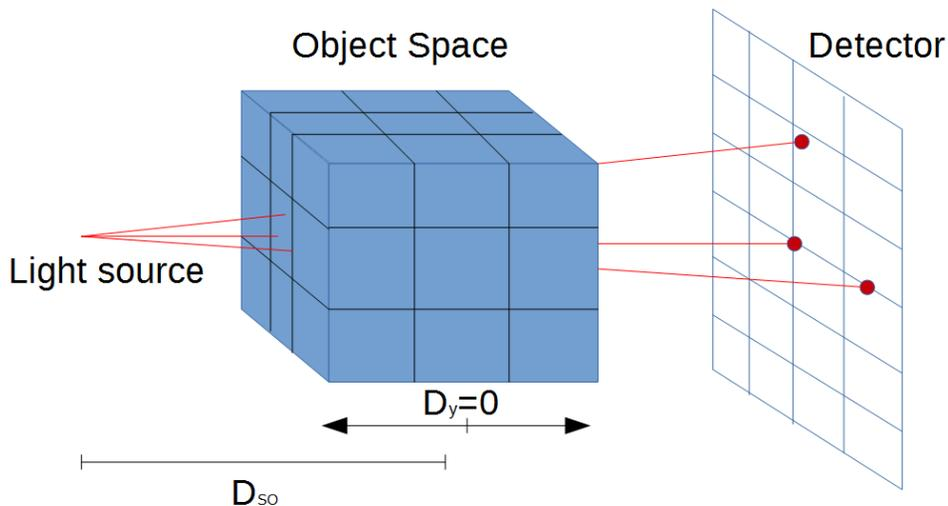
Figure 7: Ray tracing through three example voxels (blue) to find the corresponding points on the detection plane (red dots). The detection plane has a grid of values supplied by the projection data. These values are linearly interpolated in 2D to find the values at the red dots.  $D_{s0}$  is the distance between the source and object center, and  $D_y$  is the distance from the center of the object to a given voxel, which is used in the tracing process.
