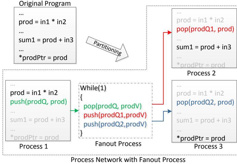
Figure 4.2: Addition of Fanout Process while Partitioning
