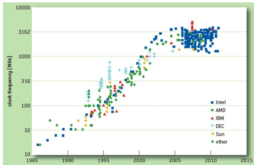
Figure 1.1: Processor Frequency Scaling Over Time [3]
