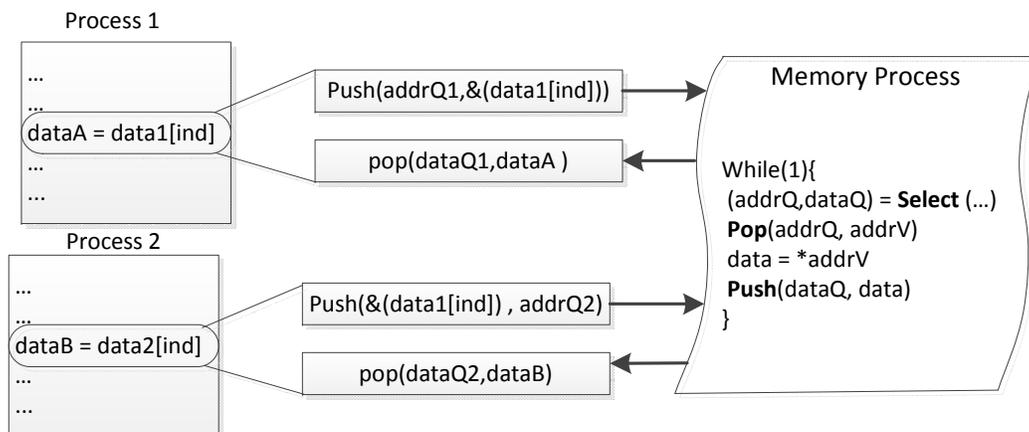
Figure 4.1: Modeling Memory Access as Inter-process Communication
