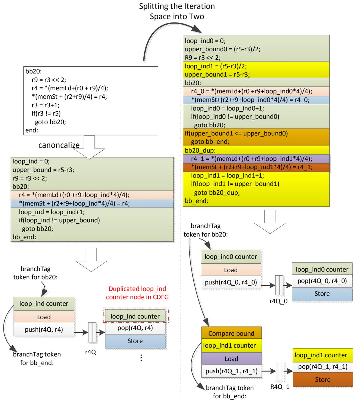
Figure 5.9: Thread-level Parallelization
