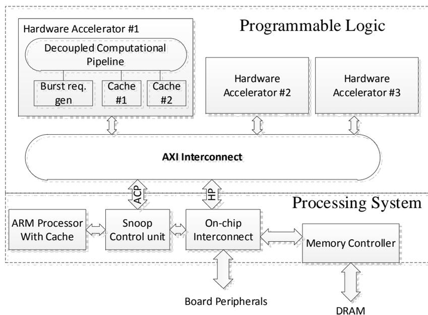
Figure 3.15: Implementation of Computational Pipeline in FPGA SoC
