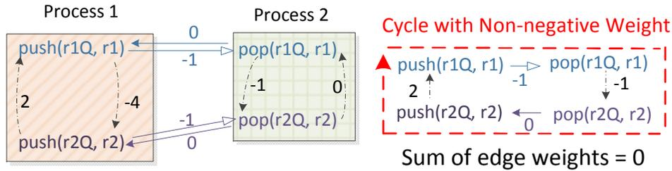
Figure 4.5: Deadlock Detection using Graph with Weighted Edge
