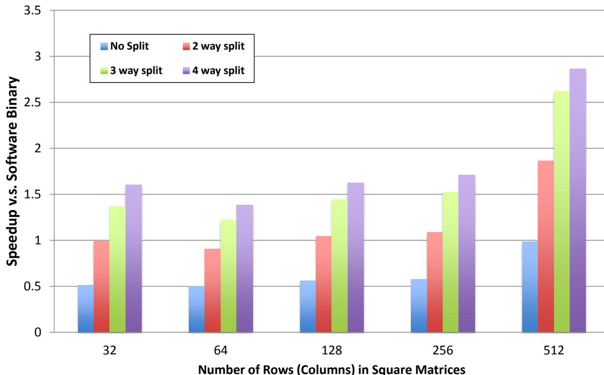
Figure 5.15: Performance Comparison of Decoupled Computational Pipeline and Software Binary for Matrix Multiplication
