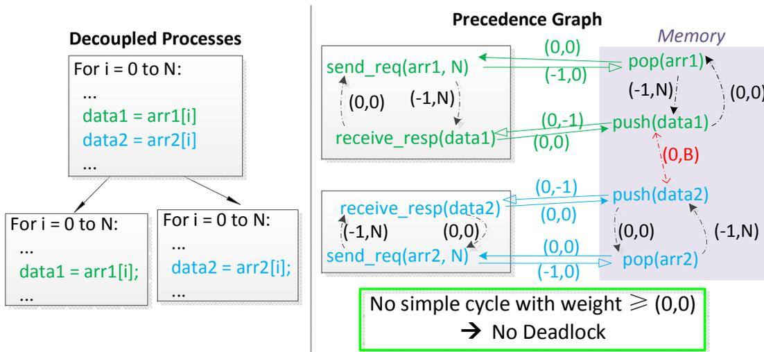
Figure 4.14: Burst Mode Memory Access by Decoupled Processes
