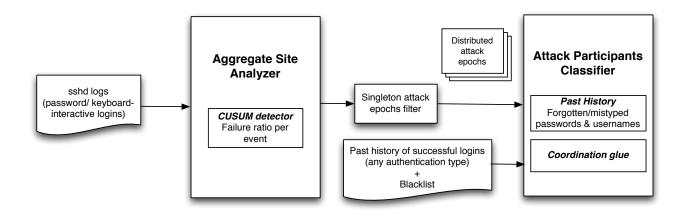
Figure 4.1: System diagram of our distributed SSH brute-forcing detector
