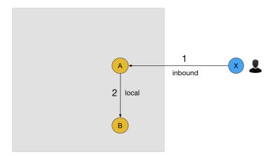
(a) User at an external machine X logs into machine A at the site and steps through it to access machine B.
