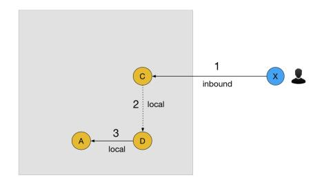
Figure 5.4: Example scenario involving the user stepping through a machine that does not syslog: a user at the external machine X logs into the cluster C at the site and steps through it to access the cluster node D, which does not syslog. She then copies data from D to her machine A.
