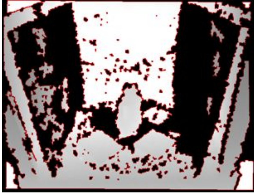
Figure 2.3: Applying depth discontinuity filtering. Pixels marked in red are considered unreliable due to either a discontinuity or neighboring pixels that were not measured by the Carmine depth sensor. Before proceeding, we discard depth measurements associated with the red pixels.
