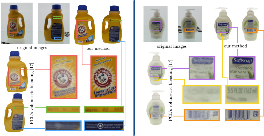
Figure 4.1: Arm & Hammer Detergent (top) and Softsoap Aloe Vera (bottom), reconstructed using our method and PCL’s volumetric blending 80 . The BigBIRD scanning rig (Figure 2.1) captures 600 DSLR RGB images per object 90 ; we show two per object here. Our color models can recover very fine textural details: in the Aloe Vera soap, the “5.5 FL OZ” text is 3 mm tall; the numbers under the barcode are just over 1 mm tall. PCL’s volumetric blending smooths away these details.
