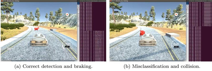
Fig. 8: Unity-Udacity simulator AEBS. The onboard camera sends images to the CNN. When a cow is detected a braking action is triggered until the car comes to a complete stop. Full videos available at <https://www.youtube.com/watch?v=Sa4oLGcHAhY> and <https://www.youtube.com/watch?v=MaRoU50gimE>.
