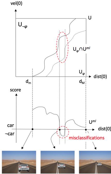
Fig. 2: Compositional falsification scheme on AEBS model. The “score” indicates the confidence level with which the classifier determines whether the image contains a car or not.
