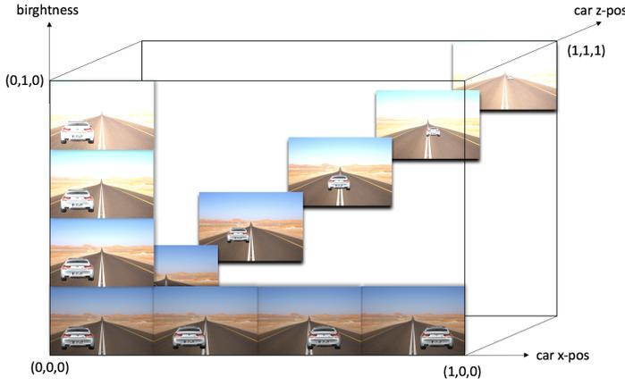
Fig. 3: Feature Space Abstraction. The cube represents the abstract space  $A$  with the three dimensions corresponding to three different image modifications. The displayed road images correspond to concretized elements of the concrete feature space  $\tilde{X}$ .
