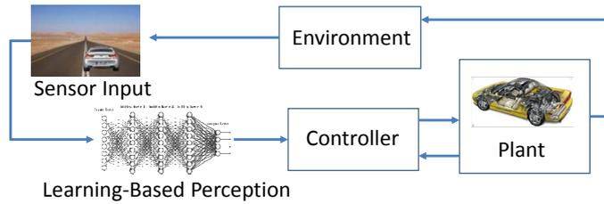
Fig. 1: Automatic Emergency Braking System (AEBS) in closed loop. A machine learning based image classifier is used to perceive objects in the ego vehicle’s frame of view.
