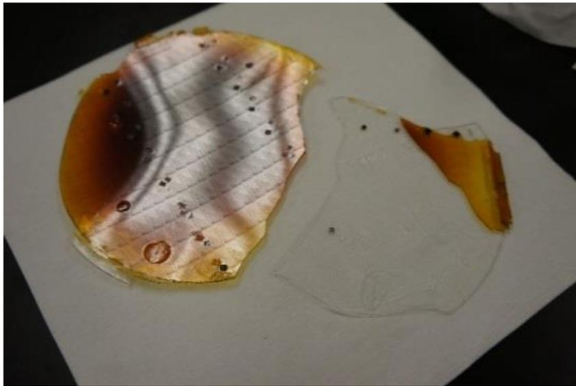
Figure 3-8. Epoxy molding on top of six inch glass carrier wafer that has cracked due to thermal stresses during curing.
