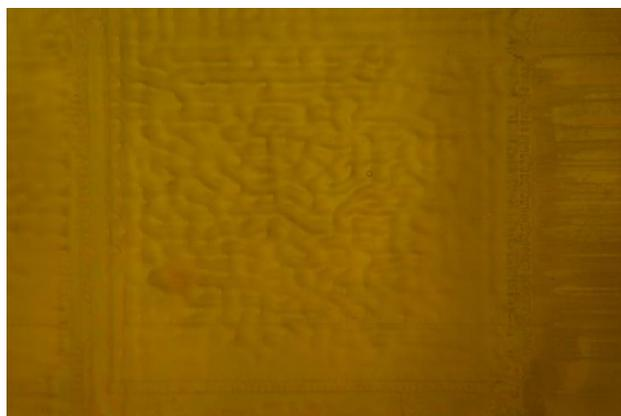
Figure 2-11. Optical micrograph of printing artifacts on plastic (PET) confirming that printing artifacts are independent of paper substrate (7 layers of PVP, 718cP).
