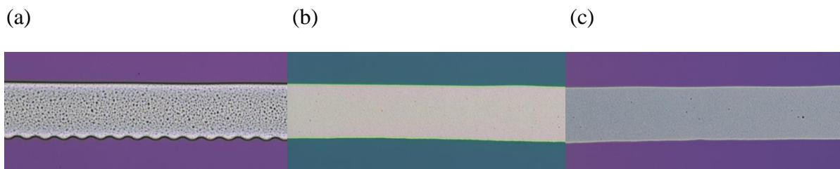
Figure 5-27. ANP gate on top of D320 gate dielectric after sintering. (a) Sintering at 100°C for 30 minutes without ramp resulting in large number of holes in dielectric (black dots). (b) Sintering at 30°C for 15 minutes in vacuum significantly improves the hole density. (c) Further heating at 100°C for 10 minutes after initial drying at 30°C does not result in the creation of holes.
