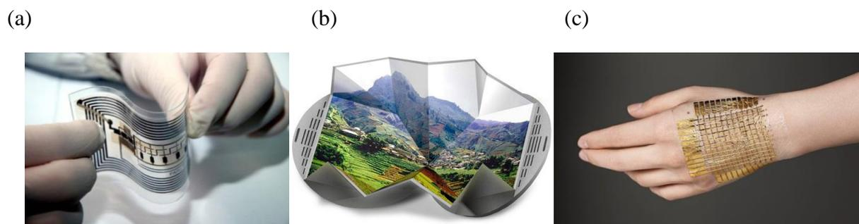
Figure 1-1. Applications that are fundamentally large-area and thus ideally suited to take advantage of the benefits of printed electronics (a) RFID tag with antenna ([www.wired.com](http://www.wired.com)), (b) Flexible display ([www.display-central.com](http://www.display-central.com)), (c) Electronic skin sensor network ([www.hight3ch.com](http://www.hight3ch.com))
