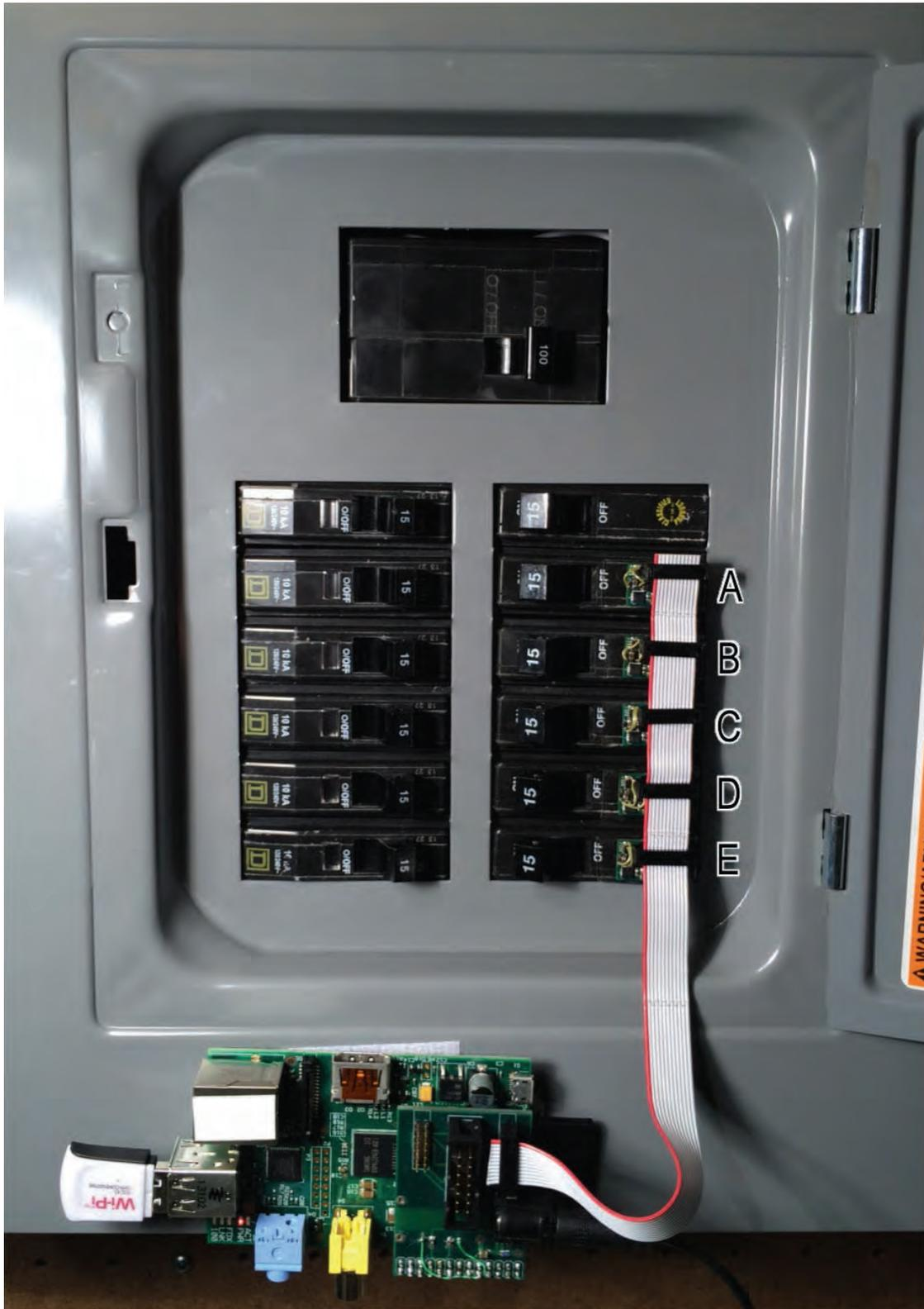
Figure 3.2: PASEM system installation on circuit breaker panel. Five PASEM devices installed with wireless base station at bottom. Circuit breakers labeled for reference.
