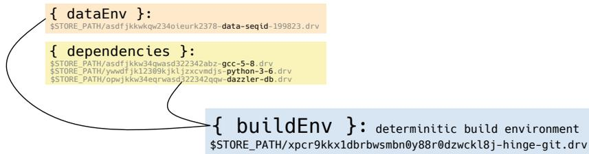
Figure 1: Each package is built in a fully deterministic environment. By computing the cryptographic hash for each derivation, we can guarantee that each invocation of the build leads to the same exact binary.
