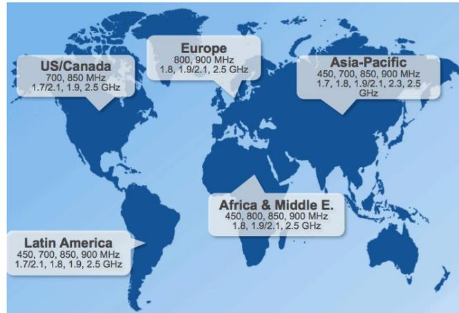
Figure 1.4: LTE global frequency allocations.
