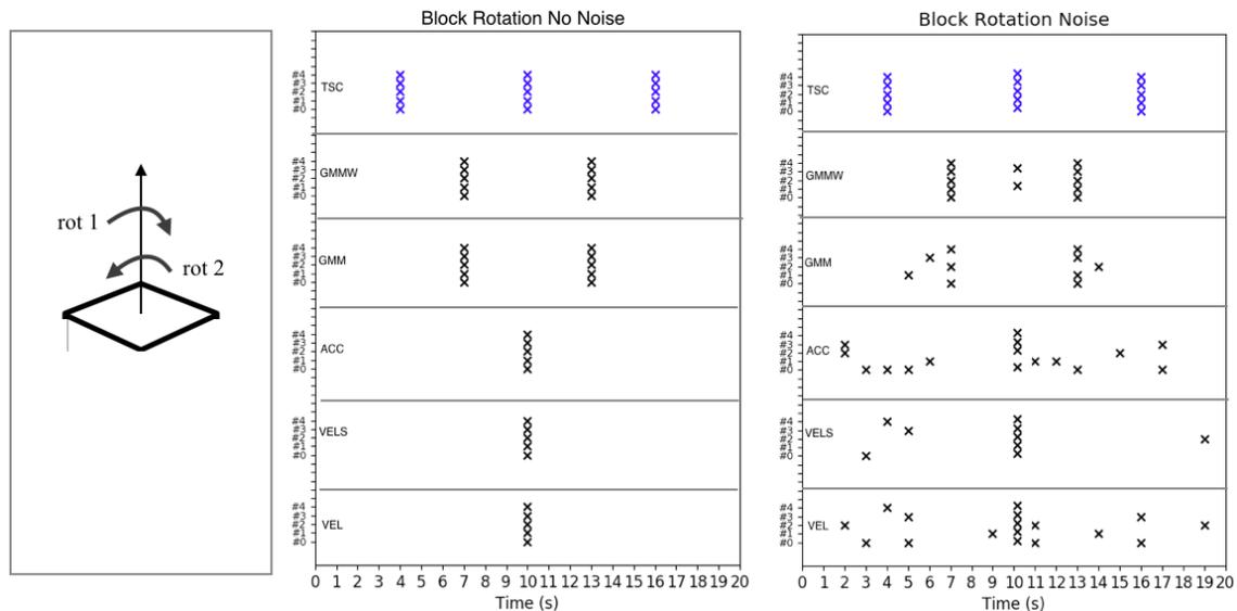
Figure 3.6: Plots the identified transitions with each segmentation algorithm with and without noise. While all techniques are precise when there is no noise, TSC is the most robust in the presence of noise but finds additional segments.
