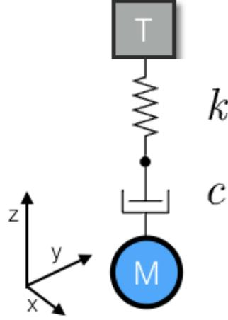
Figure 6.1: This illustration describes a basic mass-spring-damper system with spring constant  $k$  and damping constant  $c$ .
