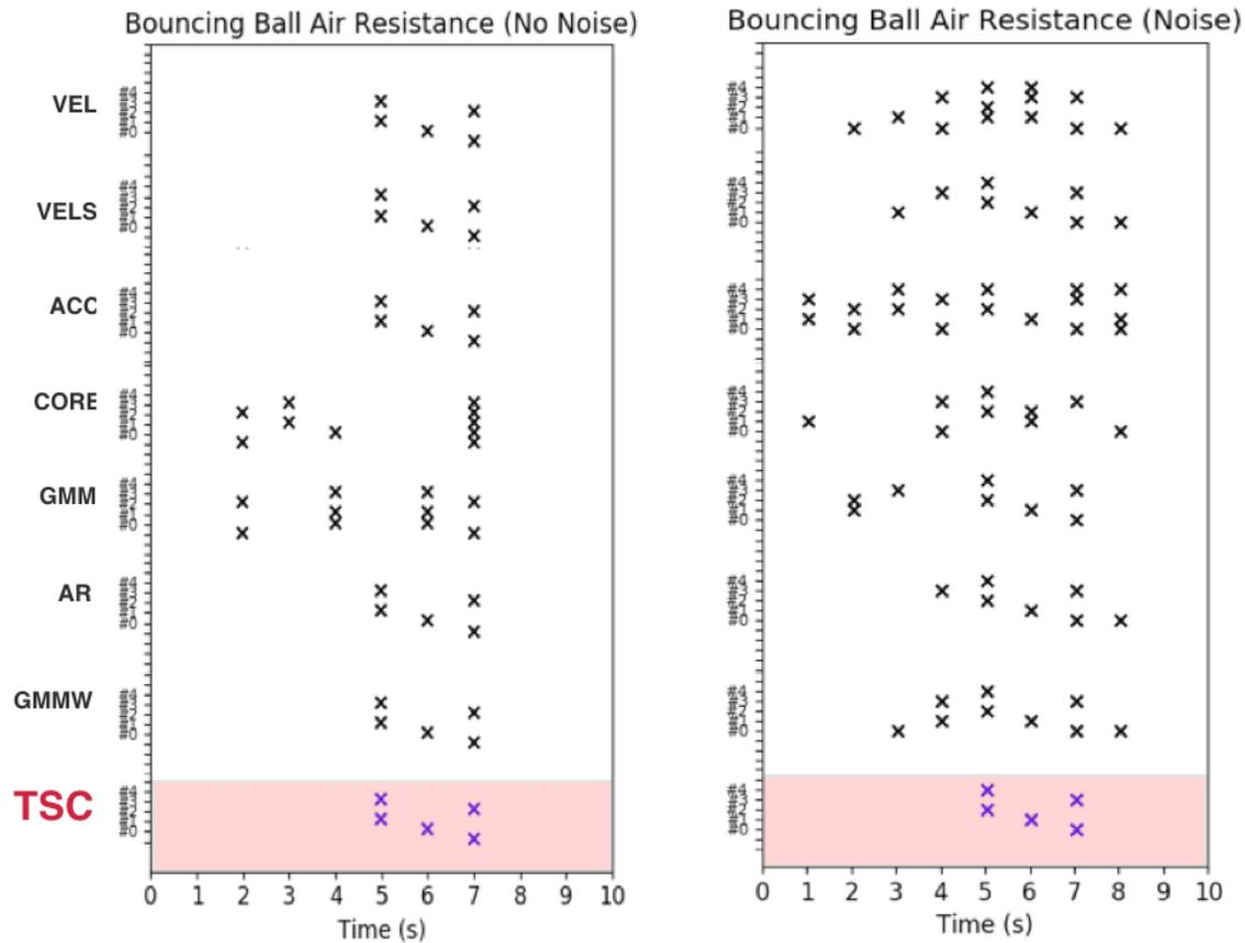
Figure 3.3: Plots the identified transitions with each segmentation algorithm with and without noise. In this example, temporal variation is added by incorporating a random “air resistance” factor. TSC is consistent even in the presence of this temporal variation.
