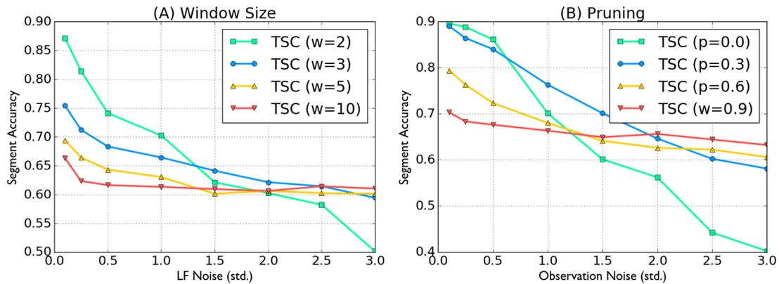
Figure 3.11: (A) shows the performance curves of different choices of windows as a function of the process noise. Larger windows can reject higher amounts of process noise but are less efficient at low noise levels. (B) the performance curves of different choices of the pruning threshold. Larger pruning thresholds are more robust to high amounts of observation noise but less accurate in the low noise setting. We selected  $(w = 3, \rho = 0.3)$  in our synthetic experiments.
