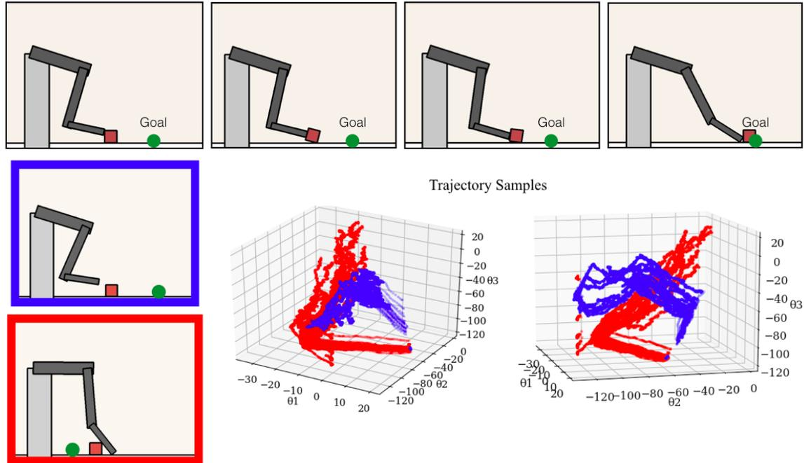
Figure 2.1: A 3-link robot arm has to push a box along a surface with friction to a randomly chosen goal state to the box’s left or right without toppling it. Due to the collision and contact constraints of the 2D Surface Pushing task, it leads to two geometrically distinct pushing skills, backhand and forehand, for goals on the left and on the right. Right: 50 sampled trajectories from a motion-planning supervisor.
