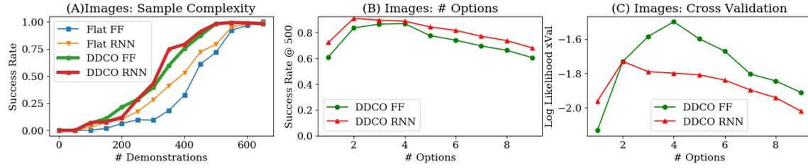
Figure 2.3: 2D Surface Pushing from image observations and image observations. (A) The sample complexity of different policy representations, (B) The success rate for different numbers of discovered options, (C) The peak in the reward correlates over the number of options with the 10-fold cross-validated log-likelihood.
