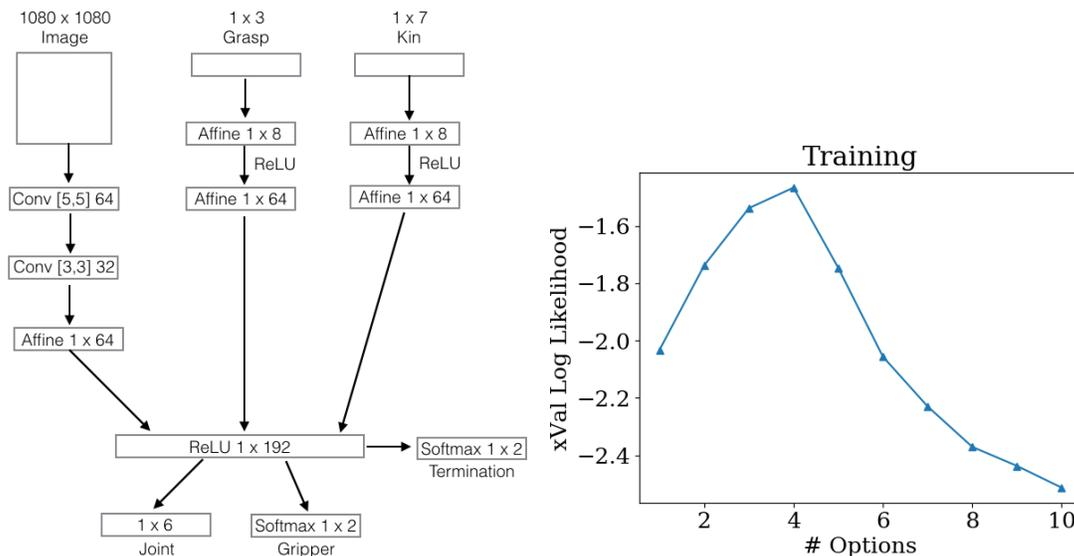
Figure 2.14: We use the above neural network to parametrize each of the four options learned by DDO. In this network, there are three inputs the a binary image, a candidate grasp, and kinematics. These inputs are processed through individual neural net branches and aggregated into a single output layer. This output layer sets the joint angles of the robot and the gripper state (open or closed). Option termination is also determined from this output.
