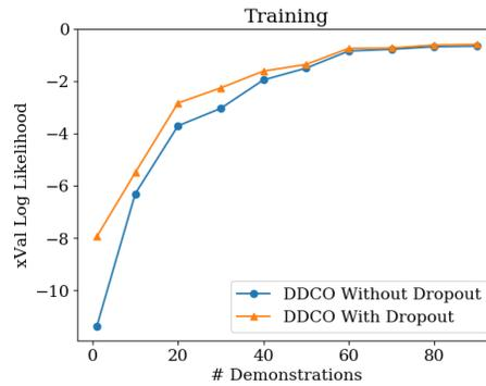
Figure 2.20: Dropout seems to have a substantial effect on improving cross-validation accuracy on a hold out set.
