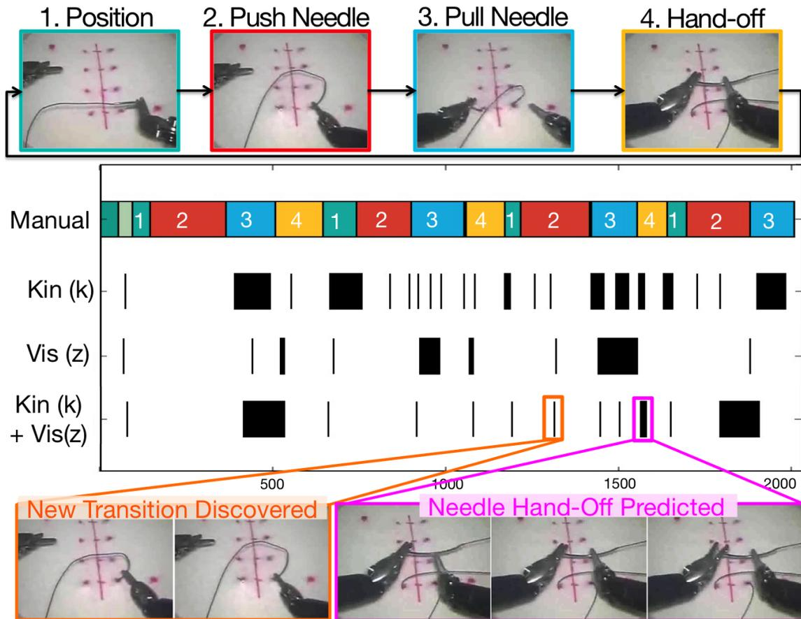
Figure 3.21: The first row shows a manual segmentation of the suturing task in 4 steps: (1) Needle Positioning, (2) Needle Pushing, (3) Pulling Needle, (4) Hand-off. TSC extracts many of the important transitions without labels and also discovers un-labeled transition events.
