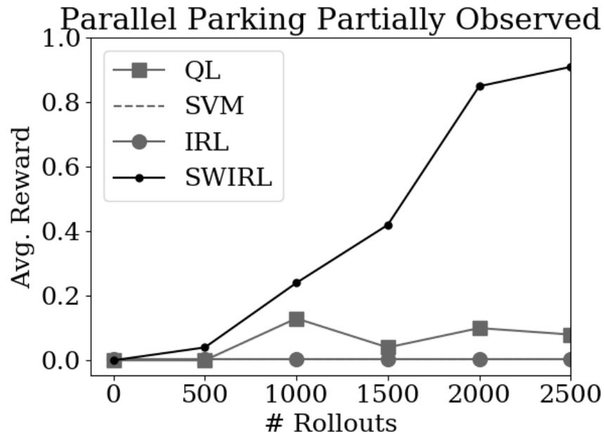
Figure 3.33: We hid the velocity state from the robot, so the robot only sees  $(x, y, \theta)$ . For a fixed number of demonstrations 5, we vary the number of rollouts and measure the average reward at each rollout. (QL) denotes Q-learning, (SVM) denotes a baseline of behavioral cloning with a SVM policy representation, (IRL) denotes MaxEnt-IRL with estimated dynamics, and (SWIRL) denotes SWIRL. SWIRL converges will the other approaches fail to reach a reliable success rate
