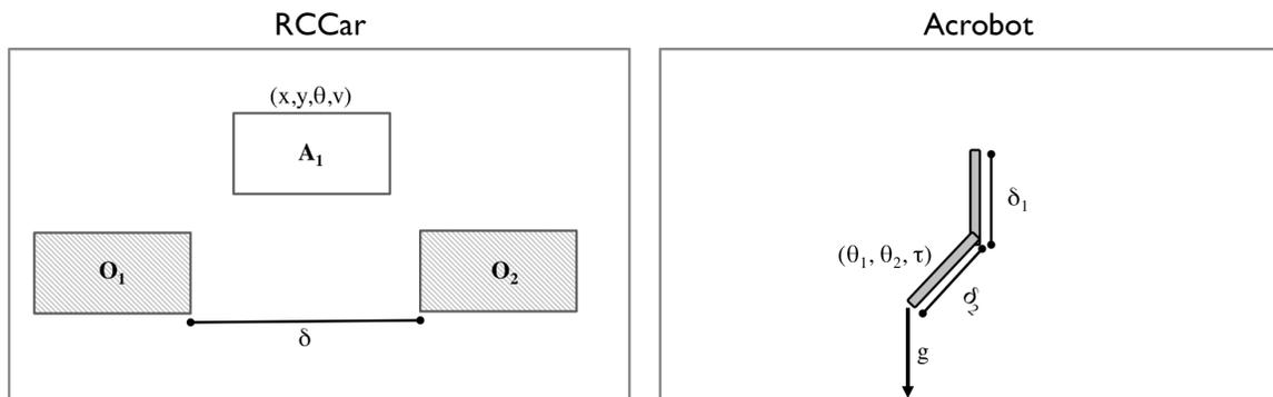
Figure 3.24: (A) Simulated control task with a car with noisy non-holonomic dynamics. The car ( $A_1$ ) is controlled by accelerating and turning in discrete increments. The task is to park the car between two obstacles.
