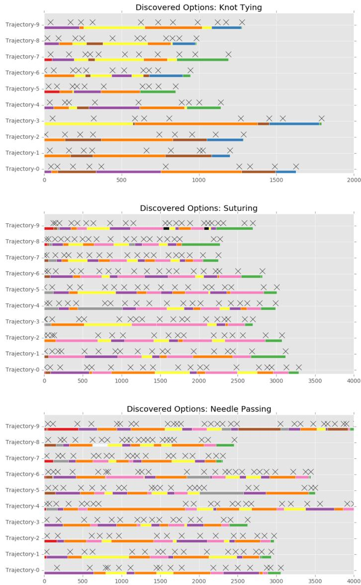
Figure 2.21: Segmentation of human demonstrations in three surgical tasks. Each line represents a trajectory, with segment color indicating the option inferred by DDO as most likely to be active at that time. Human annotations are marked as  $\times$  above the segments. Automated segmentation achieves a good alignment with human annotation — 72% of option boundaries have exactly one annotation in a 300 ms window around them.
