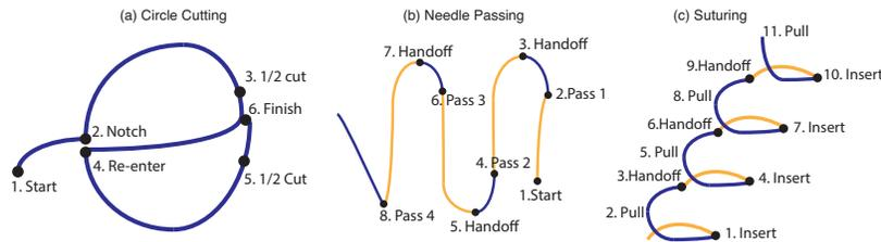
Figure 3.14: Hand annotations of the three tasks: (a) circle cutting, (b) needle passing, and (c) suturing. Right arm actions are listed in dark blue and left arm actions are listed in yellow.
