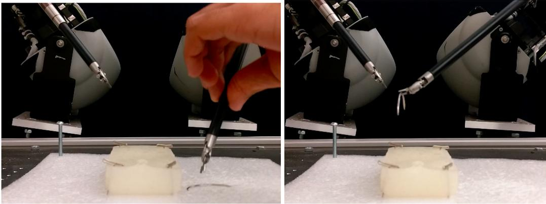
Figure 2.8: To collect demonstrations, we programmed an initial open-loop control policy. We observed the policy execute and interrupted the robot via keyboard input when adjustment was needed.
