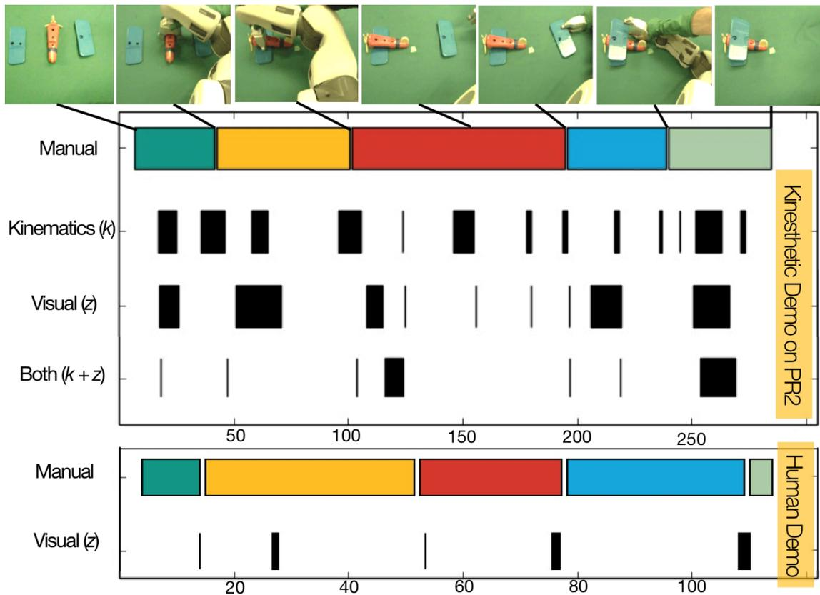
Figure 3.23: We compare TSC on 12 kinesthetic demonstrations (top) and 8 human demonstrations (bottom). No kinematics were available for the human demonstrations. We illustrate the segmentation for an example demonstration of each. Our manual annotation of the task has five steps and TSC recovers this structure separately for both Kinesthetic demos on PR2 and Human demos with the same visual features.
