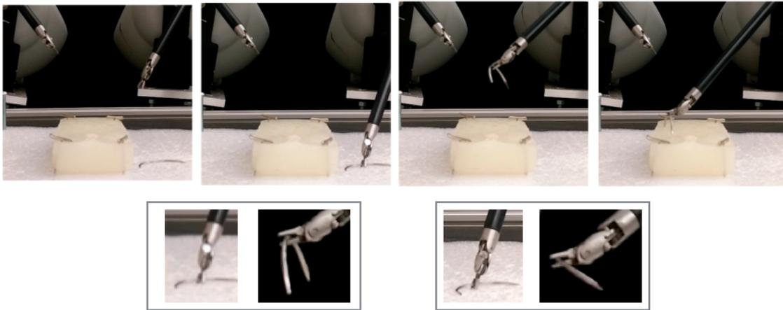
Figure 2.7: A needle orienting and insertion task. The robot must grasp a surgical needle, reorient it in parallel to a tissue phantom, and insert the needle.
