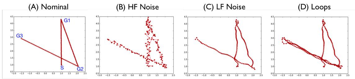
Figure 3.7: One of 20 instances with random goal points  $G1$ ,  $G2$ ,  $G3$ . (a) Observations from a simulated demonstration with three regimes, (b) Observations corrupted with Gaussian white sensor noise, (c) Observations corrupted with low frequency process noise, and (d) Observations corrupted with an inserted loop. See Figure 3.11 for evaluation on loops.
