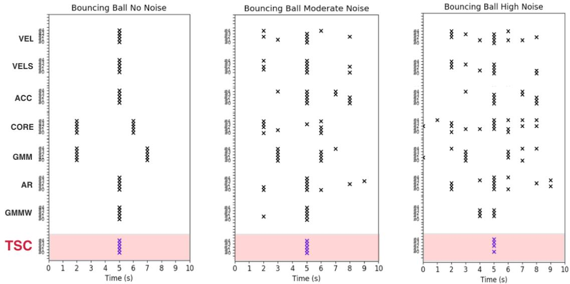
Figure 3.2: Plots the identified transitions with each segmentation algorithm with and without noise. While all techniques are precise when there is no noise, TSC is the most robust in the presence of noise.
