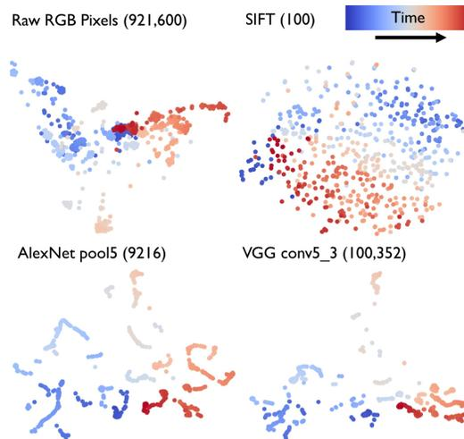
Figure 3.20: Each data point in the figure corresponds to a t-SNE visualization of features of a single frame in the video. (a) RGB pixel values of original image (b) shallow SIFT features (c) CNN features from AlexNet pool5 (d) CNN features from VGG Conv5\_3.
