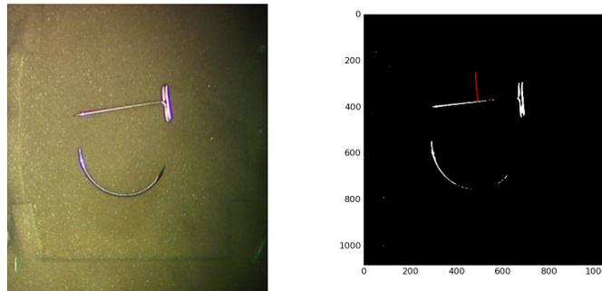
Figure 2.11: The endoscope image and a corresponding binary mask with a selected grasp. The arrow corresponds to the orientation of the gripper along the grasp axis.
