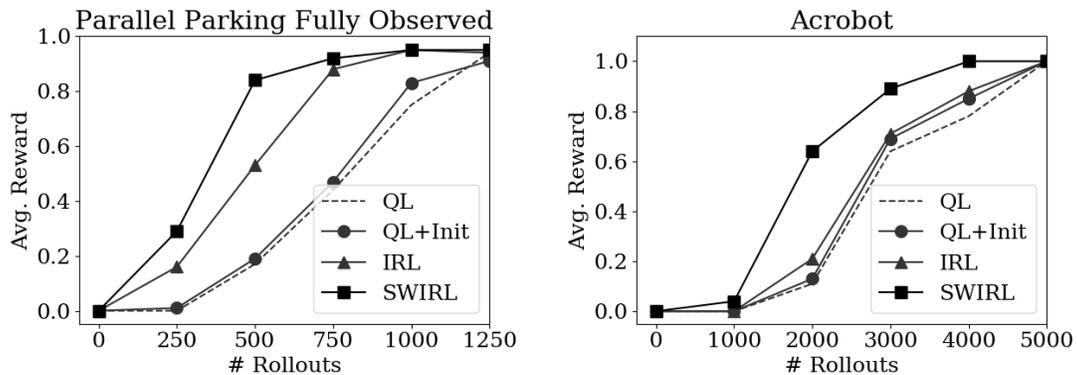
Figure 3.27: Comparison of hybrid approaches. (Parallel Parking) For a fixed number of demonstrations 5, we vary the number of rollouts and measure the average reward at each rollout. (Acrobot) For a fixed number of demonstrations 15, we vary the number of rollouts and measure the average reward at each rollout.
