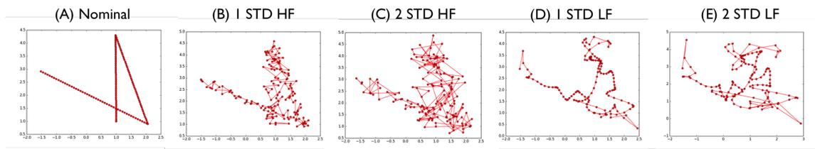
Figure 3.8: (a) Nominal trajectory, (b) 1 std. of high frequency observation noise, (c) 2 std. of high frequency observation noise, (d) 1 std. of low frequency process noise, and (e) 2 std. of low frequency process noise.
