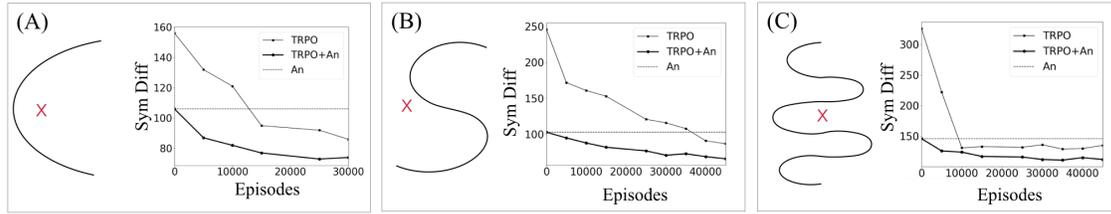
Figure 6.2: This plot shows the expected reward over 50 trials for TRPO, TRPO initialized with the analytic approximation (TRPO AN), and the analytic model on its own. Three cutting curves are visualized of increasing difficulty with a single pinch point marked in red. Results suggest that initializing with an analytic model can greatly accelerate learning.
