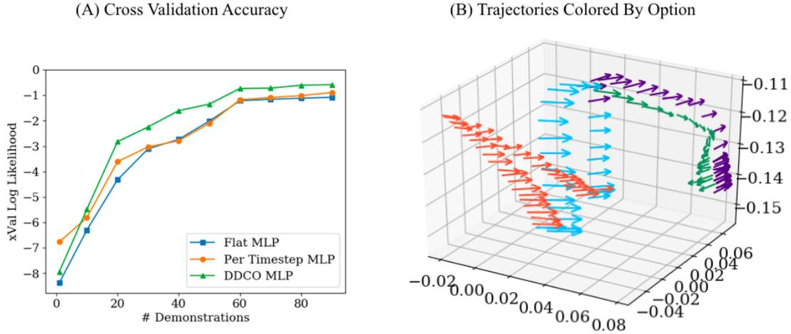
Figure 2.9: (A) We plot the cross validation likelihood of the different methods as a function of the number of demonstrations. (B) We visualize two representative trajectories (position and gripper orientation) color coded by the most likely option applied at that timestep. We find that the two trajectories have the same first two options but then differ in the final step due to the re-orientation of the gripper before insertion.
