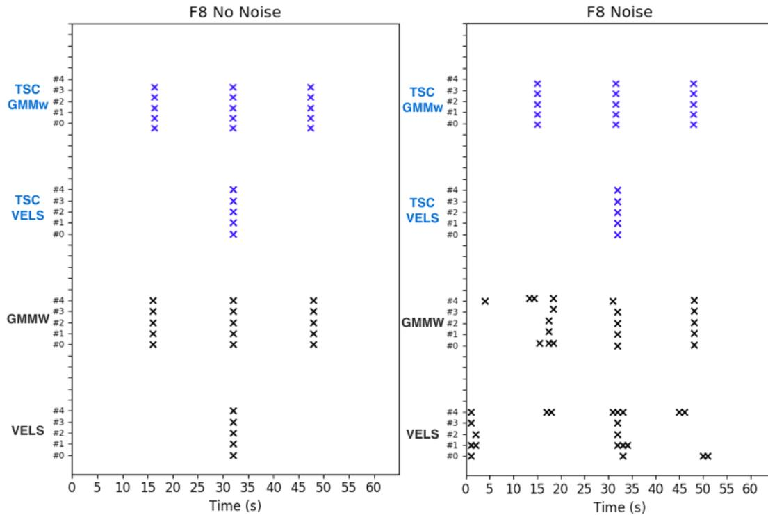
Figure 3.5: Plots the identified transitions with each segmentation algorithm with and without noise. Velocity based segmentation finds one transition point where there is a change in direction. A windowed GMM where the number of clusters is set by a DP finds three transition points. TSC can improve the precision of both techniques.
