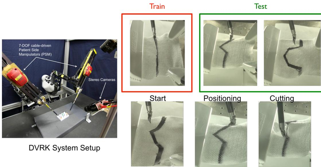
Figure 3.34: We collected demonstrations on the da Vinci surgical robot kinesthetically. The task was to cut a marked line on gauze. We demonstrated the location of the line without actually cutting it. The goal is to infer that the demonstrator’s reward function has two steps: position at a start position before the line, and then following the line. We applied this same reward to curved lines that started in different positions.
