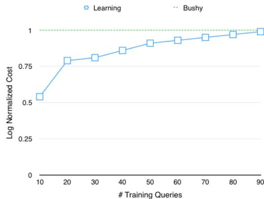
Figure 5.2: The learning curve as a function of the number of queries. The log normalized cost describes the cost difference between learning and the exhaustive bushy optimizer.
