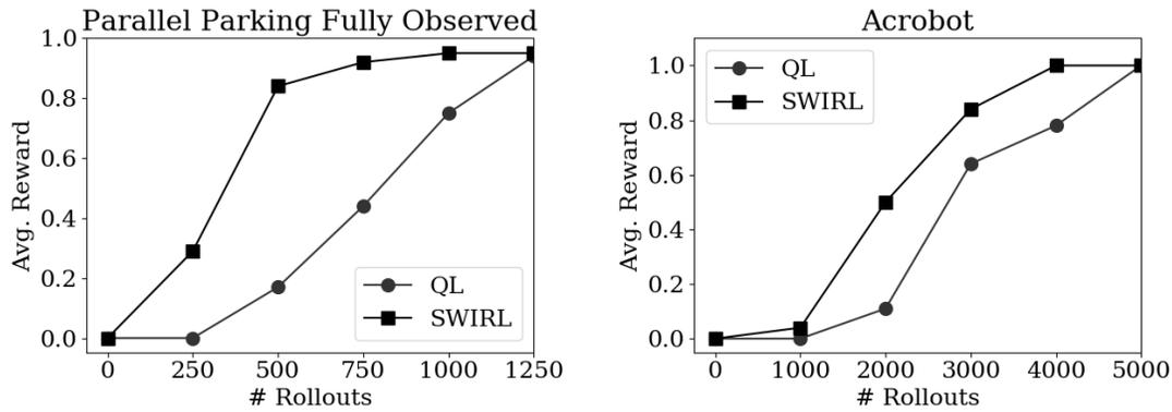
Figure 3.25: Learning curves for Q Learning (QL) and SWIRL on both simulated tasks. (Parallel Parking) For a fixed number of demonstrations 5, we vary the number of rollouts and measure the average reward at each rollout. (Acrobot) For a fixed number of demonstrations 15, we vary the number of rollouts and measure the average reward at each rollout.
