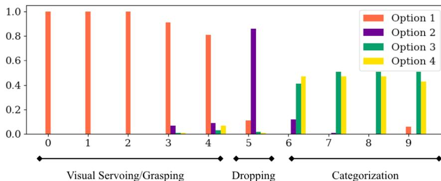
Figure 2.16: We plot the time distribution of the options selected by the high-level policy. The x-axis represents time, and the bars represent the probability mass assigned to each option. We find that the structure of the option aligns with key phases in the task such as servoing to the needle, grasping it, and categorizing.
