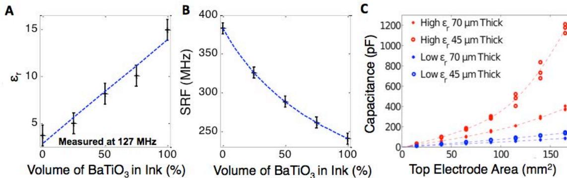
Figure 3.7: **A** Relative dielectric constant, measured at 127 MHz, as the volume of barium titanate in the ink is increased. High dielectric constant is achieved with barium titanate ink, while low dielectric constant is achieved with ultraviolet-curable ink. Error bars show standard deviation. **B**. Self-resonant frequencies of printed capacitors vs. dielectric ink composition **C**. Dependence of capacitance with top electrode area, dielectric thickness and ink composition.
