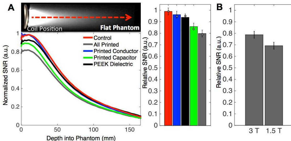
Figure 3.8: **A.** Normalized SNR versus depth into the phantom for coils fabricated with different permutations of printed components at 3T, with schematic showing coil position 3 mm away from conductive fluid. Bar graph summarizes trends shown in relative SNR for each coil type. Dot on bar graph shows predicted SNR, extracted from bench top quality factor measurements. **B.** Relative measured (bars) and bench top-predicted (dots) image SNR of printed coils at 1.5T and 3T.
