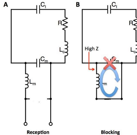
Figure 1.5 **A.** Effective coil circuit during reception. No bias to diode makes it appear removed from the circuit. **B.** When PIN diode is biased it passes RF energy, creating a trap circuit that prevents current from circulating on the main loop.
