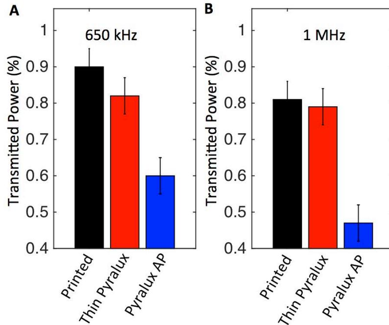
Figure 5.13: Acoustic transmission for printed coil structure (black) Pyralux AP 9121R (red) Pyralux AP 7156E (blue) at **A** 650 kHz and **B** 1 MHz. All materials were encapsulated in 76  $\mu\text{m}$  of PTFE on both sides.
