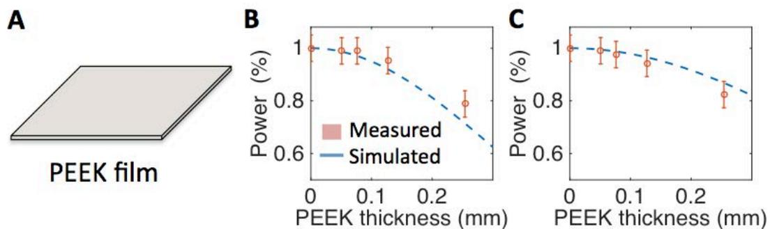
Figure 5.9: **A.** Illustration of the PEEK test film **B.** Relative acoustic power for several thicknesses of the PEEK plastic at 1 MHz and **C.** 650 kHz. Dotted blue line shows attenuation estimated by the acoustic model described in section 5.1.1 [16].
