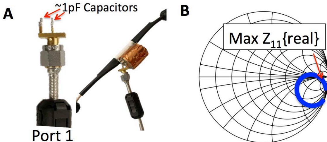
Figure 2.8 **A.** Photograph showing the setup used for the balun input impedance measurement by making contact across the tuning capacitor. **B.** Smith chart illustrating the location of the maximum real impedance of the balun using a capacitor tipped probe.
