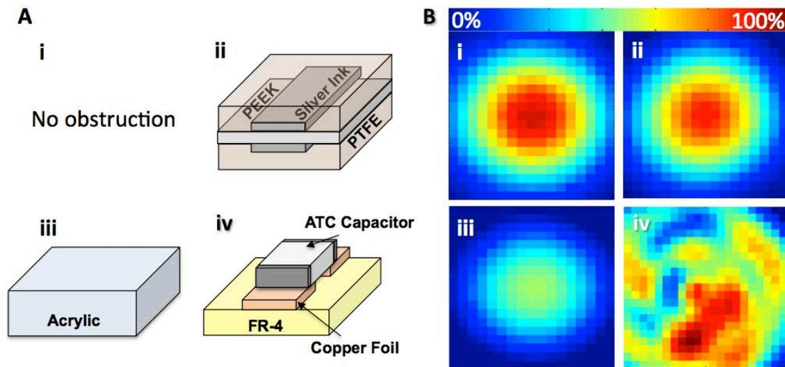
Figure 5.12: **A.** Illustrations of (i) no obstruction, (ii) printed coil capacitor in beam path, (iii) 2 mm acrylic plastic, and (iv) traditionally used porcelain tuning capacitor in beam path tested for attenuation and scattering **B.** 2D acoustic profiles for transducer focal point over 4x4 mm area showing relative intensity with (i) no obstruction, (ii) printed coil capacitor in beam path, (iii) 2 mm acrylic plastic, and (iv) traditionally used porcelain tuning capacitor in beam path.
