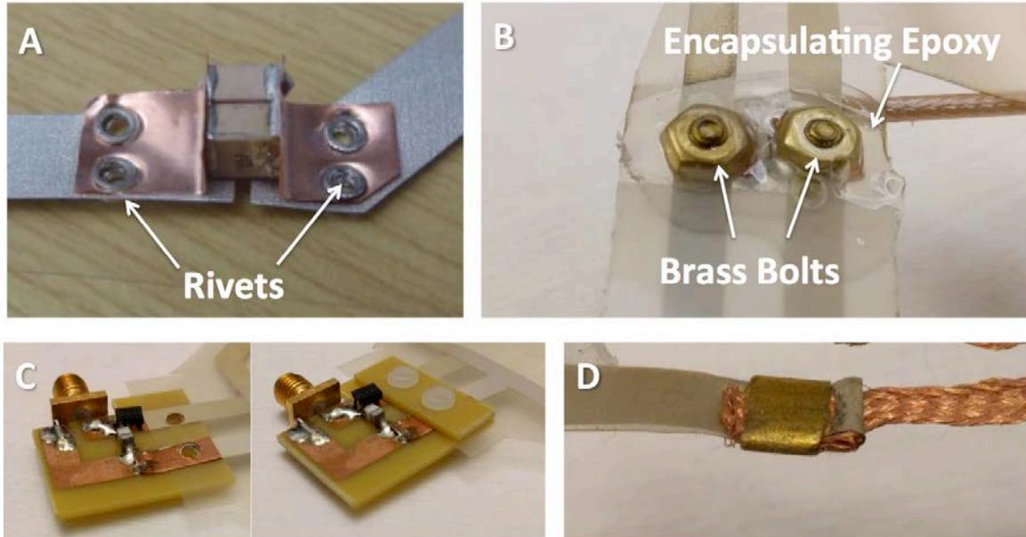
Figure 2.11: **A.** Photograph showing copper strips riveted to the printed coil. **B.** Photograph of the brass bolts clamping the coaxial cable to a printed coil **C.** Photographs showing the clamping board interfacing between printed and non-printed components for a single coil testing. A thin copper strip is soldered onto the board to make the top contact to the coil. **D.** Close up photograph showing the brass crimp used to join the printed array to the coaxial cables and copper braid.
