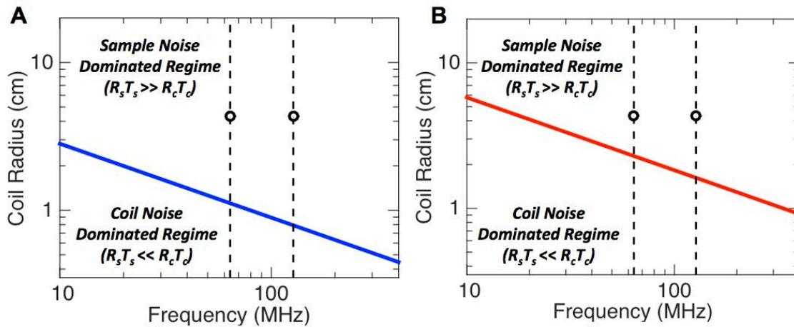
Figure 3.6: Frequency dependence of sample noise and coil noise dominated regimes. For **A** copper based coil and **B** printed conductor coil. Black circles highlight coil used in example at 1.5 and 3 T.
