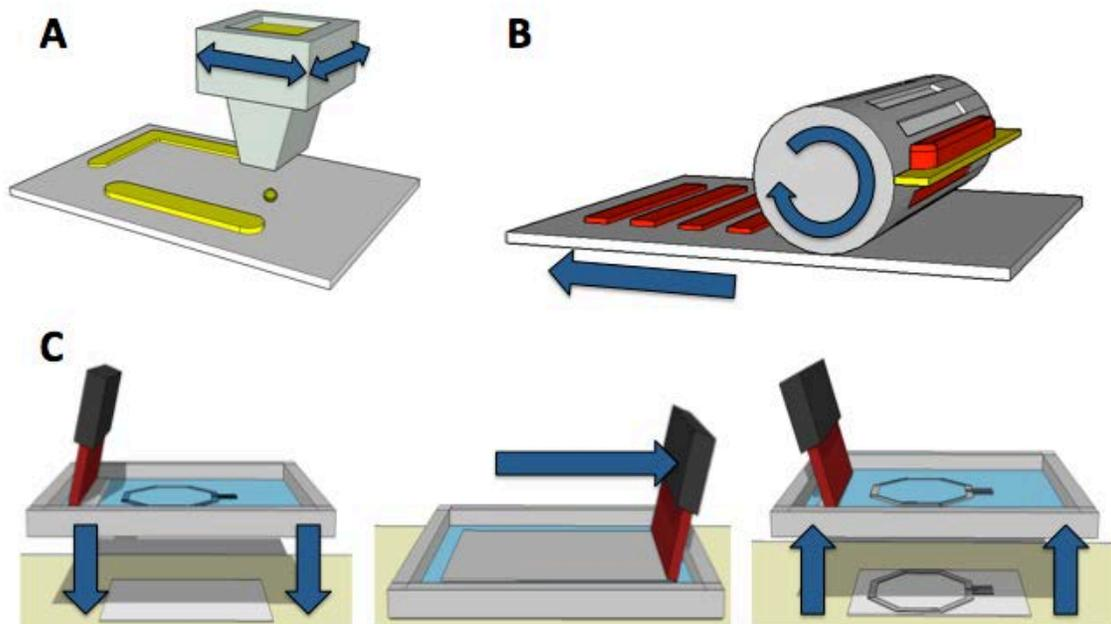
Figure 1.16: **A.** Inkjet printer nozzle depositing ink (yellow) drop-by-drop to create patterns on the substrate below. **B.** Gravure printer (gray cylinder) depositing ink (red) in a pattern as the etched cylinder is rolled along substrate. **C.** Screen printer depositing ink through patterned holes in the screen.
