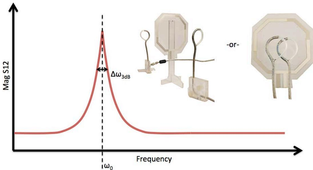
Figure 2.3: Setup and measurement of a surface coil's quality factor by an  $S_{21}$  measurement. Insets show two possible decoupling configurations used to perform the measurement. This technique does not require any special preparation of coil input impedance.
