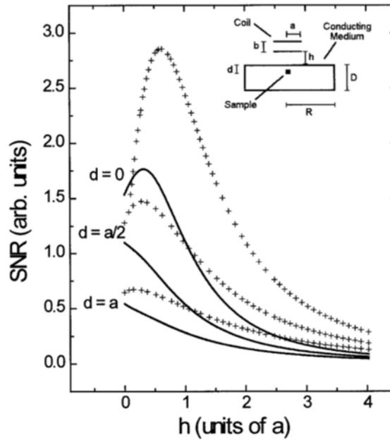
Figure 1.13: Dependence of SNR on coil height for signals from a depth  $d$  for an ideal simple surface coil (solid line) and a two coil NMR gradiometer probe (dotted line) system with the coil spacing equal to one-half the coil radius ( $b = a/2$ ) as computed using Eq. 1.8. The inset shows the geometry used here. (Reproduced from Suits et. Al [30] with permission)
