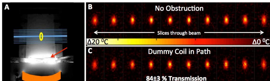
Figure 5.17: **A.** Scan of the phantom on a fibroid transducer using printed array. Red arrow shows location of the array, orange shape highlights location of the transducer, blue lines show the locations of slices used to track heating, and yellow oval shows approximate location of heating. **B.** Heating point inside of phantom without a coil and **C** with the array present. Heating is tracked with body coil in both cases for maintain the same conditions for comparison.
