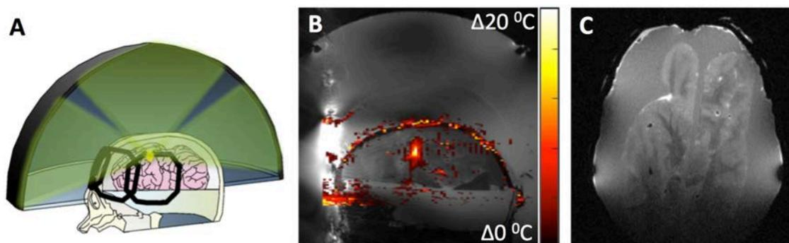
Figure 5.18: **A.** Illustration showing printed array wrapped around skull and brain phantom containing bovine brain submerged in water inside the head transducer. **B.** Sagittal of brain phantom with overlaid heating map tracked with 4-channel array. **C.** Axial scan of skull and brain phantom showing anatomical image quality from the 4-channel array.
