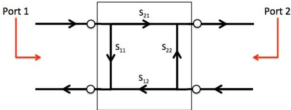
Figure 2.1: Scattering parameters from a general 2-port network. The scattered waves from ports 1 and 2, represented by arrows, are shown as the scattering parameters  $S_{11}$ ,  $S_{12}$ ,  $S_{21}$ ,  $S_{22}$ .
