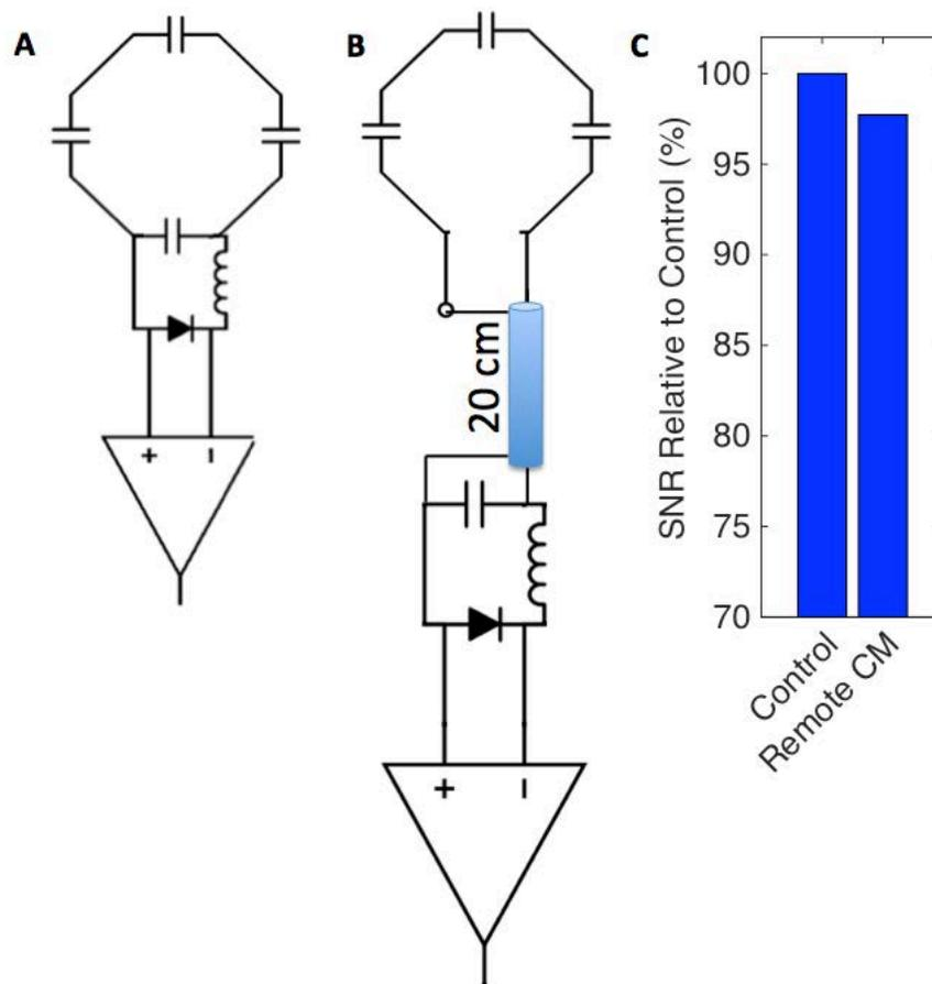
Figure 4.8: **A.** Schematic of the coil circuit with close Q-spoiling circuit. **B.** Schematic of coil with remote matching capacitor and Q spoiling circuit. **C.** SNR from scans taken with the coils using circuits shown in **A** and **B**.
