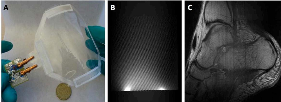
Figure 2.10: **A.** Photograph of a coil design connected to the scanner by a loose clamping alligator clips. **B.** Image of a phantom and **C** of a volunteer illustrating sine wave artifacts caused by the spiking induced by ineffective coil connection.
