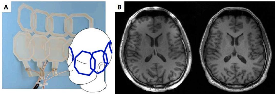
Figure 4.12: **A.** Photograph of two printed 4-channel arrays combined to make an 8-channel array and placement on a volunteer. **B.** Axial slice of a volunteer's brain using (left) the printed coil array and (right) the commercially available 12-channel head array. Similar to phantom images, printed coil shows higher SNR near surface of the brain and slightly lower in the center compared to commercial 12-channel array.
