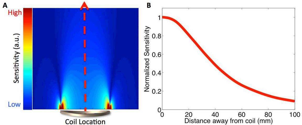
Figure 1.12: **A.** Sensitivity profile for 10 cm diameter receive coil in free-space calculated with equations 1.2-1.7. Red dotted cutline shows location of coil centerline. **B.** Sensitivity along central axis of coil in free-space.
