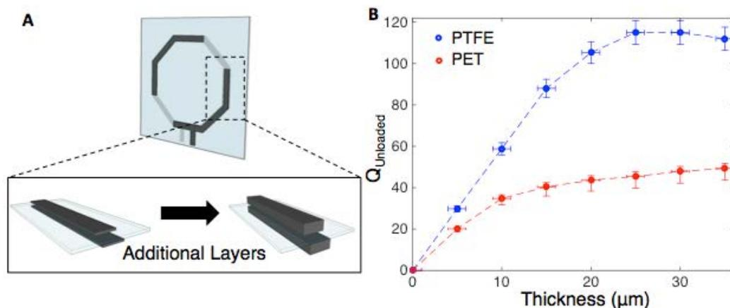
Figure 4.6: **A.** Illustration of a printed coil with inset showing an increase of the printed layer (grey) thickness, obtained by printing additional layers of conductor. **B.**  $Q_{\text{Unloaded}}$  of coils made with increasing thickness of DuPont 5064H silver ink for highest (PTFE) and lowest (PET) performing flexible substrates in blue and red. [Reproduced with permission from Corea et al. [7]]
