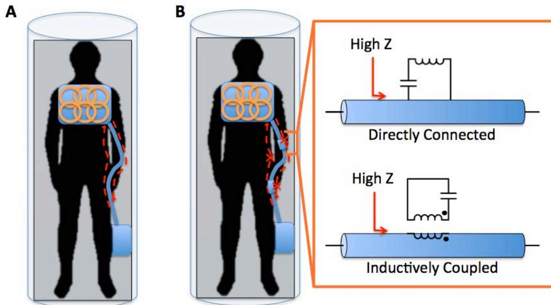
Figure 1.8: **A.** Patient in scanner with coil array placed on chest inside scanner without baluns. Red dotted lines show potential current loop. **B.** Patient in scanner with balun equipped coil array. Baluns break up current loop with high impedance and prevent coupling to the transmit coil. Inset shows (top) directly soldered balun circuit and (bottom) inductively coupled balun circuit used to create high impedance on the outside of the cable.
