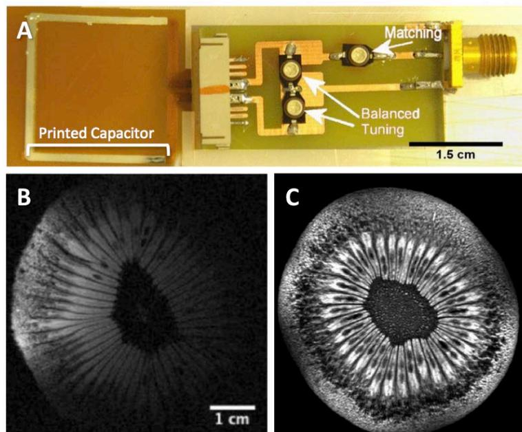
Figure 1.17: **A.** Photograph of a flexible coil fabricated using inkjet printing. **B.** Scan of a kiwi fruit using flex coil from Mager et al at 9.4 T. (reproduced with permission from Mager et al. [53]). **C.** Higher SNR image of kiwi fruit from 4.7 T scanner with an inflexible coil. (Image reproduced with permission from Erikson et al. [54]).
