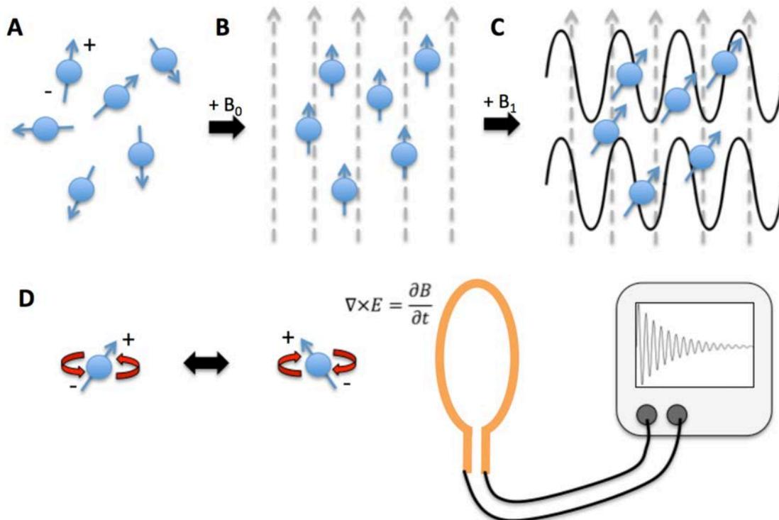
Figure 1.1: **A.** Nuclear spins with magnetic moments randomly oriented with out an external field **B.** Spins aligning with the external magnetic field. **C.** Radio frequency energy is applied to impart some flip angle to spins, creating a transverse magnetic field component. **D.** The precession of spins creates a changing magnetic field that can be detected using a loop of wire through faraday induction.
