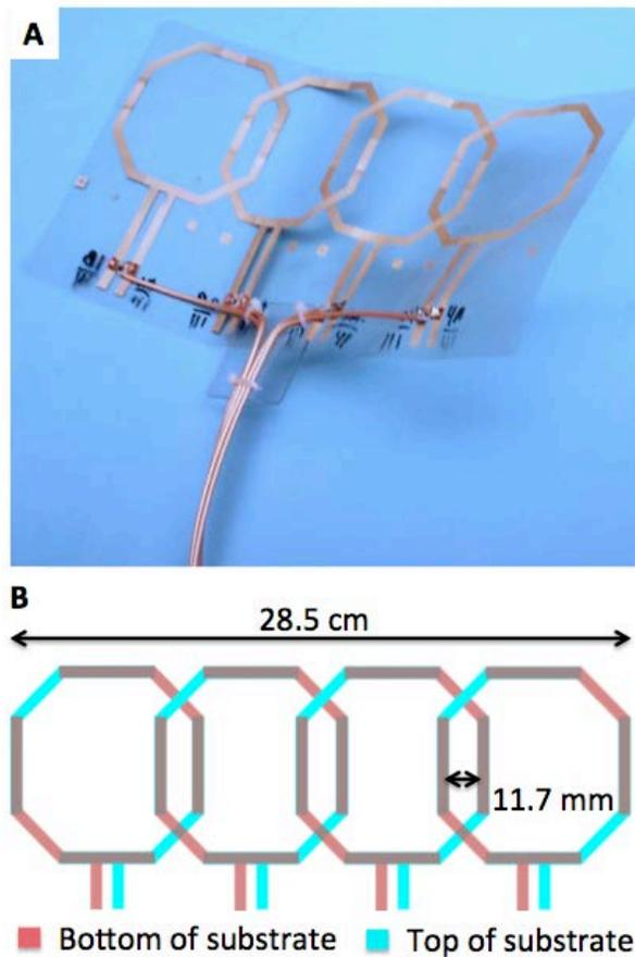
Figure 4.3 **A.** Photograph of coil array. Transmission lines connecting the coils to the MRI scanner are also shown coming out of the bottom of coil array. **B** Single coil elements are shifted to adjacent positions to form a multi-channel array.
