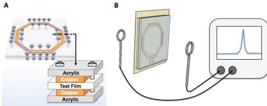
Figure 4.4: **A.** Illustration of the testing rig developed to characterize the dielectric loss of flexible substrates prior to printing. This setup mimics the geometry of the printed coils. The stack of materials is highlighted in lower right. **B.** Illustration of  $Q_{\text{Unloaded}}$  measurement setup using two probes separated by several diameters with test rig in the center.
