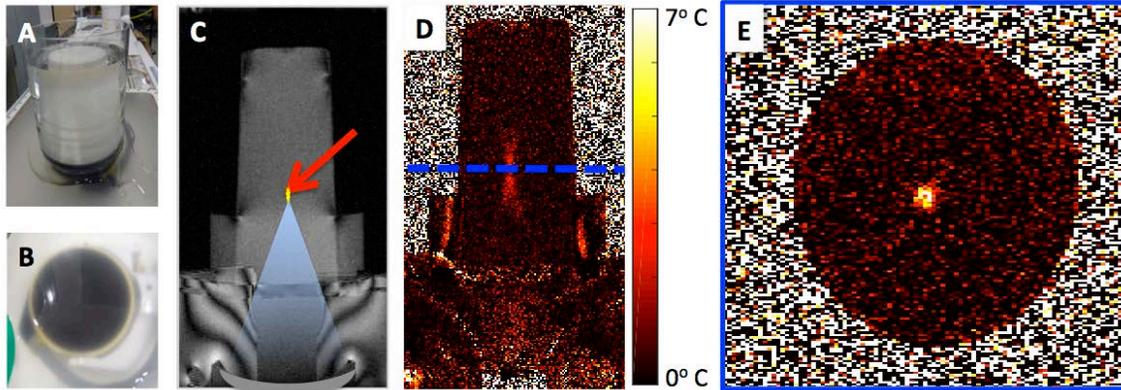
Figure 5.5: **A.** Photograph of gel phantom in water bath. **B.** Top down photograph of ultrasonic transducer. **C.** Cross-sectional magnitude image of phantom sitting on top of transducer with focal path (blue) and focal point (red arrow) highlighted. **D.** Coronal temperature map of cylindrical phantom. Blue dotted line indicates location of maximum temperature map slice shown in **E.**
