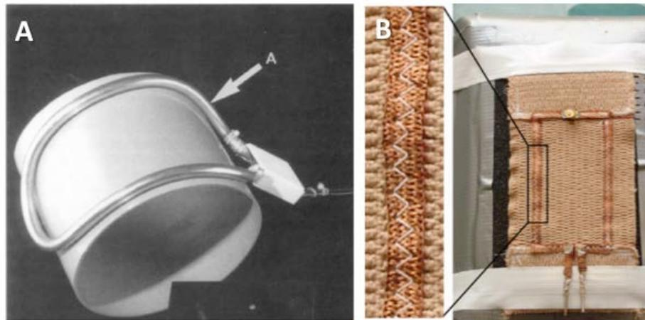
Figure 1.15: **A.** mercury filled tube creating flexible coil (Reproduced with permission from Malko et al.[37]). **B.** Copper wire sewn into stretchable fabric to create flexible and stretchable coil. Inset shows close up of copper sewn into fabric. (Reproduced with permission from Nordmeyer-Massner et al. [39])
