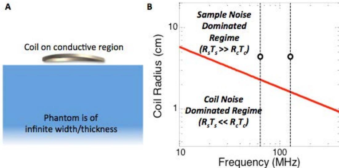
Figure 1.9: **A.** Coil on semi-infinite phantom with conductivity similar to tissue (0.67 S/m). **B.** Frequency dependence of sample noise and coil noise dominated regimes. Black circles highlight coil used in example at 1.5 and 3 T.
