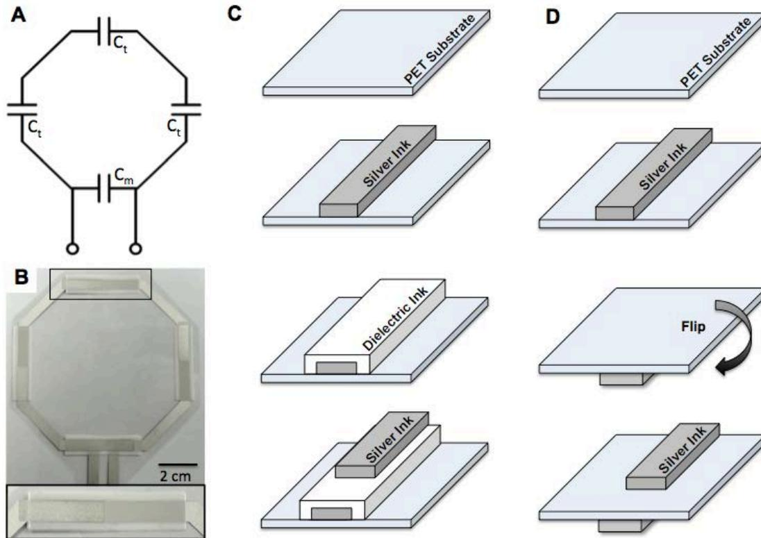
Figure 3.5: **A.** Schematic of a printed coil showing tuning,  $C_t$ , and matching,  $C_m$ , capacitors. **B.** Photograph of a printed coil. Inset highlights top-down view of printed capacitor. **C.** Coil printing process flow with printed dielectric **D.** Coil printing process flow using the substrate as a dielectric.
