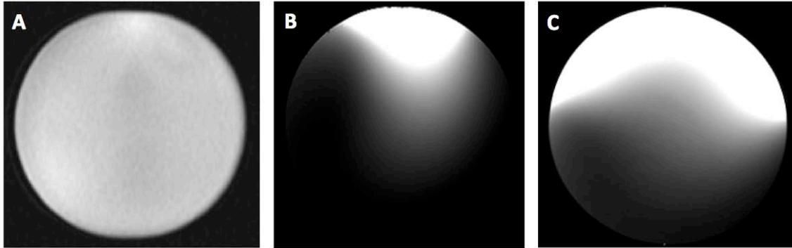
Figure 1.11: **A.** Image of cylindrical phantom with large volume coil showing large field of view but high noise. **B.** Single surface coil image of phantom providing high signal locally on top of phantom, but poor field of view. **C.** Image from array of surface coils providing high signal and an increased field of view. All images were acquired using the same scan parameters and are displayed with similar windowing.
