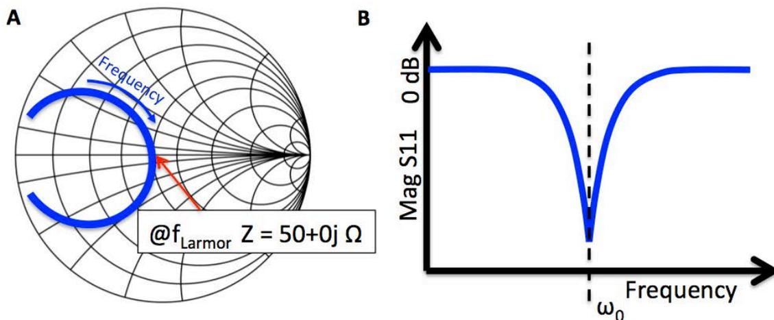
Figure 2.4: **A.** Smith chart of the coil impedance matched to 50 Ω at the Larmor frequency **B.** Magnitude of S<sub>11</sub> response for a properly tuned coil showing minimum response at the Larmor frequency.
