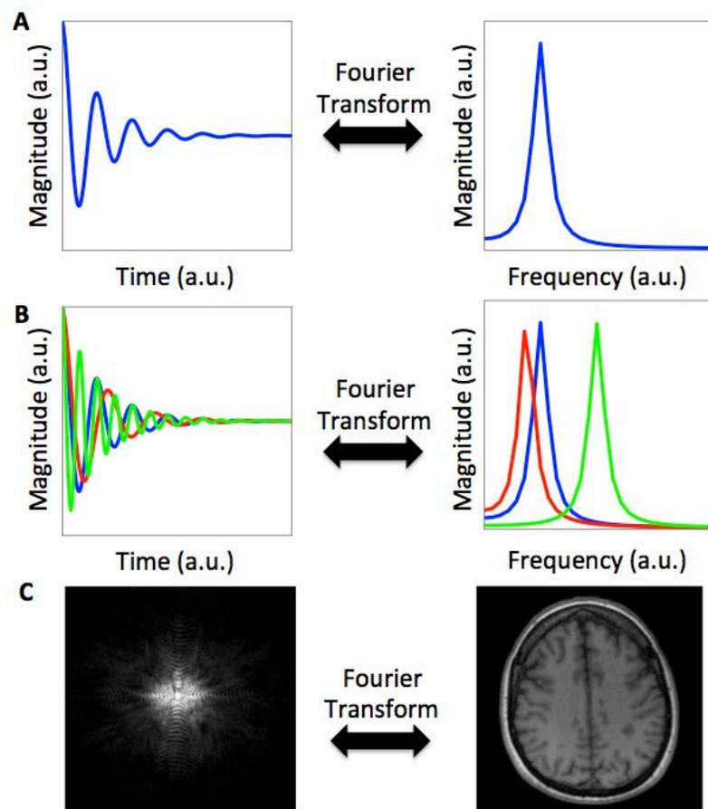
Figure 1.2: **A.** Free-induction decay (FID) from spin at one frequency. Fourier transform reveals frequency. **B.** FID of several spins all at different frequencies received at the same time. Fourier transform reveals separate frequencies. **C.** K-space from scanner and image produced after Fourier transform is taken.
