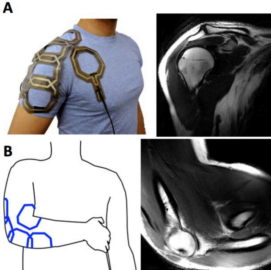
Figure 4.13: **A.** Photograph of the printed array on the shoulder of a volunteer with respective image taken with array. **B.** Illustration of coil on elbow of volunteer in bent position with respective scan from array.
