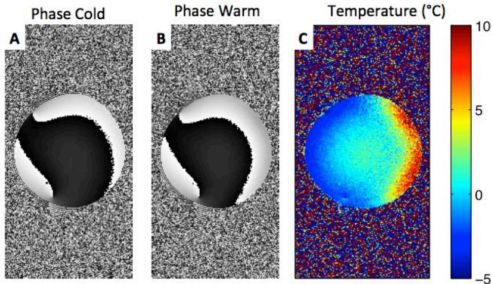
Figure 5.4: **A.** Phase map of a cylindrical gel phantom. **B.** Phase map of the cylindrical phantom after warm tower was applied to right side. **C.** Temperature map showing increase in temperature throughout the entire cross section of the phantom.
