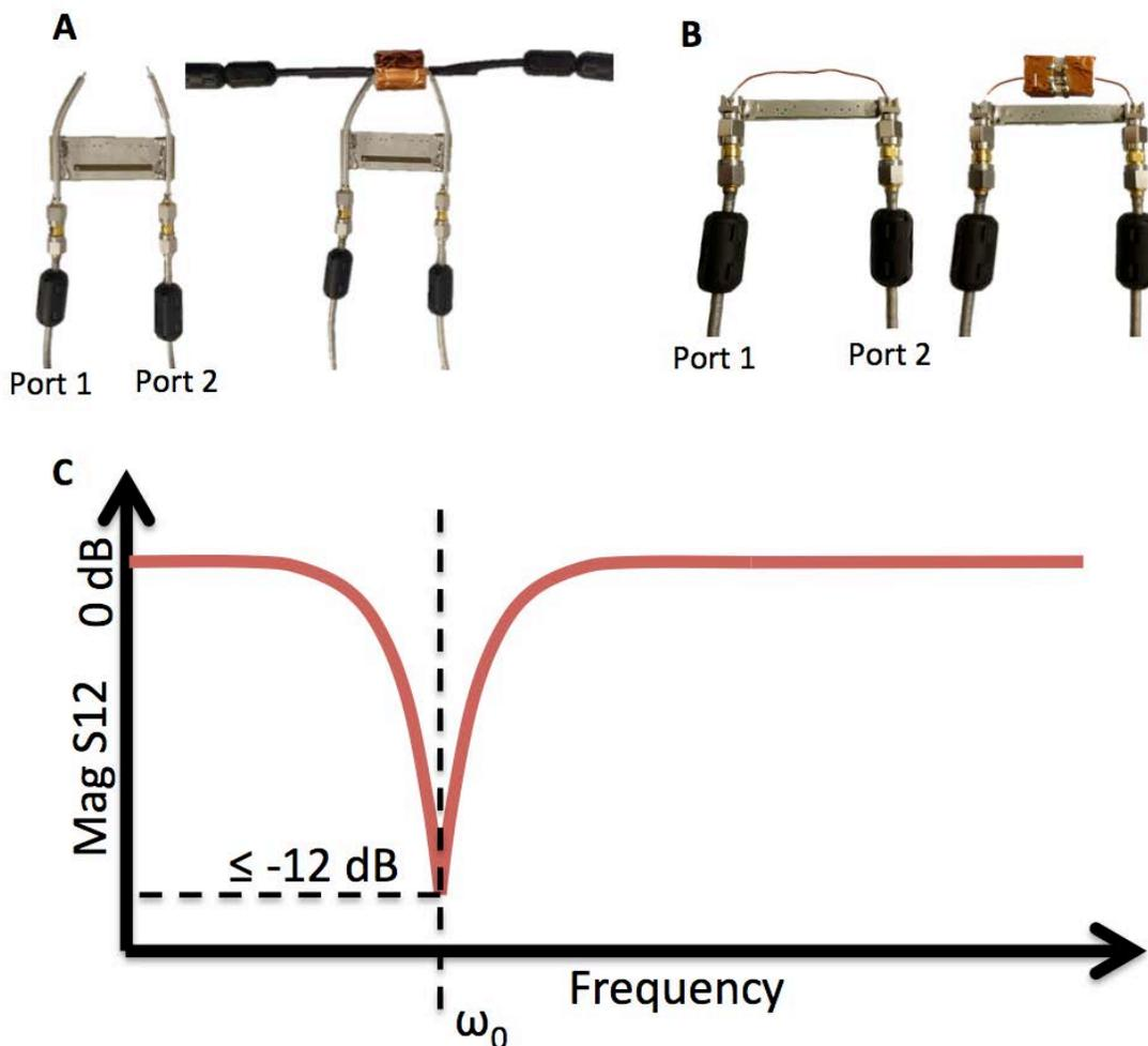
Figure 2.9 A. Photograph of the measurement setup to make momentary contact across the balun with an  $S_{12}$  probe and characterize the impedance. B. Photograph of the measurement setup used to measure the balun attenuation by an inductively coupled  $S_{12}$  probe. C. Typical  $S_{12}$  response of a tuned balun highlighting the location and magnitude of the center frequency.
