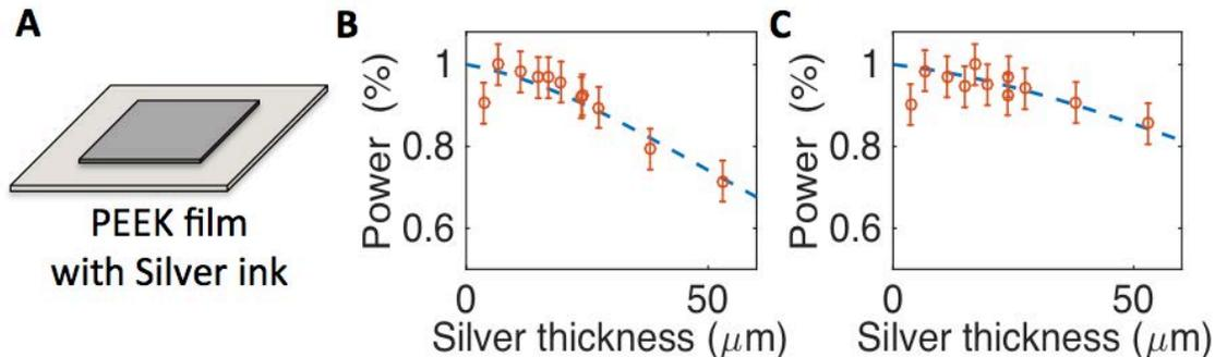
Figure 5.10: **A.** Illustration of the film stack characterized by the acoustic testing. Relative acoustic power for several thicknesses of Dupont 5064H silver ink on 76  $\mu\text{m}$  thick PEEK plastic at **B** 1 MHz and **C** 650 kHz. Dotted blue line shows the attenuation estimated by the acoustic model described in section 5.1.1 [16].
