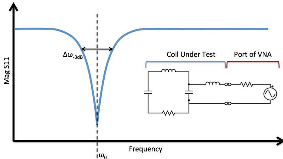
Figure 2.2: Illustration detailing calculation of quality factor for a surface coil by direct  $S_{11}$  measurements. Inset shows the resistance of the port that will dissipate half of the power, artificially lowering the measured  $Q$ .
