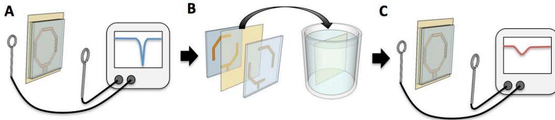
Figure 5.6: **A.** Illustration showing experimental setup during coil  $Q_{\text{Unloaded}}$  measurements in the test rig. **B.** Illustration showing how substrate is immersed in water for 24 hours. **C.** Illustration showing coil changes in  $Q_{\text{Unloaded}}$  and resonance frequency after water submersion.
