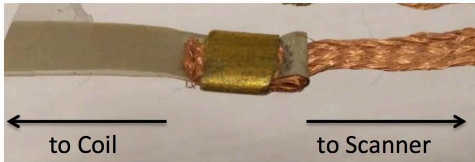
Figure 4.9: Photograph of flexible coil and copper braid crimp connection used to connect the printed array to the scanner.
