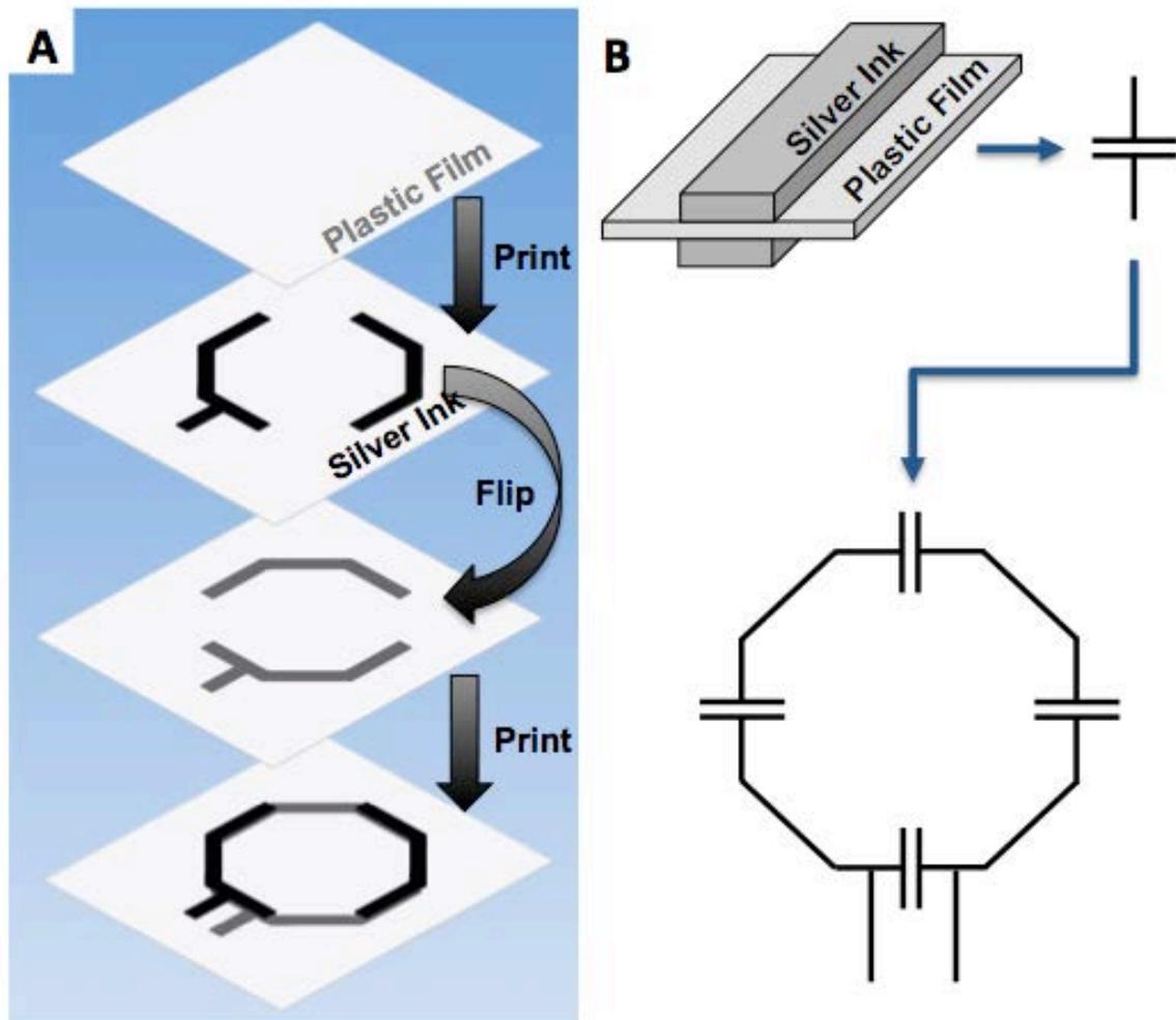
Figure. 4.1: **A.** Illustration of the printed coils fabrication process. Conductive features are printed on each side of the substrate to form tuning and matching capacitors. **B.** Cross-section schematic of coil capacitors formed between two printed metal features and the plastic substrate along with the equivalent circuit of the printed portion of the receive coil.
