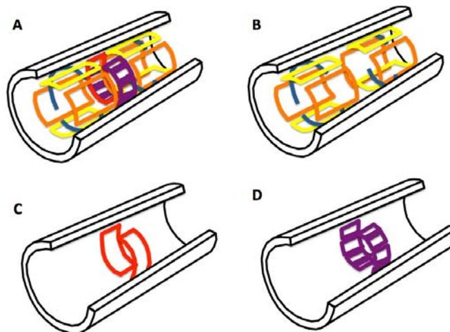
Figure 1.3: **A.** Simplified illustration of different types of coils in an MRI scanner. White coil is the superconducting solenoid that provides a large static magnetic field ( $B_0$ ). **B.** Gradient coils that provide unique magnetic field strength in X, Y and Z. **C.** Transmit coils that excite nuclear magnetic moments in sample with RF pulses. **D.** Shim coils which help maintain field homogeneity when different samples are placed inside scanner.
