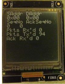
Figure 4-5: LCD Debug Screen via UART
