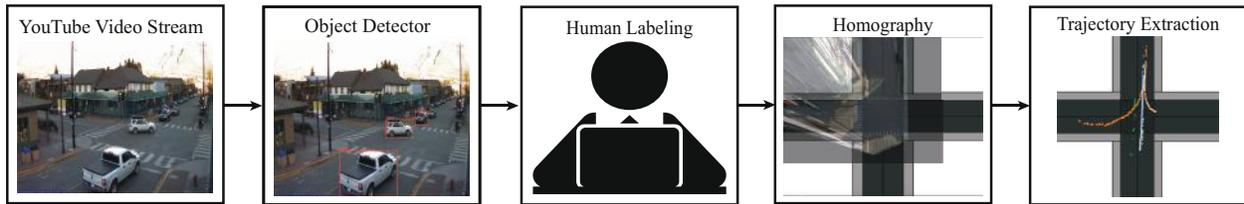
Figure 3.1: TCP system architecture (excluding learning and analysis). First, we capture a video stream of a traffic intersection and use SSD, a deep object detection network, to identify and label vehicles. Then, we manually label the first detection of each vehicle in the video stream. Finally, we map the identified vehicles to a bird’s eye view using homography and run a probabilistic grouping algorithm to extract trajectories.
