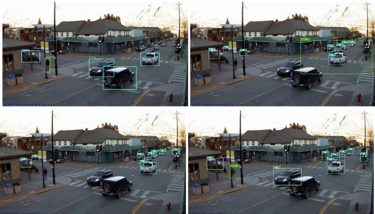
Figure 4.1: Example detections from each of the four networks on a sample daytime image: SSD-VGGNet (top left), SSD-InceptionNet (top right), SSD-MobileNet (bottom left), and Faster-RCNN (bottom right). Detections of cars are shown with blue bounding boxes, and detections of people are shown with green bounding boxes.
