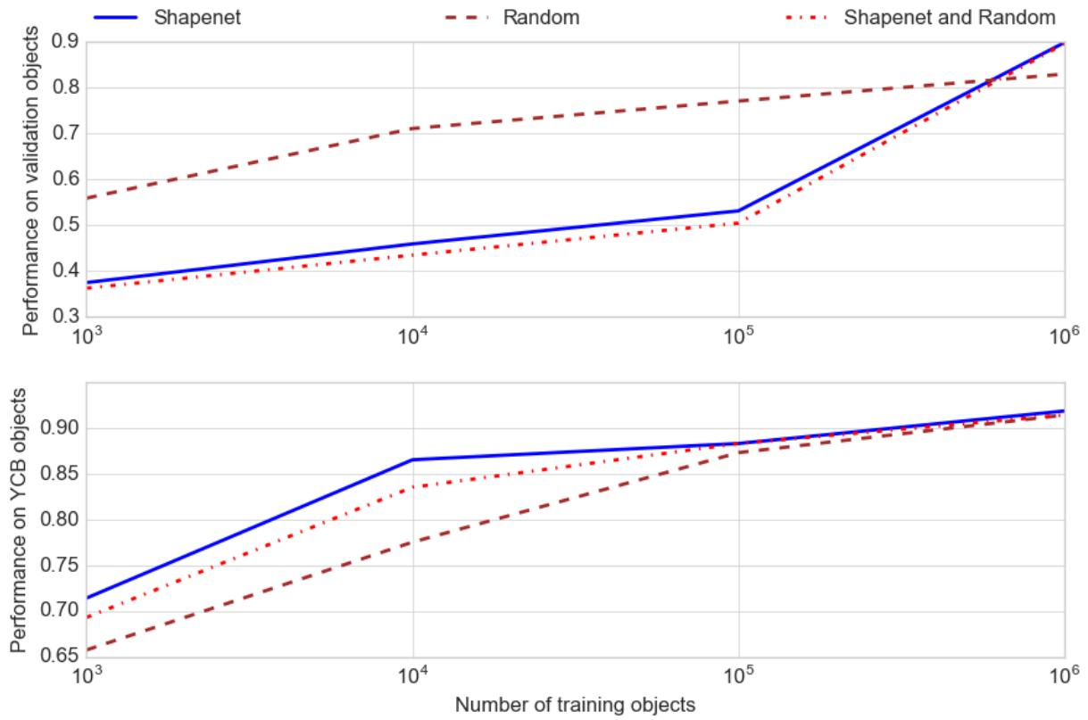
Figure 3.7: Impact of number of unique training objects used on the performance of the learned model on held out data at test time. Each line represents a different training set. The top chart indicates the performance of the models on held out data from the same distribution (i.e., held out ShapeNet or Random objects depending on the training set), and the bottom chart shows performance on out-of-sample objects from the ShapeNet dataset.
