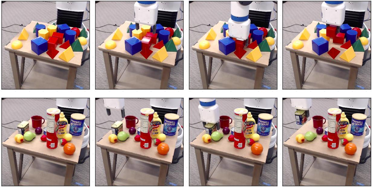
Figure 2.12: Two representative executions of grasping objects using vision learned in simulation only. The object detector network estimates the positions of the object of interest, and then a motion planner plans a simple sequence of motions to grasp the object at that location.
