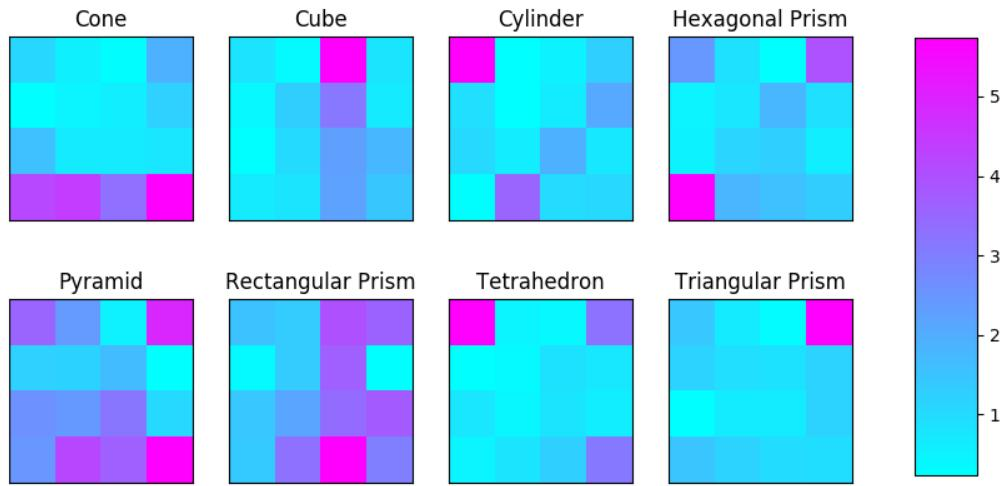
Figure 2.7: Error distribution by object position. We divided the table into 4 horizontal and 4 vertical buckets. The bottom-left of each heatmap corresponds to the front-left corner of the table in the camera frame. The scale on the right represents average error in centimeters.
