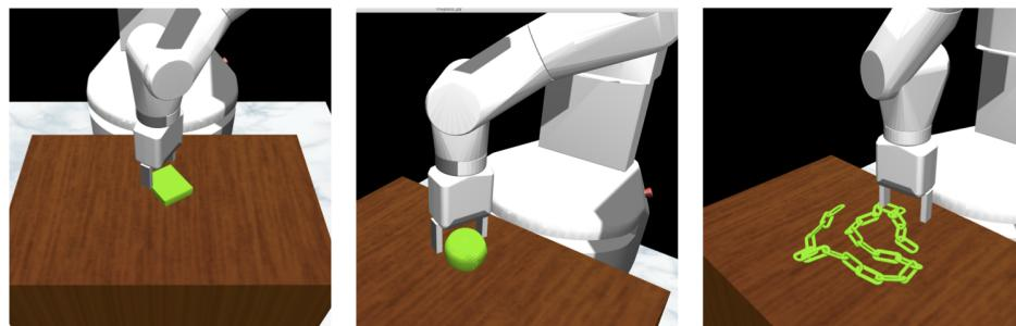
Figure 3.5: Examples of three observed failure cases for our learned models. Left: the model chooses a grasp for an object that is close to the maximum size of the gripper that collides with the object. Middle: the model chooses a grasp for a large, highly curved object that causes it to slip off. Right: the model fails to find a promising grasp for a highly irregular object.
