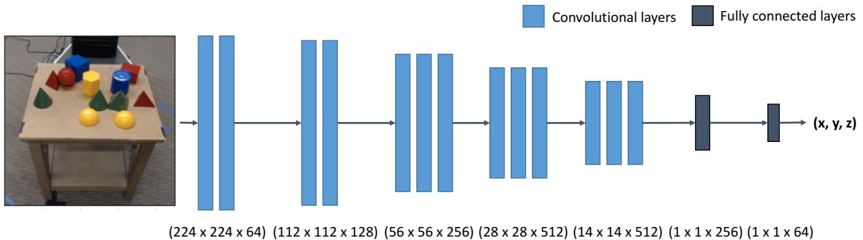
Figure 2.2: The model architecture used in our experiments. Each vertical bar corresponds to a layer of the model. ReLU nonlinearities are used throughout, and max pooling occurs between each of the groupings of convolutional layers. The input is an image from an external webcam downsized to  $(224 \times 224)$ .
