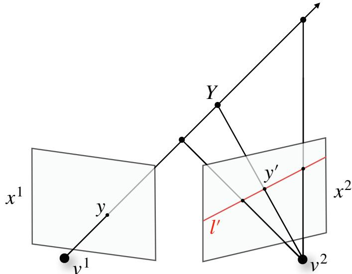
Figure 4.2: Illustration of the epipolar geometry. For any image point  $y$  in  $x^1$  corresponding to a 3D point  $Y$ , the image point  $y'$  in  $x^2$  that corresponds to  $Y$  is constrained to lie on a line  $l'$  in  $x^2$ . This line corresponds to the projection onto  $x^2$  of the ray passing through the camera center of  $v^1$  and  $y$ . This line depends only on the intrinsic geometry between  $v^1$  and  $v^2$ , not the content of the scene.
