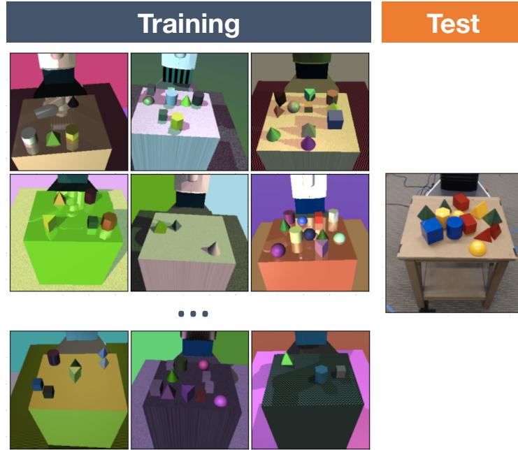
Figure 2.1: Illustration of our approach. An object detector is trained on hundreds of thousands of low-fidelity rendered images with random camera positions, lighting conditions, object positions, and non-realistic textures. At test time, the same detector is used in the real world with no additional training.
