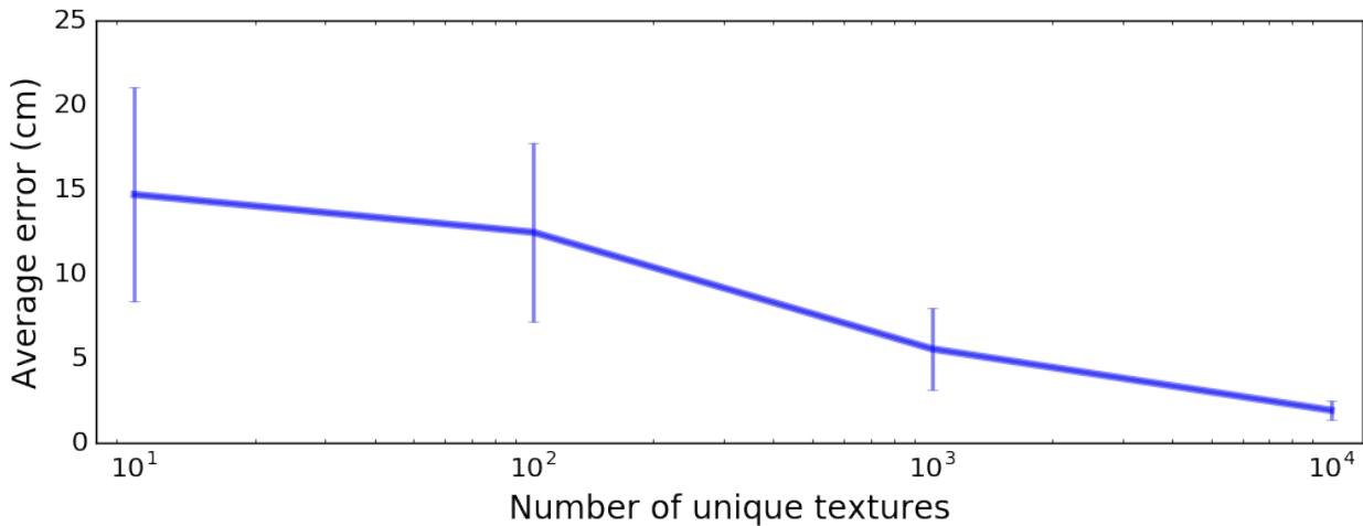
Figure 2.10: Sensitivity to amount of texture randomization. In each case, the detector was trained using 10,000 random object positions and combinations of distractors, but only the given number of unique texturizations and lighting conditions were used.
