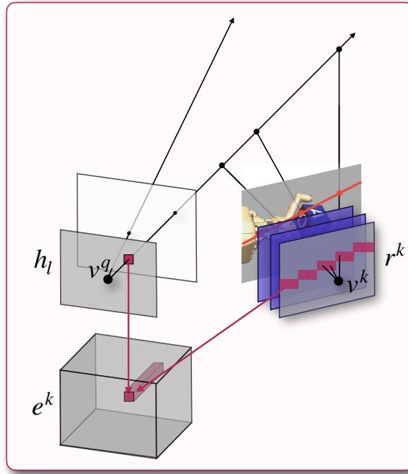
Figure 4.3: Constructing the epipolar representation  $e^k$  for a given camera viewpoint  $v^k$ . For a given spatial position in the decoder state  $h_l$ , there is a 1-dimensional subset of feature maps  $l'$  in  $r^k$  arising from the epipolar geometry. This can be viewed as the projection of the line passing from the camera center at  $v^q$  through the image point onto  $r^k$ . The epipolar representation  $e^k$  is constructed by stacking these lines along a third spatial dimension.
