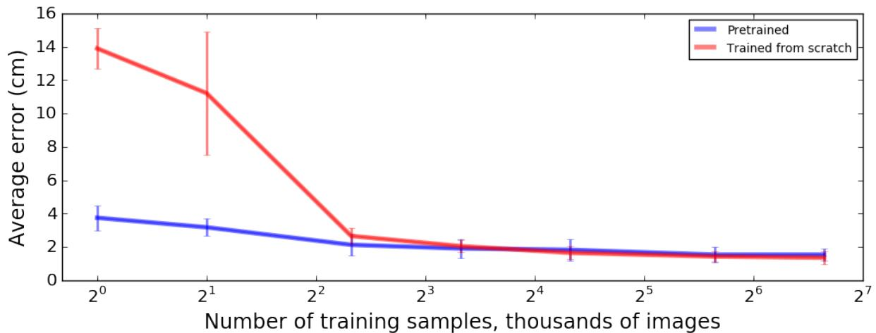
Figure 2.9: Sensitivity of test error on real images to the number of simulated training examples used. Each training example corresponds to a single labeled example of an object on the table with between 0 and 10 distractor objects. Lighting and all textures are randomized between iterations.
