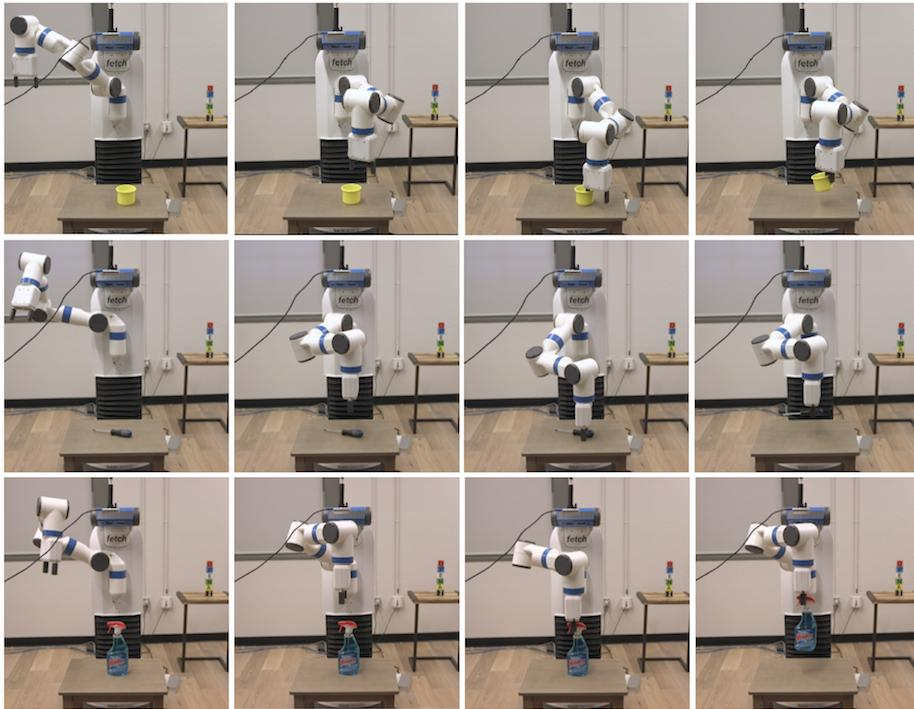
Figure 3.9: Typical grasp executions on the physical robot.
